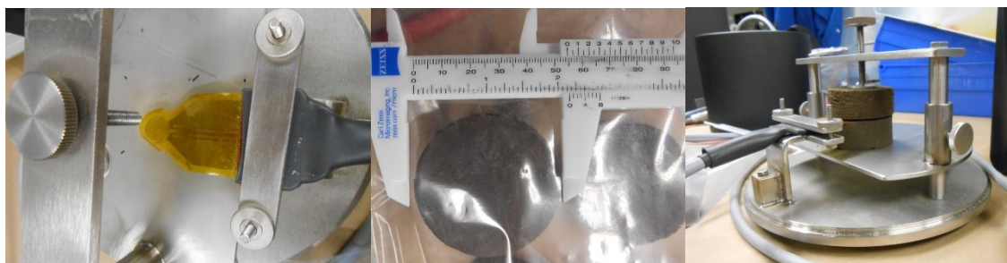
Figure 8-3: Thermal properties measurement a) HOT DISK TPS 500 S. b) prepared sample. c) Sample in the equipment for measurement
