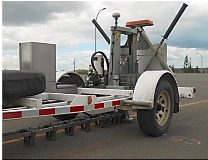
Figure 4-9: Overview of FWD equipment and the location of sensors
