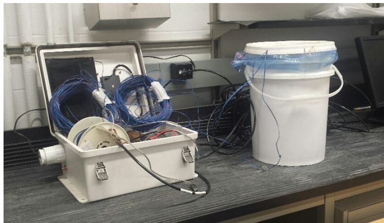
Figure 9-3 The thermocouples at different depths
