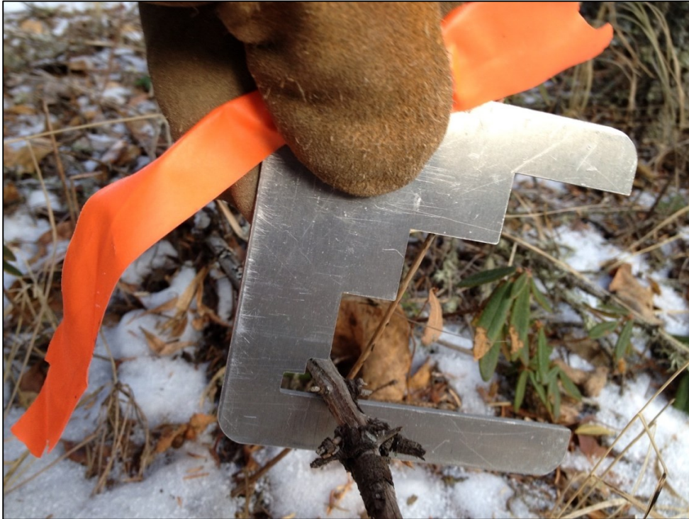
Figure 8. Go-no-go gauge; sample showing size class 2, 0.5 to 1cm.
