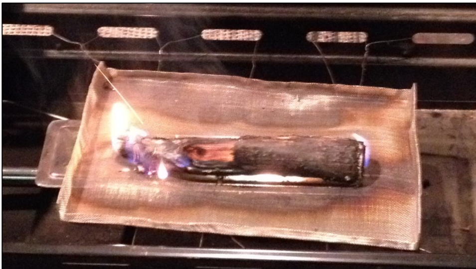
Figure 9. Sample being burned under simulated surface fire conditions in the lab.
