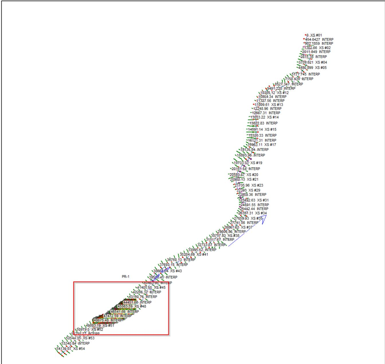
We have a small section of “Terrain” loaded into this model. This is a high-resolution digital elevation model showing the ground elevations. The data was collected using airborne LiDAR and verified with a third-party on-site survey. The terrain data has been “hydro-flattened”, meaning that the area below the normal water surface is flat. The real life model has a terrain file that covers the entire model domain.
