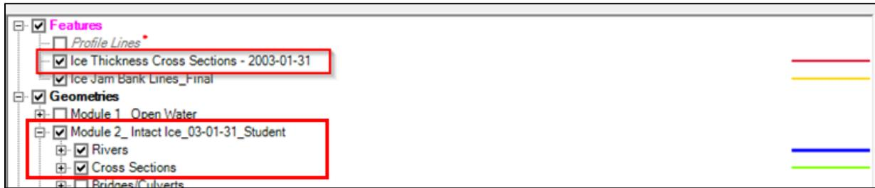
This will allow you to view the locations of several cross-sections where ice thicknesses and water levels were measured on January 31, 2003. These were saved in a shapefile and then added to 'RAS mapper'.
