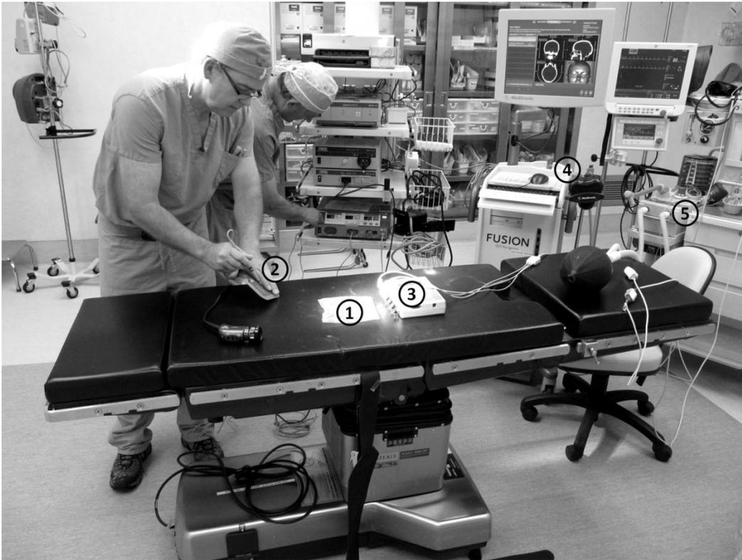
Figure 5-12: OP setup with 1) sensor platform, 2) electrocautery generator, 3) patient simulator, 4) navigation system, 5) anesthesia machine
