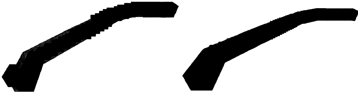
Figure 5-10: Intersection of the block model with the cut-and-fill stope by full blocks (left) and refined blocks (right).
