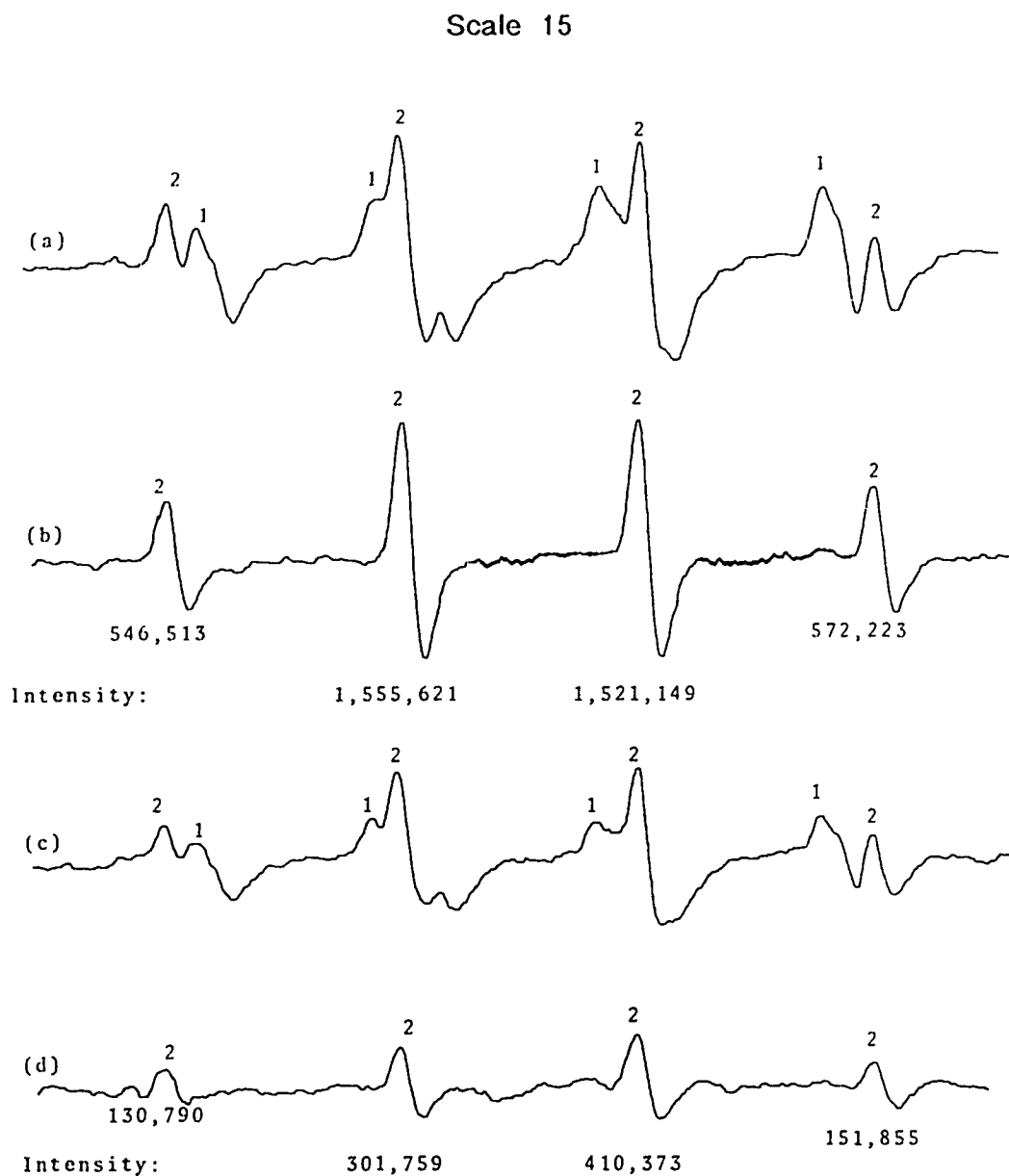
Figure 21: Effect of high concentrations of ferrous ion on the formation of hydroxyl radicals in the presence of SOD. ESR spectra were obtained following the reaction of xanthine with xanthine oxidase in the presence of (a) 40 \mu\text{M Fe}^{2+} ; (b) 40 \mu\text{M Fe}^{2+} and 40 units/ml SOD; (c) 80 \mu\text{M Fe}^{2+} ; (d) 80 \mu\text{M Fe}^{2+} and 40 units/ml SOD.
