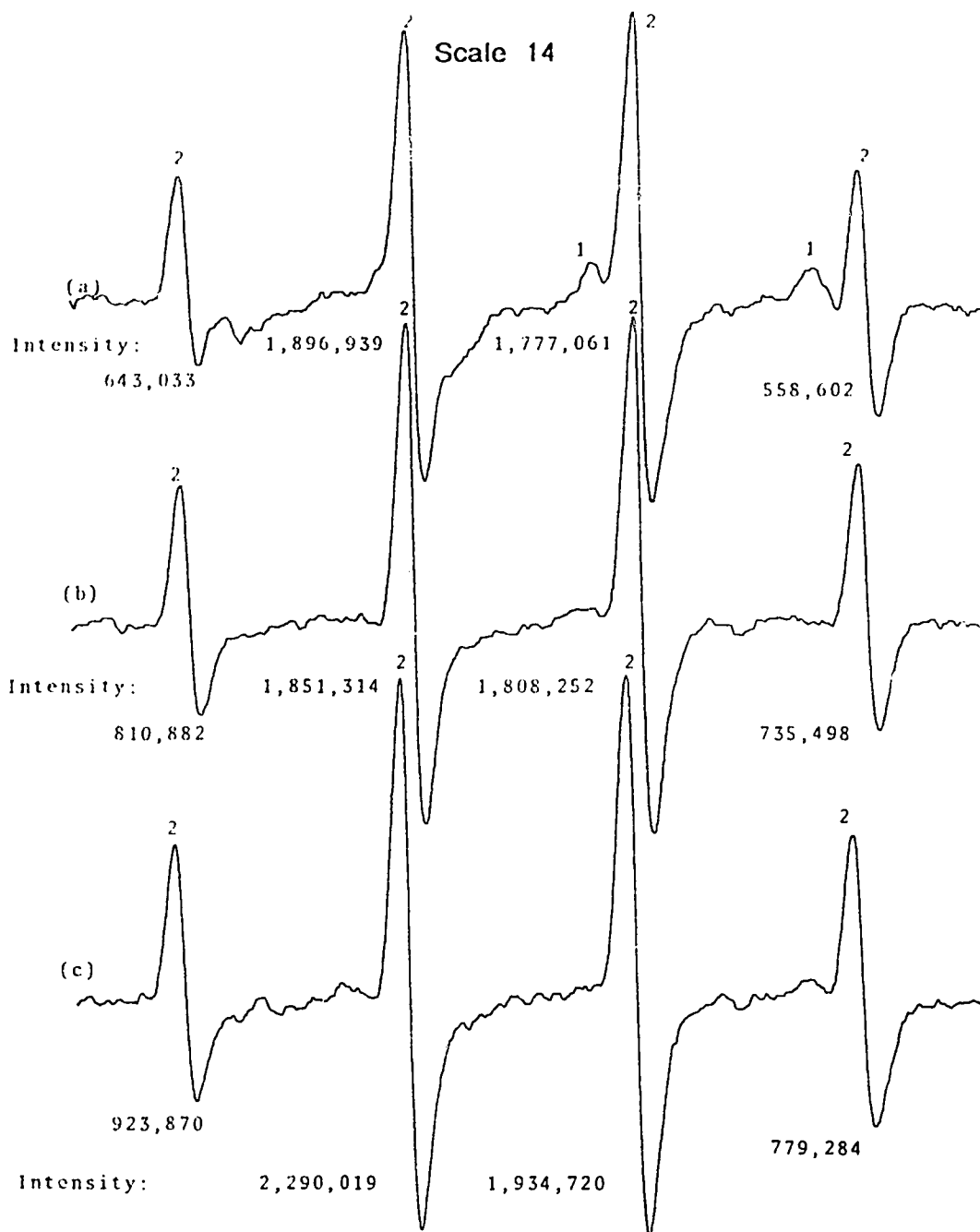
Figure 32: Dose-response characteristics of SOD on enhancing the formation of hydroxyl radical in the presence of ferric ion. ESR spectra were obtained following the reaction of xanthine with xanthine oxidase in the presence of 0.3 mM \text{Fe}^{3+} and (a), 5 units/ml SOD; (b), 10 units/ml SOD; (c), 20 units/ml SOD; (d), 40 units/ml SOD; (e), 80 units/ml SOD; (f), 300 units/ml SOD.
