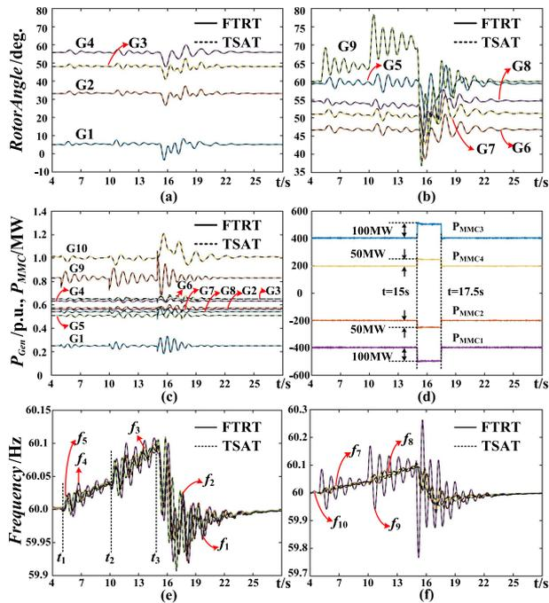
Fig. 9. FTRT co-simulation for preview of AC/DC grid behavior under inter-area oscillation: (a) Generator rotor angles, (b) output power of generators and MMCs, and (c) generator frequencies.
