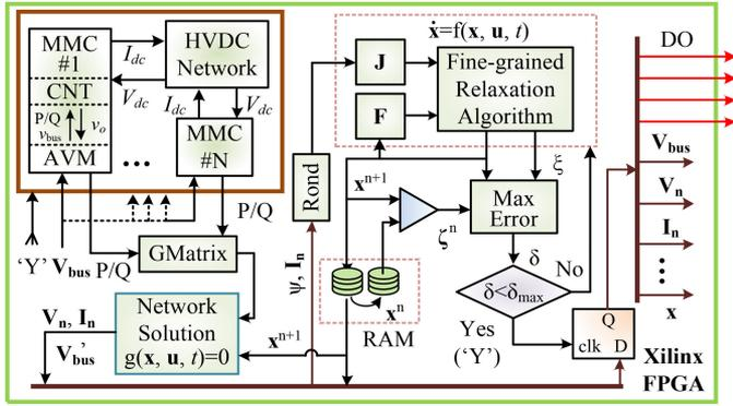
Fig. 4. Integrated AC/DC grid top-level hardware design scheme and signal flow routes.
