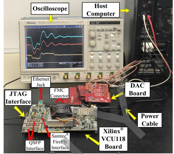
Fig. 3. Hardware setup for FTRT simulation.
