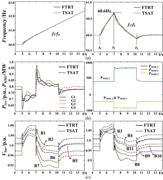
Fig. 7. Predictive control based on FTRT co-simulation for power system stability analysis: (a) AC grid frequency, (b) output power of synchronous generators and MMCs, and (c) AC bus voltages.
