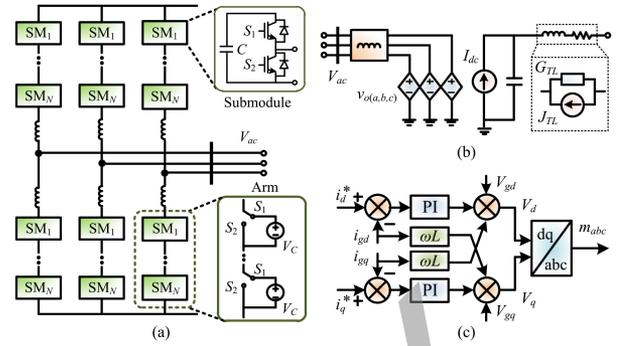
Fig. 2. Three-phase MMC as an HVDC converter: (a) Circuit configuration, (b) average value model, and (c) current controller in  $d$ - $q$  frame.
