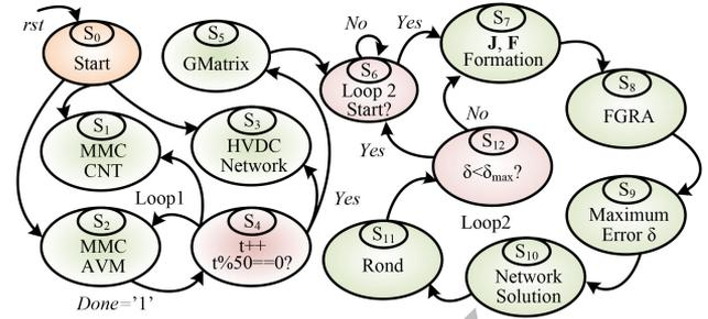
Fig. 5. Top-level finite state machine for the coordination of hardware modules of the integrated AC/DC grid.
