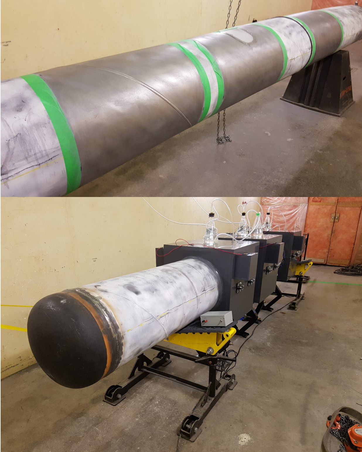
Figure 3.4 (Top) final metal surface preparation of selected areas of the pipe segment and (bottom) pipe segment during live testing.
