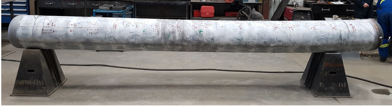
Figure 3.10 Pipe segment after post test NDE.
