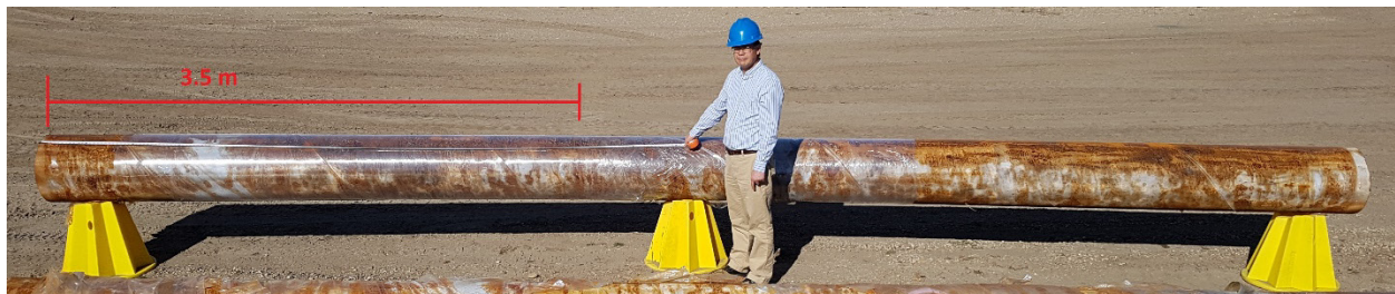
Figure 3.2 Image of the pipe that was designated for testing, taken before it was cut down to the full-scale specimen length showing the external surface condition.
