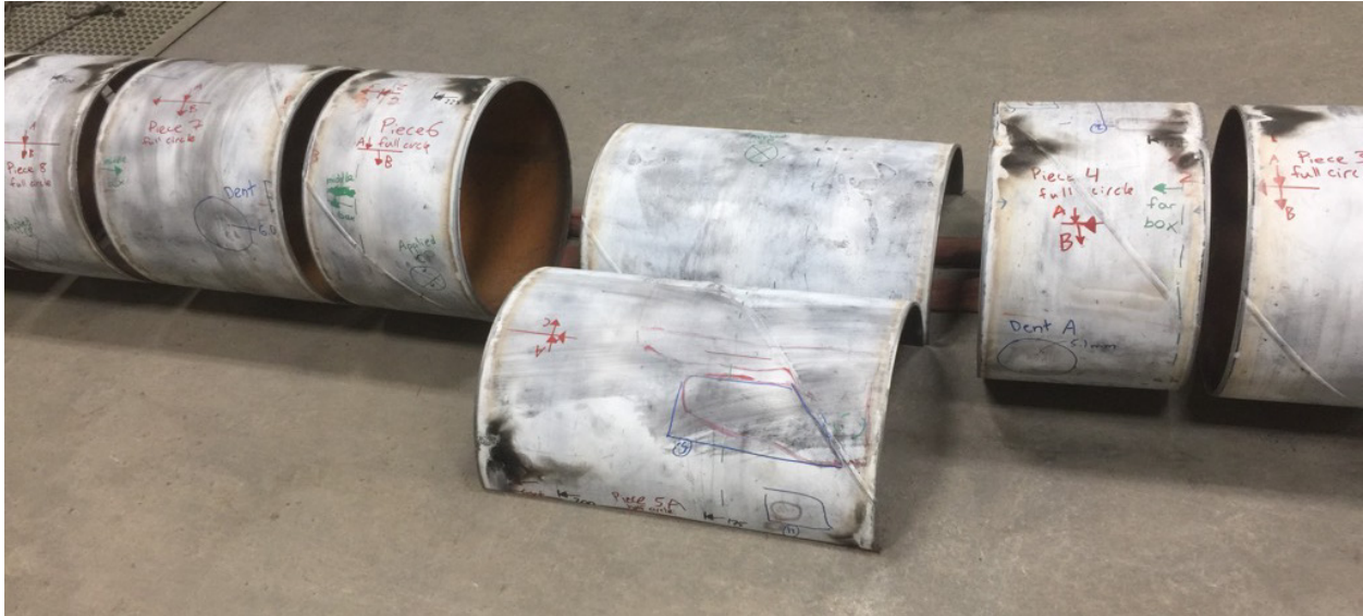
Figure 3.11 Pipe segment cut into small sections after completion of the full-scale test.
