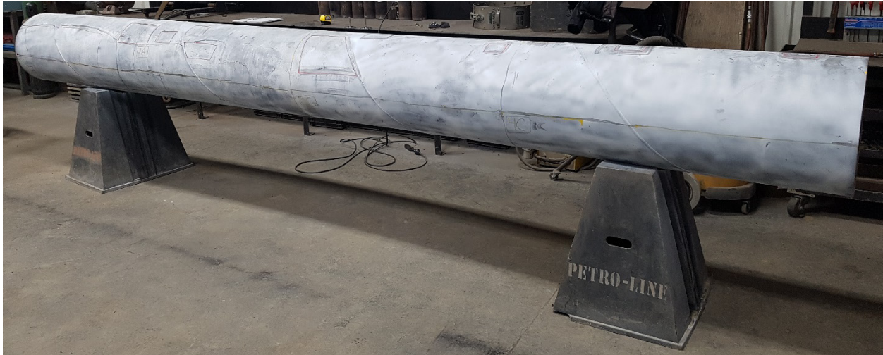
Figure 3.3 4.77 m pipe segment after pre-test MPI, with SCC colony borders drawn in red.
