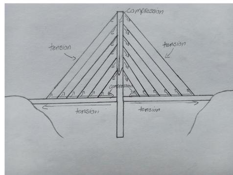
Figure 1: Sketch illustrating the forces being applied to the bridge
