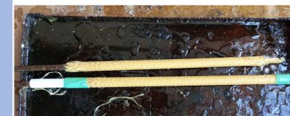
Figure 7: Dry preforms being cured
