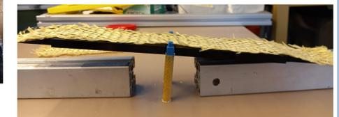
Figure 8: Assembly of the braided composite walking bridge
