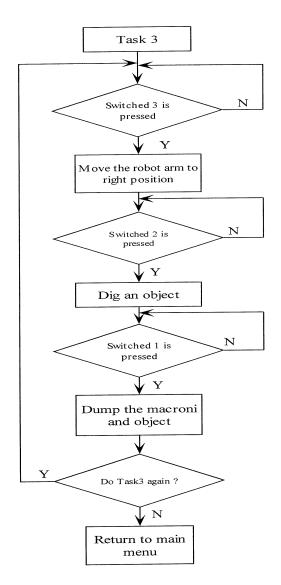
Fig. 8. Software control for switch controlled playback of movements by individual user interface switch.
