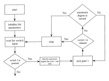
Fig. 6. Software control of individual joints by individual user interface switch pairs.
