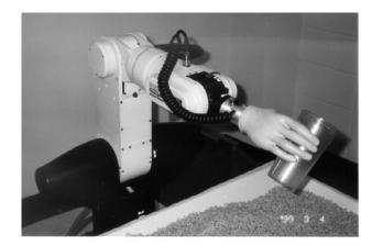
Fig. 4. The robot hand with glove.
