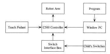
Fig. 2. Block diagram of the robot arm system.
