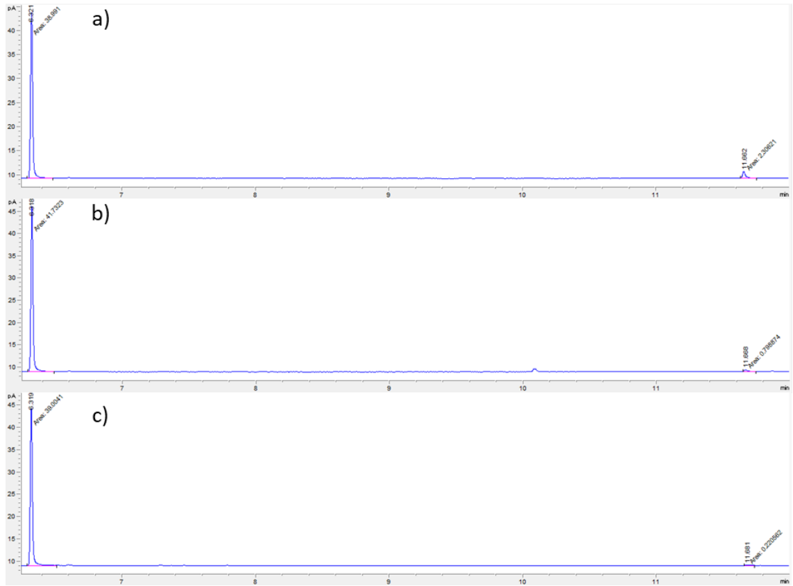
Figure A.7 Chromatographic signal for fluoranthene after exposure to a) cotton, b) polyamide, and c) polyester, and extraction in saltwater solutions
