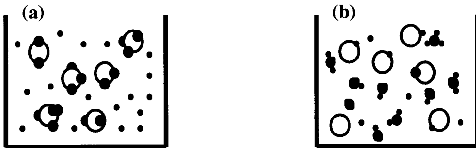
Figure 1.3: Schematic of a bitumen extraction system without slime coating (a), and with slime coating (b). Air bubbles are illustrated as hollow white circles, bitumen drops as solid black circles, and fine particles as the small solid grey circles.
