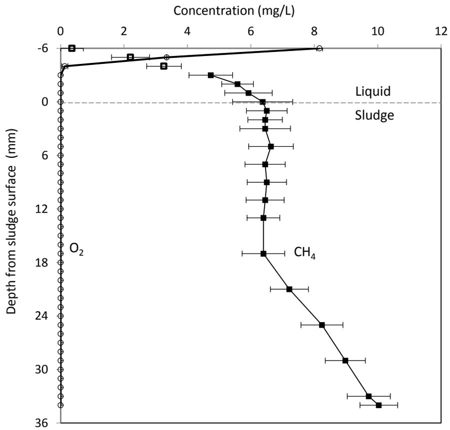
Figure 14 Oxygen and methane concentration profiles
