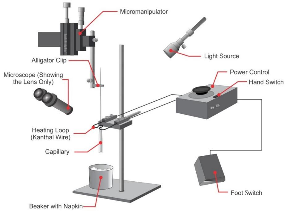
Figure 6 Schematic diagram for tapering of gas and media capillary
