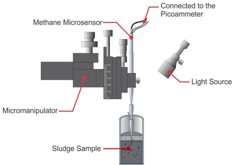
Figure 13 Experimental up for sample testing
