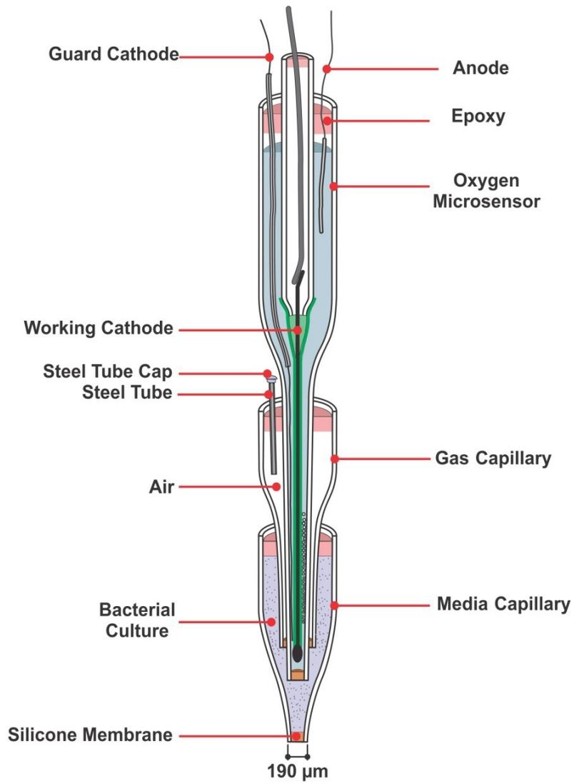
Figure 2 Schematic diagram of the methane microbiosensor
