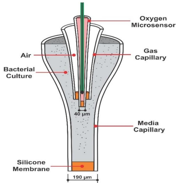
Figure 4 Schematic diagram of the tip of the methane microbiosensor
