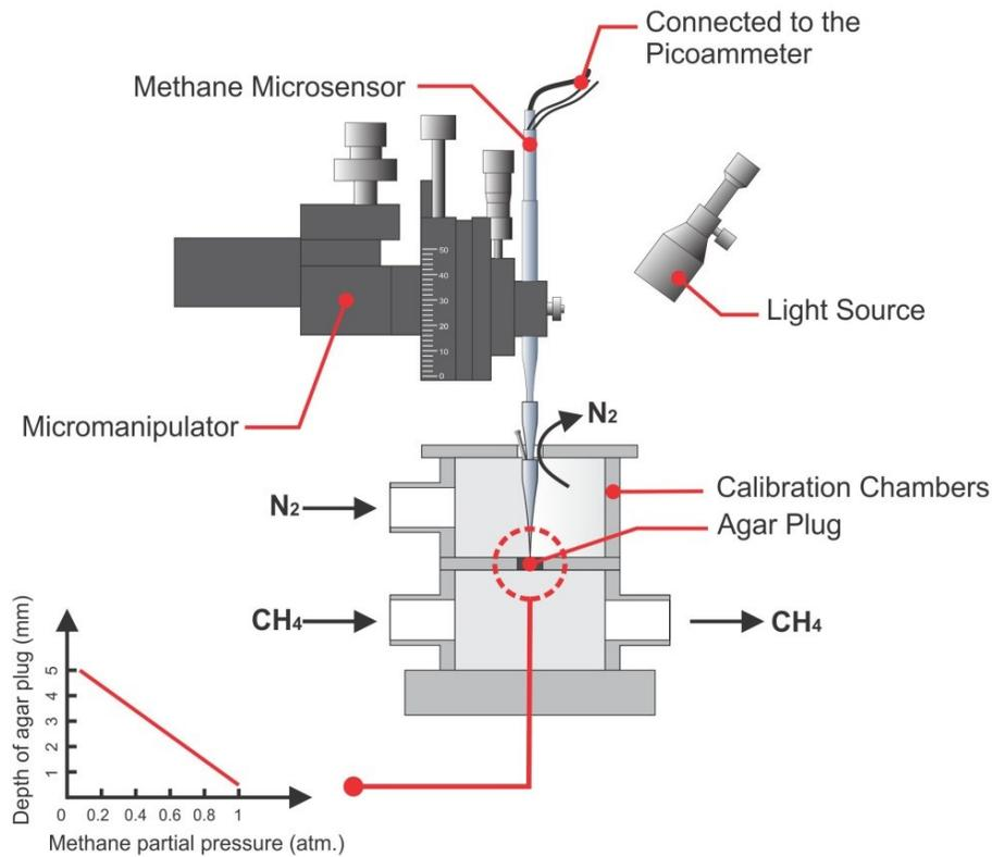
Figure 8 Experimental setup for calibration
