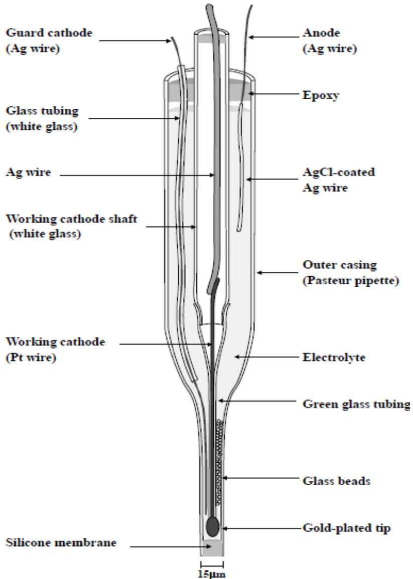
Figure 1 Schematic diagram of the oxygen microsensor (Lu & Yu, 2002).
