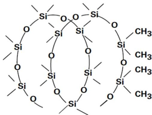
Figure 3 The basic structure of silicone rubber (Characteristic properties of Silicone Rubber Compounds, 2012)
