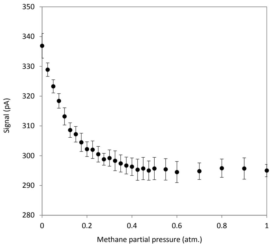
Figure 10 Calibration curve for methane microbiosensor 1 on day 6
