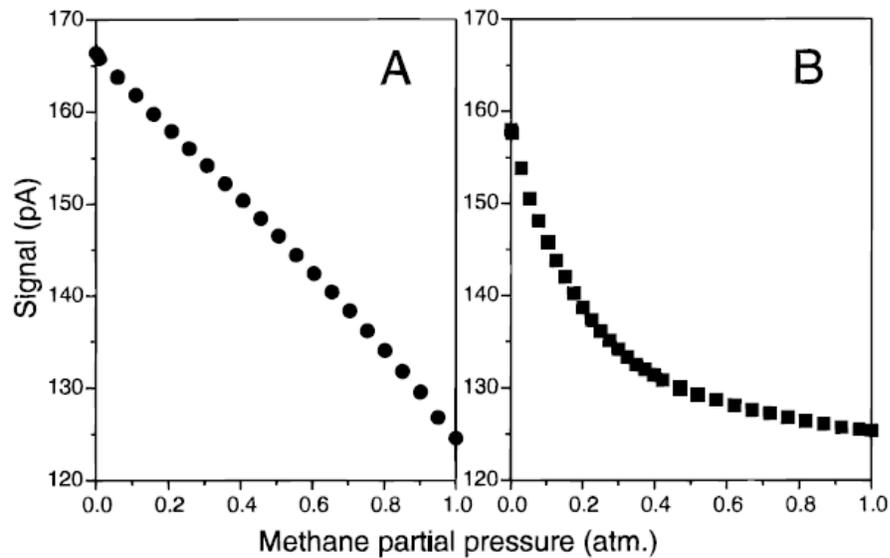
Figure 12 Calibration curves for two methane microbiosensors
