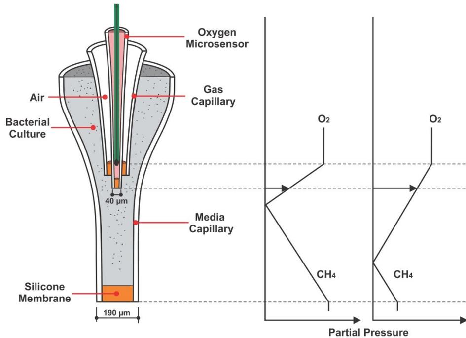
Figure 7 Schematic model of the gradients of oxygen and methane
