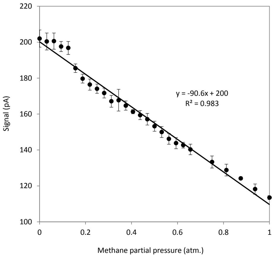
Figure 9 Calibration curve for methane microbiosensor 1 on day 2
