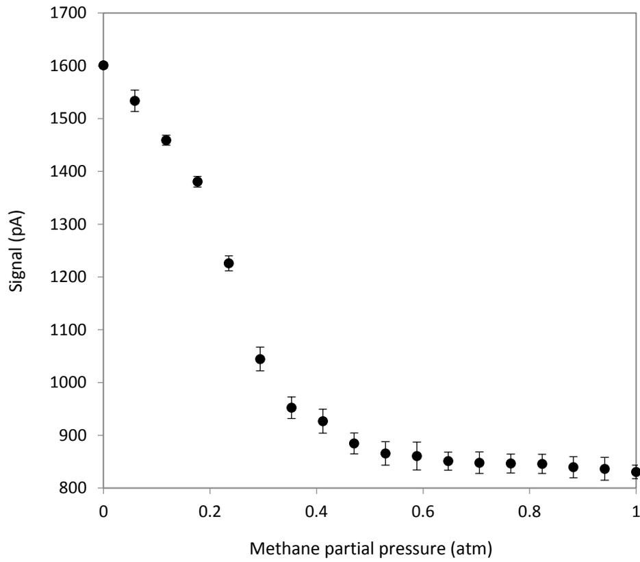
Figure 11 Calibration curve for methane microbiosensor 2 on day 5
