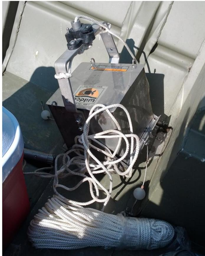
**Figure 3-5 – Eckman Dredge sediment sampler used in field study for stormwater retention pond sediment sampling**
