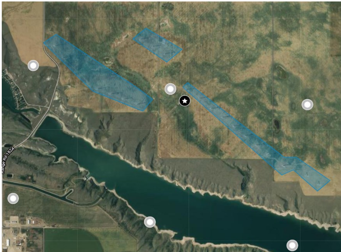
Figure 3-1. Location of wind atlas data with respect to wind farm layout at Chin Chute using Google Maps.
