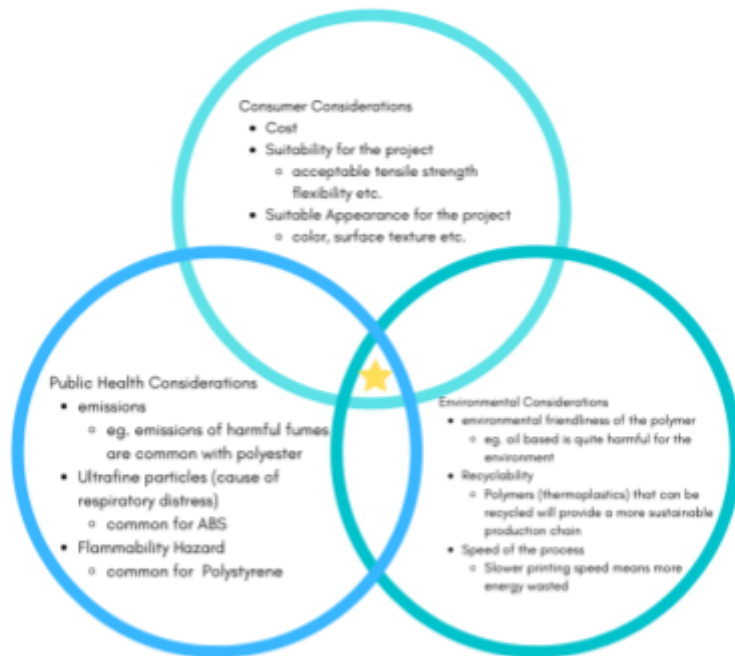
Figure 2 - Venn Diagram of different implications. (The yellow star in the center indicates the best polymer possible that has taken into consideration all three impacts.)
