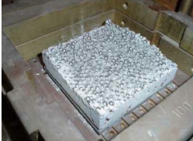
Figure B.6 Failure surface of the lower half of the synthetic conglomerate after direct shear testing (Akram 2010)
