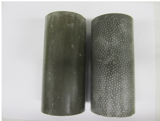
Figure 4.2 The cement paste and artificial conglomerate samples
