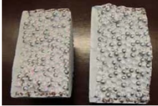
Figure B.5 The failure surface of the synthetic conglomerate after Brazilian tensile testing (Akram 2010)
