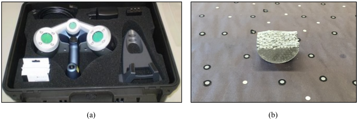
Figure 5.1 (a) 3D laser scanner (MAXscan); (b) Artificial reflective targets in the background.
