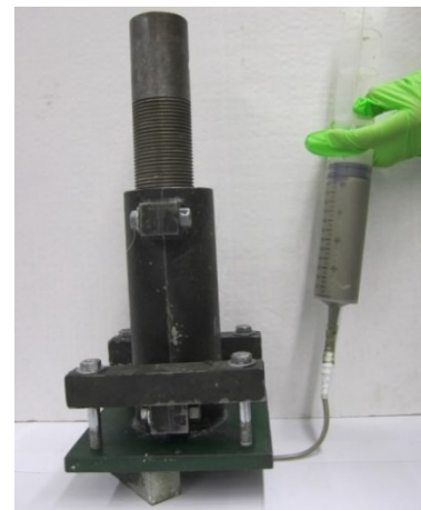
(i) Injecting cement
