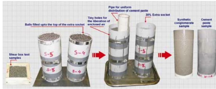
Figure B.1 Sample preparation steps (Akram 2010)
