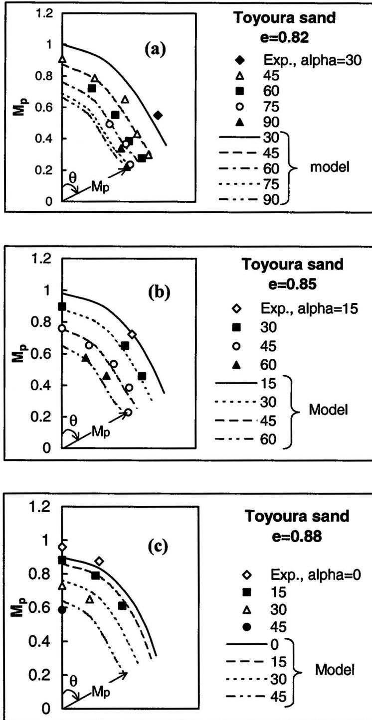
Figure 14 Comparison of modeled and measured variations of  $M_p$  with  $b$  and  $\alpha_\sigma$
