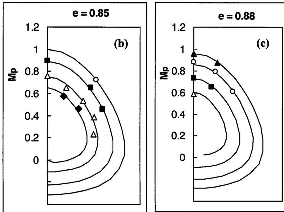
**Figure 9** Variation of  $M_p$  in Reference Octahedral Plane (ROP) for Toyoura sand
