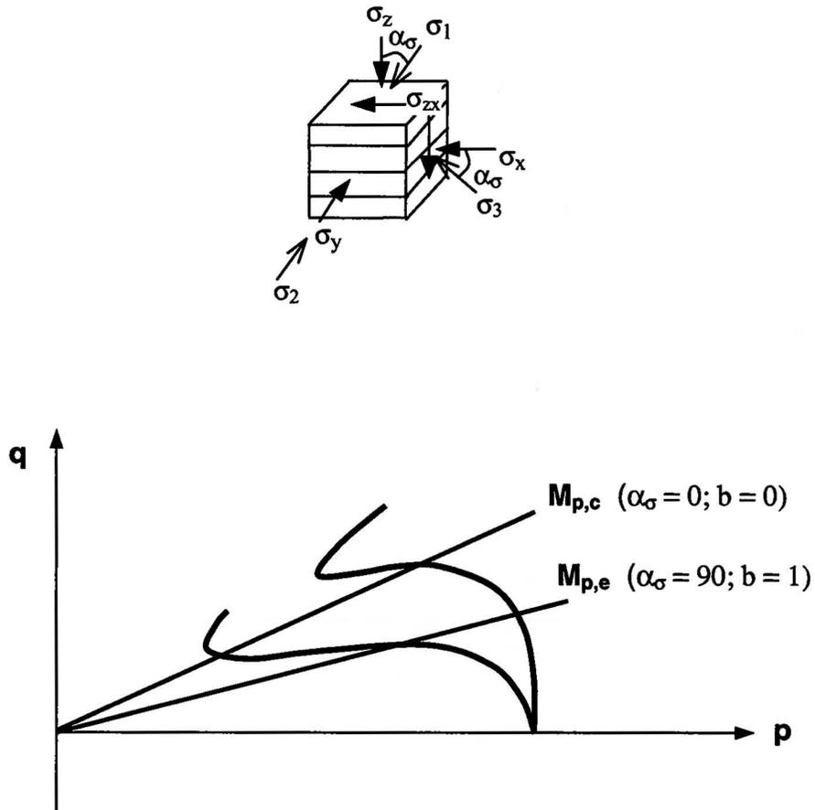
**Figure 1** Schematic representation of undrained effective stress paths and stress conditions of loose sand in triaxial compression and extension loading
