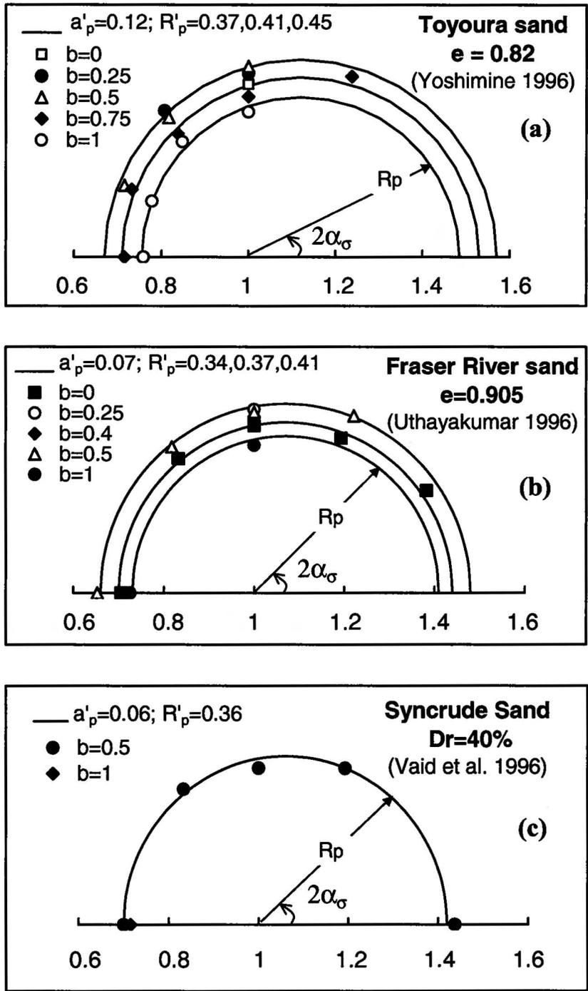
**Figure 11** Variations of  $R_p = \sin \phi_p$  with  $\alpha_\sigma$  for different sands as represented in Reference Mohr Diagram
