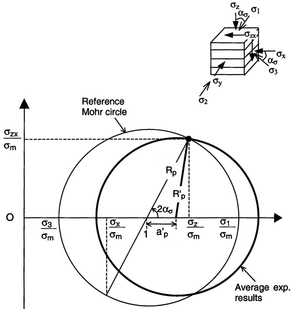
**Figure 10** Representation of stress states at P-UESP with the direction of loading  $\alpha_\sigma$  using the reference Mohr Circle (RMC).
