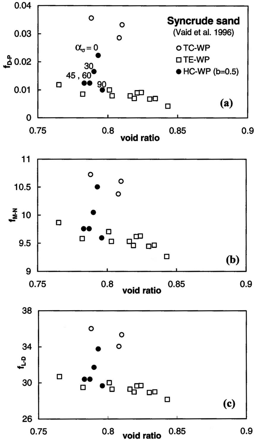
**Figure 6** Correlating stress states at P-UESP with void ratio in Syncrude sand, using different yield-failure criteria
