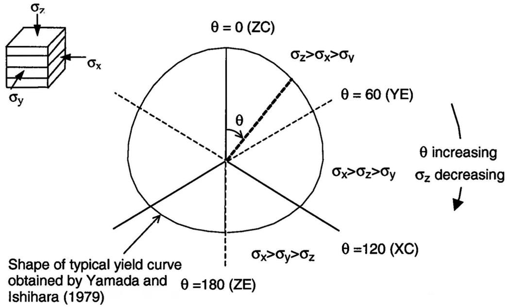
**Figure 12** Changes in relative magnitudes of principal stresses with  $\theta$  in true triaxial test (TTT).
