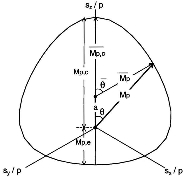
**Figure 13** Definition of parameters used in modeling the variation of  $M_p$  with  $b$  and  $\alpha_\sigma$
