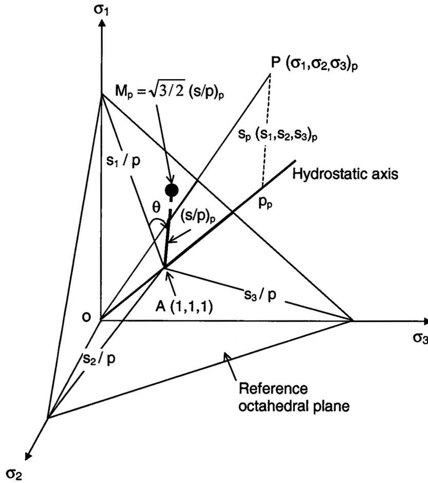
**Figure 8** Representation of stress states at the P-UESP in the “Reference Octahedral Plane” (ROP) defined in principal stress space
