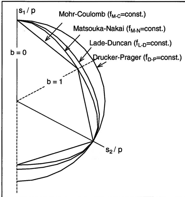
**Figure 5** Representation of different yield-failure criteria in octahedral plane
