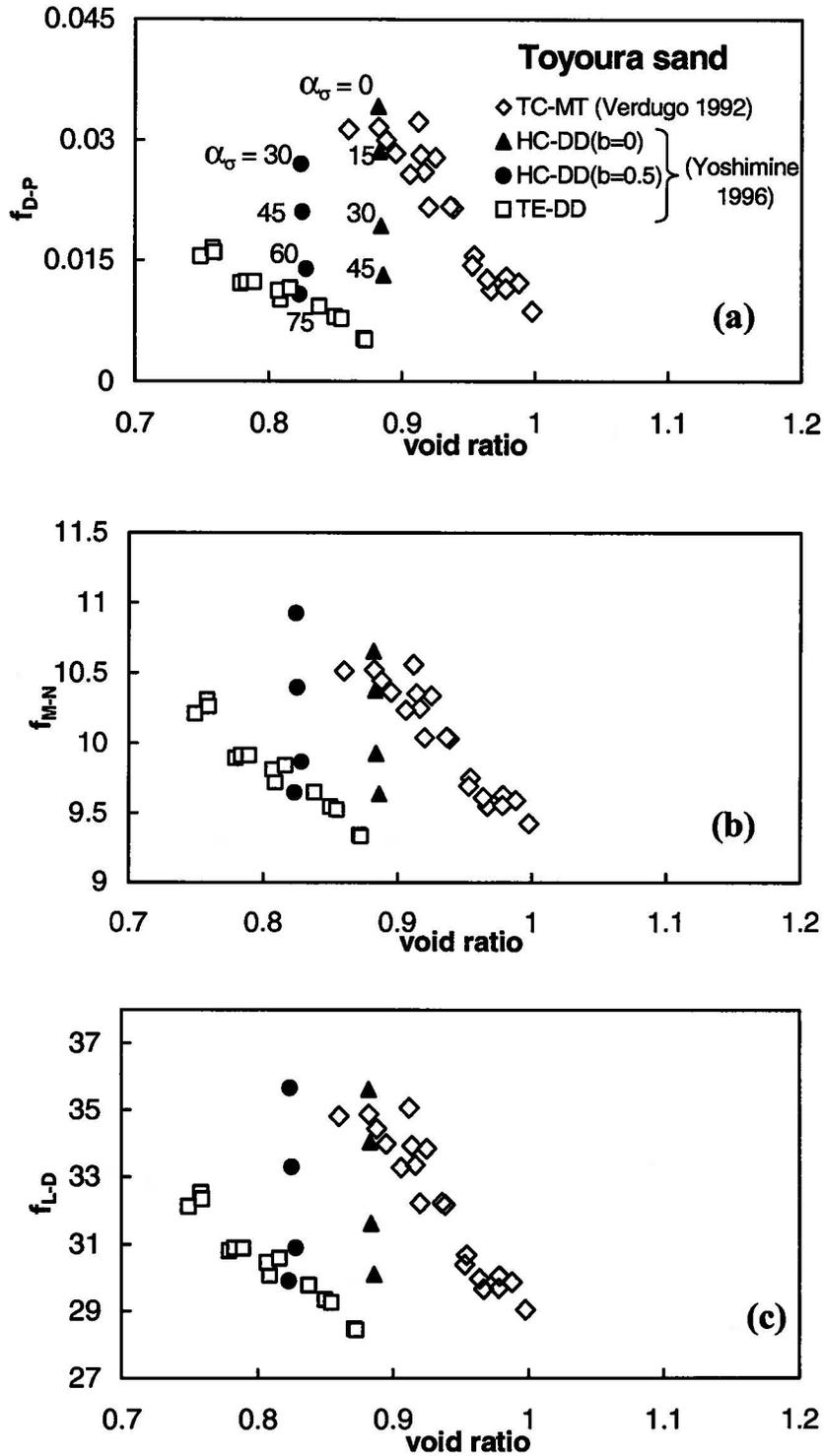
**Figure 7** Correlating stress states at P-UESP with void ratio in Toyoura sand, using different yield-failure criteria
