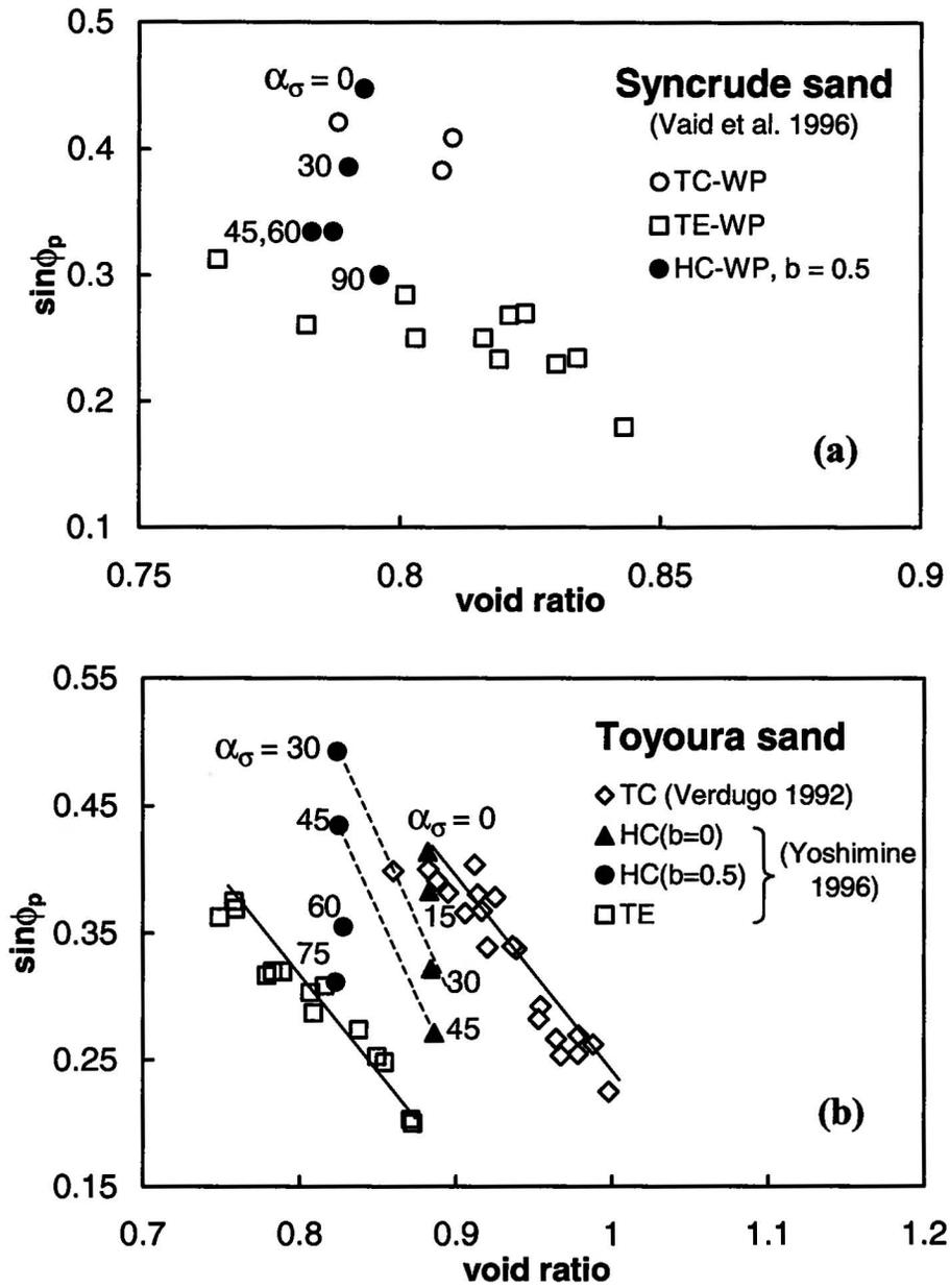
**Figure 4** Effects of direction of loading ( $\alpha_\sigma$ ) and intermediate principal stress on  $\sin\phi_p$  in Syncrude sand and Toyoura sand
