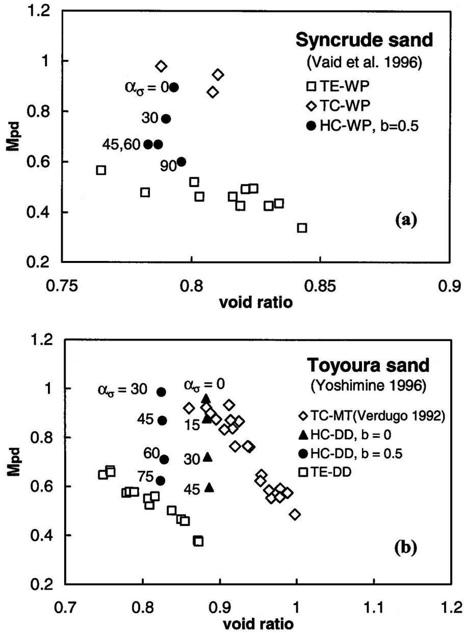
**Figure 3** Effect of direction of loading  $\alpha_\sigma$  on  $M_{1p}$  in Syncrude sand and Toyoura sand
