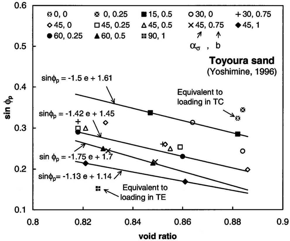
**Figure 2** Variation of  $\sin \phi_p$  with void ratio for different combinations of  $b$  and  $\alpha_\sigma$  as obtained from Hollow Cylinder tests
