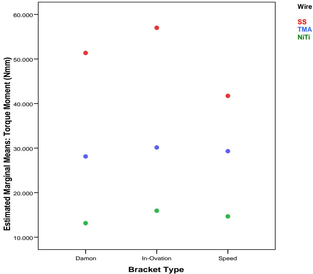
**Figure 4.17 Profile Plot at 48° of Wire Torsion**
