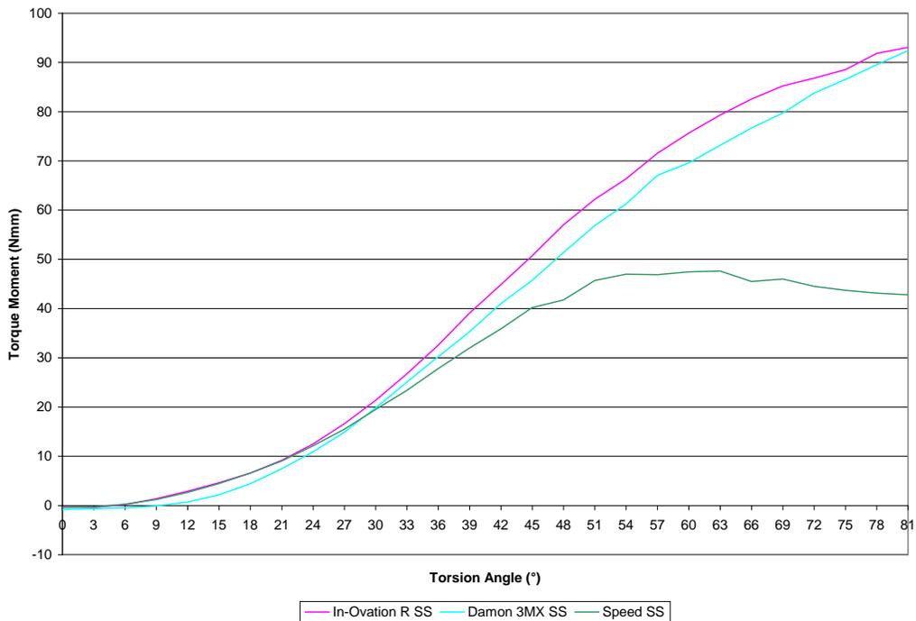
**Figure 4.7 Average Torque Expression for Stainless Steel Wire**
