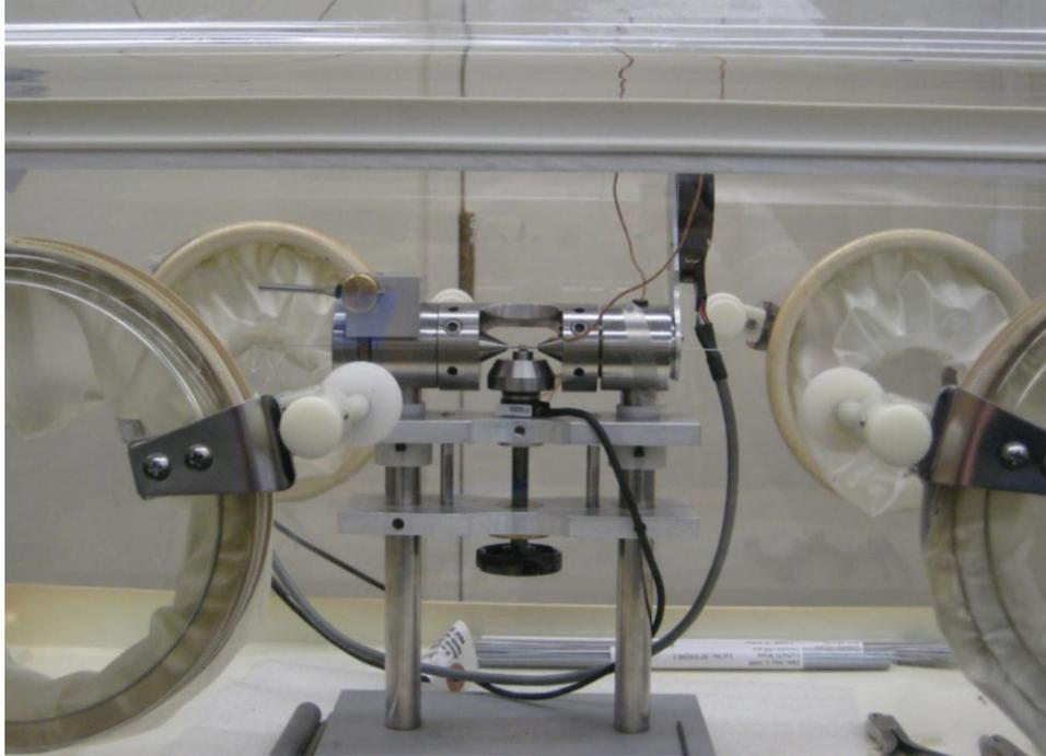
**Figure 4.3 Orthodontic Torque Measurement Device Within Incubator**
