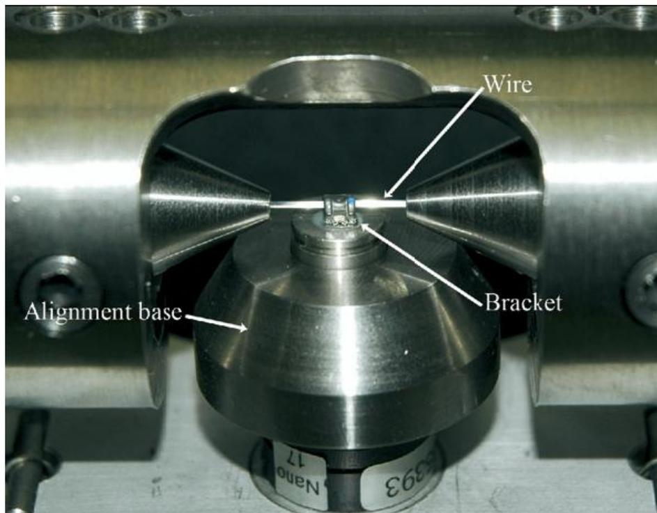
**Figure 4.2 Bracket and Wire Alignment in the Orthodontic Torque Measurement Device**
