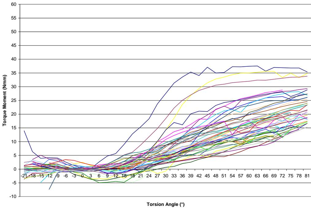
Figure K. Torque Expression for Damon 3MX Brackets with CuNiTi Wires
