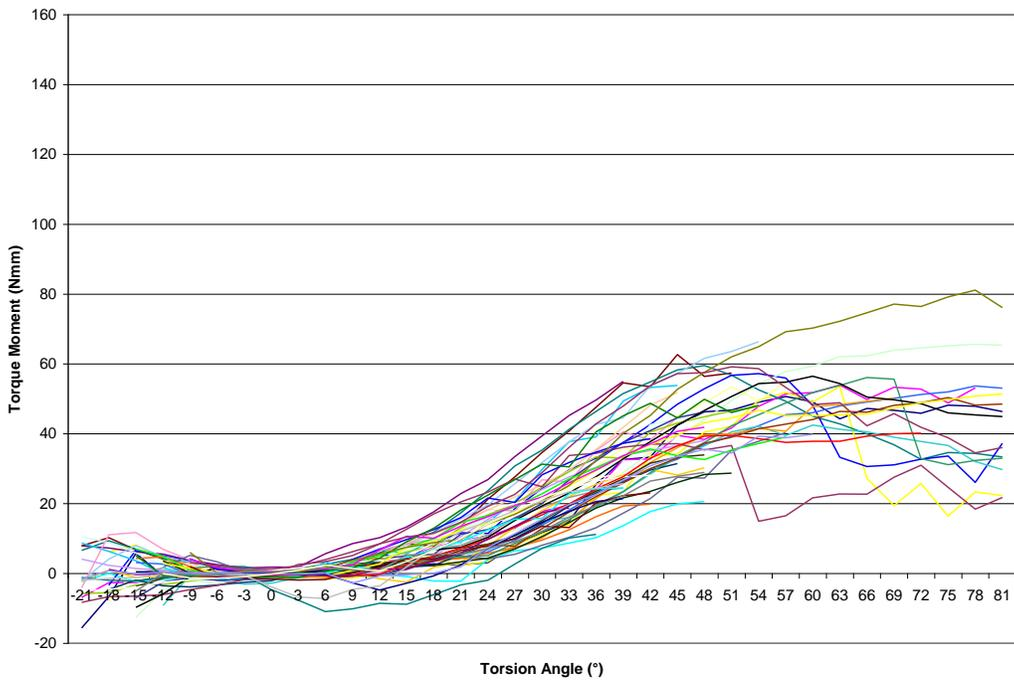
**Figure G. Torque Expression for Speed Brackets with Stainless Steel Wires**
