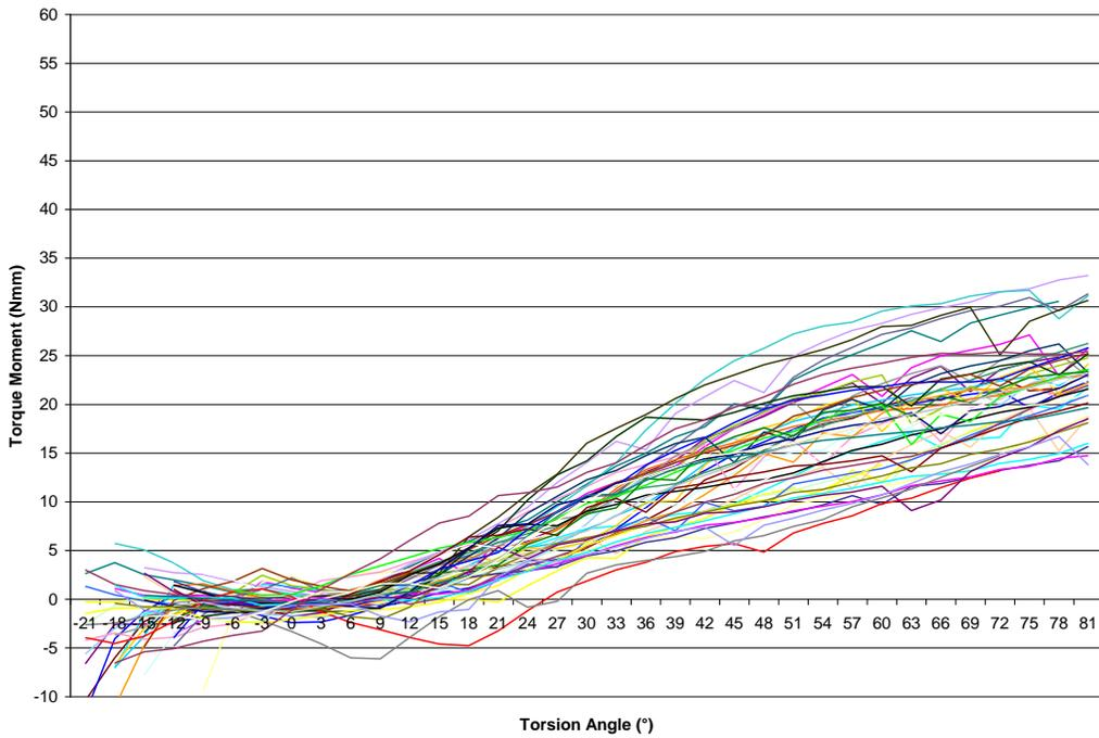
Figure M. Torque Expression for Speed Brackets with CuNiTi Wires
