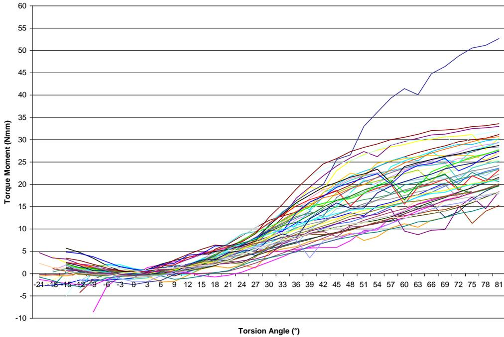
Figure L. Torque Expression for In-Ovation R Brackets with CuNiTi Wires
