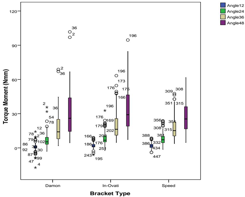
Figure 4.4 Median Torque Expression According to Torsional Angle
