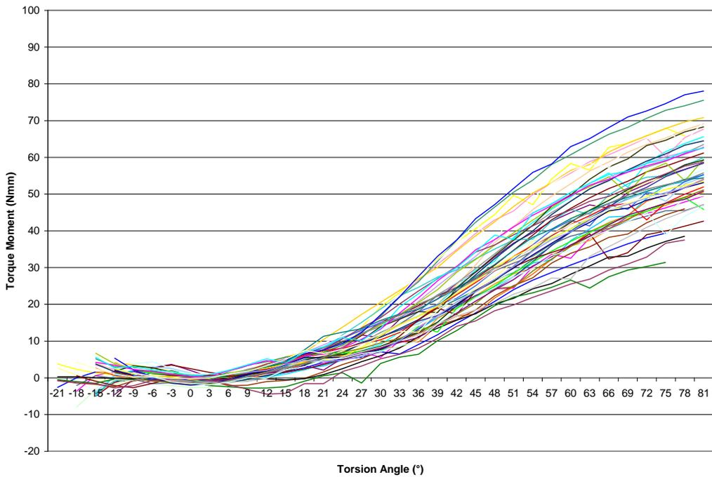
**Figure I. Torque Expression for In-Ovation R Brackets with TMA Wires**
