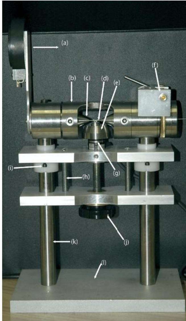
**Figure 4.1 Orthodontic Torque Measurement Device**
