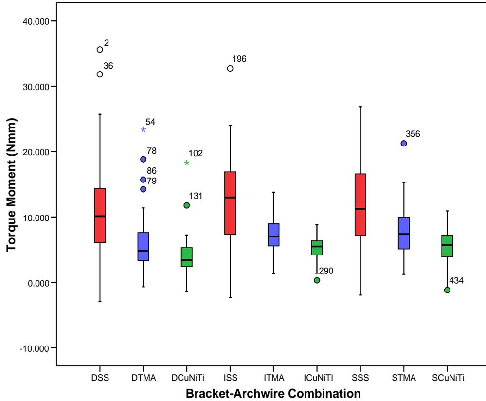
**Figure 4.5 Median Torque Expression for All Bracket-Wire Combinations at 24° of Wire Torsion**
