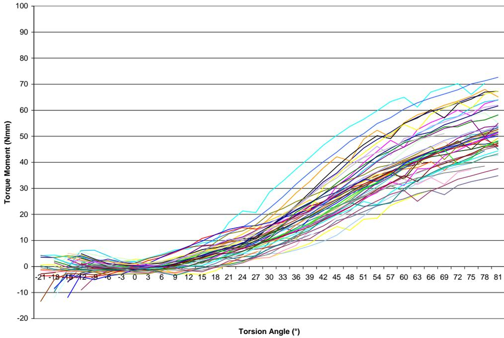
Figure J. Torque Expression for Speed Brackets with TMA Wires
