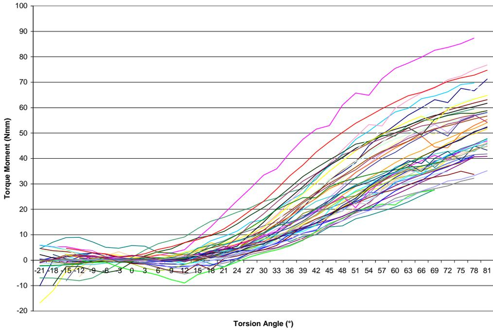
**Figure H. Torque Expression for Damon 3MX Brackets with TMA Wires**
