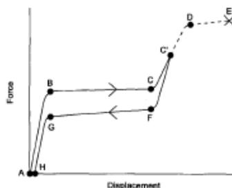
**Figure 2.1 Displacement vs. Force Plot Demonstrating Pseudoelasticity<sup>3</sup>**
