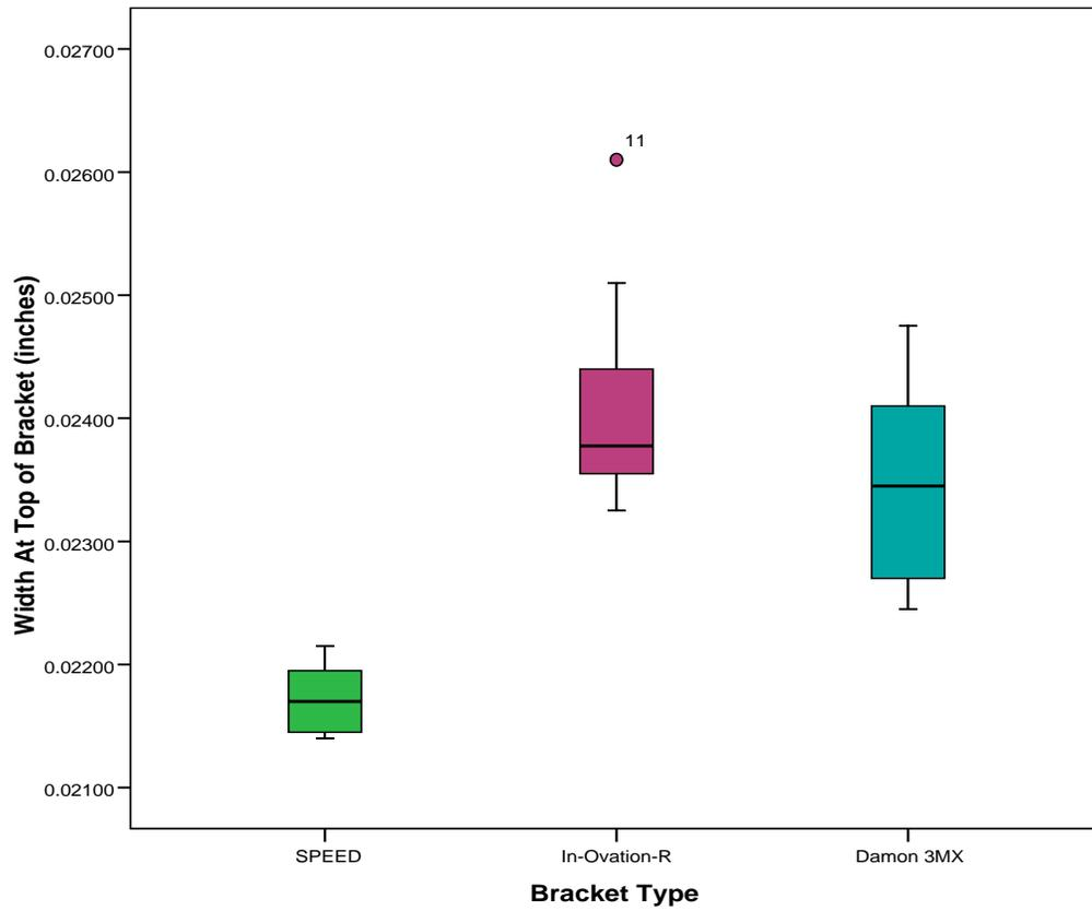
Figure 4.11 Median Bracket Top Width
