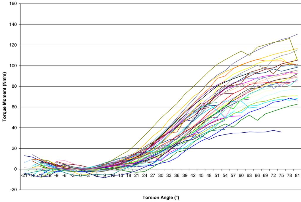
**Figure F. Torque Expression for In-Ovation R Brackets with Stainless Steel Wires**
