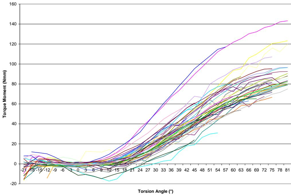
Figure E. Torque Expression for Damon 3MX Brackets with Stainless Steel Wires
