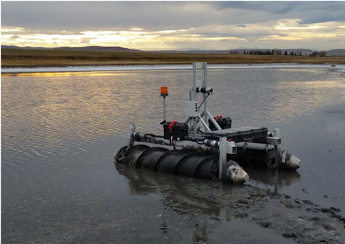
Figure 5.7: Prototype amphibious rover during slough testing. (Courtesy of Copperstone Technologies Ltd.)
