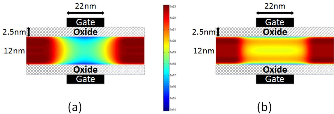
Figure 4.3: Charge distribution in a 22-nm FinFET (a) without and (b) with an appreciable gate voltage. When an appreciable gate voltage is present, the charge density exhibits two peaks, located above and below the center of the channel.
