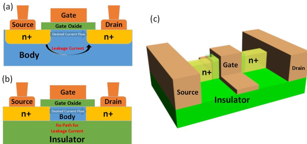
Figure 1.1: (a) A traditional planar MOSFET, (b) UTB-SOI transistor, and (c) FinFET transistor.
