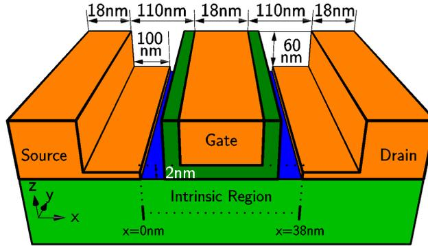
Figure 2.1: Device simulated in this study. The gate length is 18 nm and 2 nm of  $\text{Al}_2\text{O}_3$  is used as the gate oxide. A cross-section of the intrinsic region is indicated by the dotted lines. The source and drain geometries are symmetric with respect to the gate. The positions  $x = 0$  and  $x = 38$  nm, which delimit the intrinsic portion of the device, are labeled for later reference.
