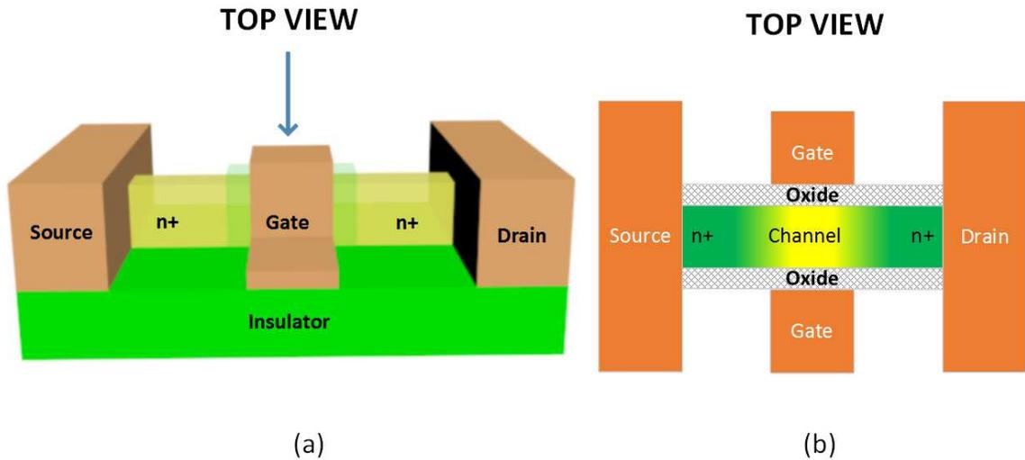
Figure 4.1: The FinFET viewed (a) in three dimensions and (b) from a top view. The simulation domain for the intrinsic device is most easily seen in part (b); it is defined by the oxide, channel, and  $n^+$  regions bounded by the orange contact regions.
