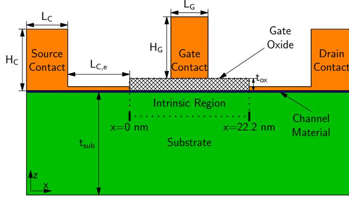
Figure 1.6: Common device structure used in Chapter 3. The dimensions are given in Tables 3.1 and 3.2. The dotted lines show a cross-section of the intrinsic portion of the device, defined as the core of the structure excluding parasitics.
