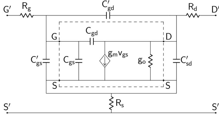
Figure 3.2: Equivalent circuit used in this study, with the intrinsic portion boxed. The labels  $S$ ,  $D$ , and  $G$  refer to the source, drain, and gate terminals, respectively, of the intrinsic device, while their primed counterparts  $S'$ ,  $D'$ , and  $G'$  refer to the corresponding extrinsic device terminals.
