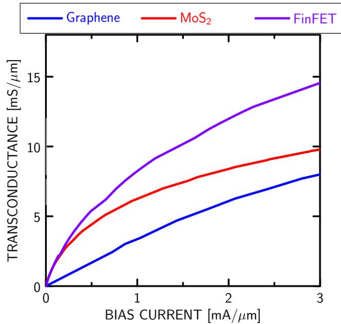
Figure 4.7: Transconductance  $g_m$  vs. drain bias current  $I_D$  for graphene, SL MoS<sub>2</sub>, and FinFET transistors. The drain and gate voltages were adjusted to provide the largest possible value of  $g_m$  at each value of  $I_D$ .
