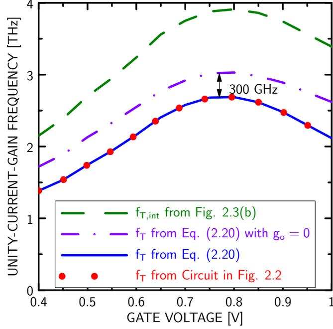
Figure 2.10: Extrinsic unity-current-gain frequency  $f_T$  vs. gate voltage  $v_G$  as found from (2.20). Values of  $f_T$  extracted from the circuit of Fig. 2.2 are also shown to validate (2.20), and values of the *intrinsic*  $f_{T,int}$  reproduced from Fig. 2.3(b) are shown for reference.
