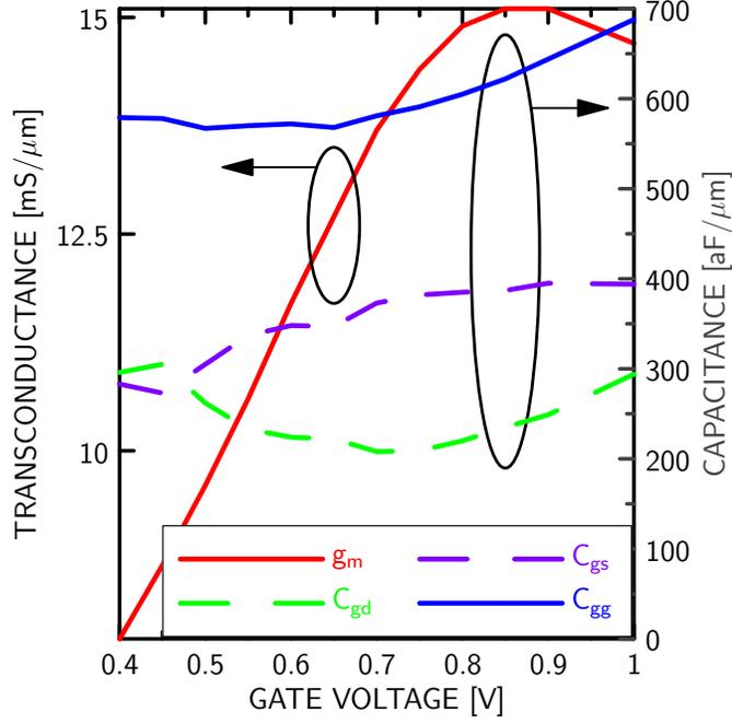
Figure 2.4: Transconductance  $g_m$  and gate capacitance  $C_{gg}$  vs. gate voltage  $v_G$  for the GFET. The components  $C_{gs}$  and  $C_{gd}$  of  $C_{gg}$  are also shown, where  $C_{gg} = C_{gs} + C_{gd}$ . The drain voltage  $v_D$  is held fixed at  $V_{DD}/2 = 0.5$  V.
