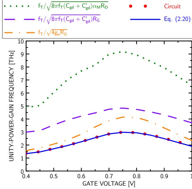
Figure 2.11: Plot of the components of the unity-power-gain frequency  $f_{\max}$  according to the expression (2.21) vs. gate voltage  $v_G$ . Values of  $f_{\max}$  obtained from the circuit of Fig. 2.2 are also shown to validate (2.21).
