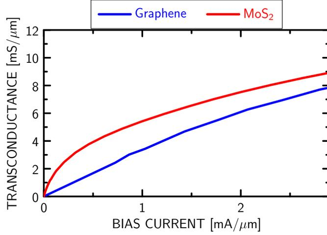
Figure 3.9: Transconductance  $g_m$  vs. bias current  $I_D$  for graphene and SL MoS<sub>2</sub> transistors. The drain and gate voltages were adjusted to provide the largest possible value of  $g_m$  at each value of  $I_D$ .
