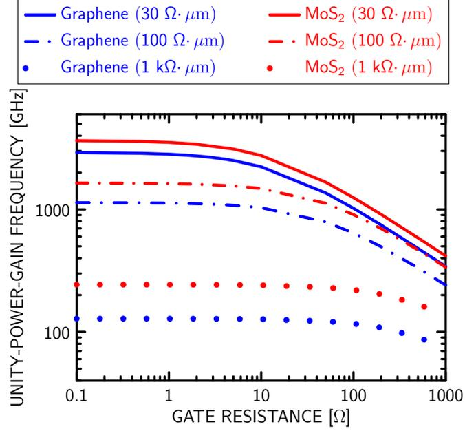
Figure 3.6: Peak (absolute maximum over all bias voltages) unity-power-gain frequency  $f_{\max}(R_g)$  vs. gate resistance  $R_g$  for graphene and MoS<sub>2</sub>. Separate curves are shown for values of contact resistance  $\rho_C$  equal to  $30 \Omega \cdot \mu\text{m}$ ,  $100 \Omega \cdot \mu\text{m}$ , and  $1 \text{ k}\Omega \cdot \mu\text{m}$ .
