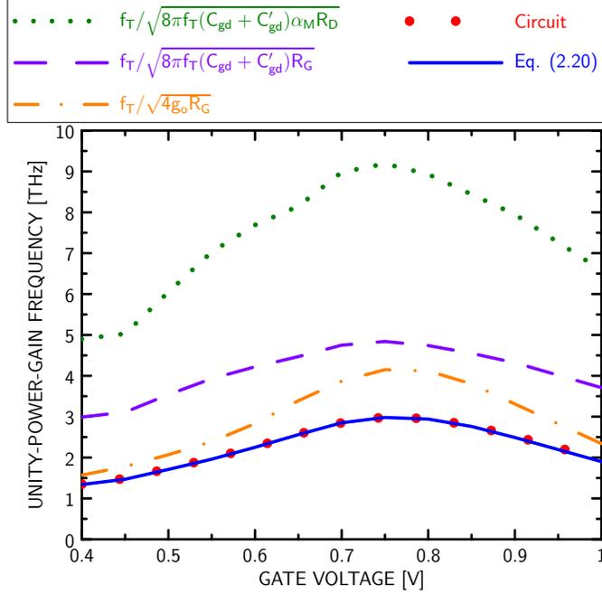
Figure 1.5: Plot of the components of the unity-power-gain frequency  $f_{\max}$  according to the expression (2.21) vs. gate voltage  $v_G$ . Values of  $f_{\max}$  obtained from the circuit of Fig. 2.2 in Chapter 2 are also shown to validate (2.21).
