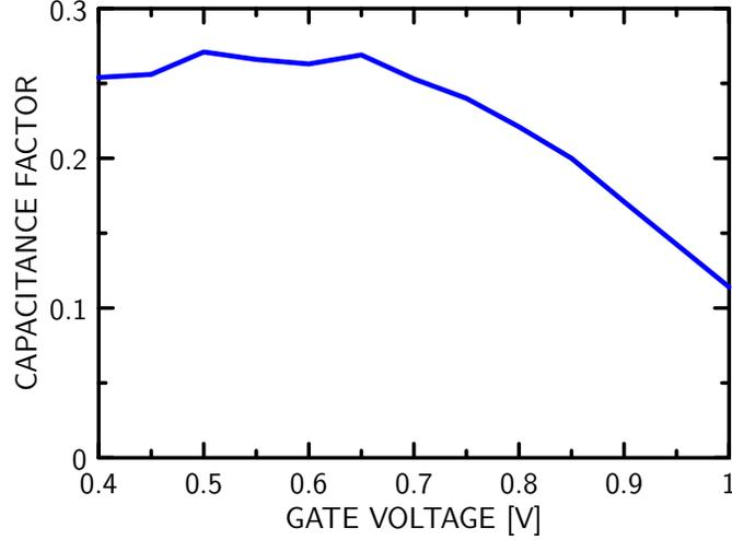
Figure 2.7: Capacitance factor  $(1 - C_{\text{gg}}/C_{\text{ox}})$  vs. gate voltage  $v_G$  for the GFET. The factor appears in the expression (2.1) for  $g_m$ .
