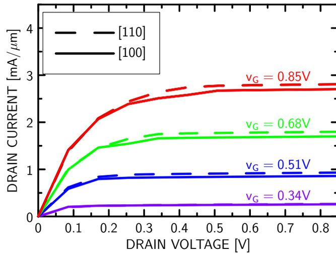
Figure 4.5: Current-voltage characteristics for a 22-nm FinFET along the [110] and [100] crystal directions.
