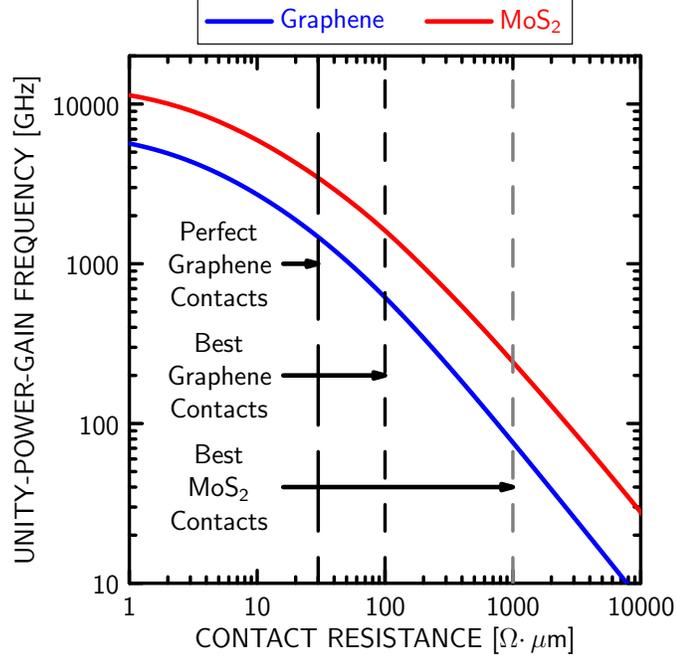
Figure 3.10: Unity-power-gain frequency  $f_{\max}(\rho_C)$  vs. the contact resistance  $\rho_C$  determining the source and drain contact resistances  $R_s$  and  $R_d$ , with  $R_g$  held at  $1 \Omega$ , and with the bias current constrained to  $1.65 \text{ mA}/\mu\text{m}$ .
