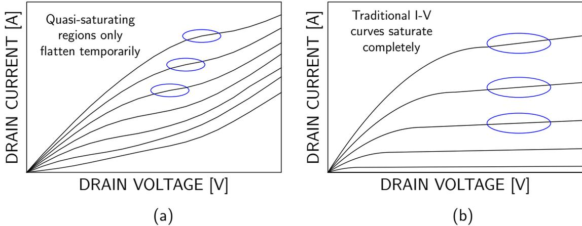
Figure 1.2: (a) Graphene vs. traditional (b) MOSFET  $I$ - $V$  curves. The graphene  $I$ - $V$  curves are generated from quantum-mechanical simulations, while the MOSFET  $I$ - $V$  curves are plotted using the standard piecewise functions [26].
