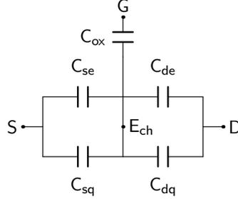
Figure A.11: Equivalent circuit between the external terminals and the channel as derived from a general theory of ballistic nanotransistors [157], [158].
