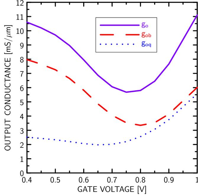
Figure 2.9: Output conductance  $g_o$  and its components  $g_{ob}$  and  $g_{oq}$  vs. gate voltage  $v_G$  for the GFET. The drain voltage is held at  $v_D = V_{DD}/2 = 0.5$  V.
