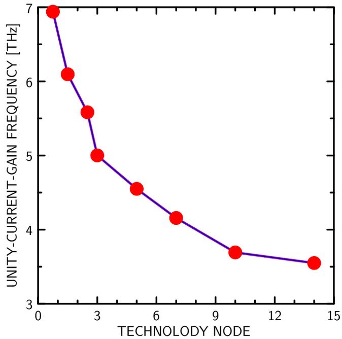
Figure 4.6: Intrinsic unity-current-gain frequency  $f_{T,int}$  vs. technology node. Nodes are identified by their ITRS [3] name in nm, *not* by gate length.
