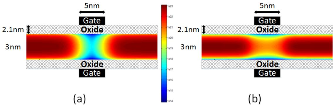
Figure 4.4: Charge distribution in a 5-nm FinFET (a) without and (b) with an appreciable gate voltage. When an appreciable gate voltage is present, the charge density exhibits a single peak, located at the center of the channel.
