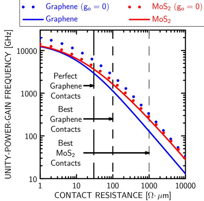
Figure 3.7: Peak unity-power-gain frequency  $f_{\max}(\rho_C)$  vs. the contact resistance  $\rho_C$  determining the source and drain resistances  $R_s$  and  $R_d$ , with  $R_g$  held at  $1 \Omega$ , as discussed in the text.
