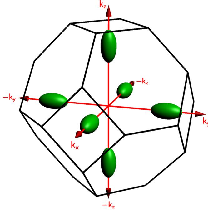
Figure 4.2: The first Brillouin zone of silicon along with the six constant-energy ellipsoids in reciprocal space. Each ellipsoid represents one valley minimum in the electronic structure.
