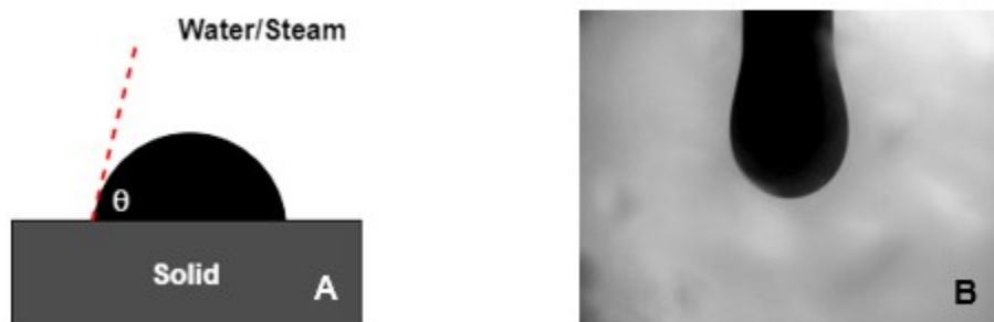
Figure 45—(a) contact angle and (b) pendant drop methodology.
