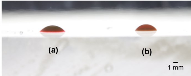
Figure 96—Wettability state observation on plexiglass surface for (a) 450 cP and (b) 111,600 cP mineral oils at 25°C.
