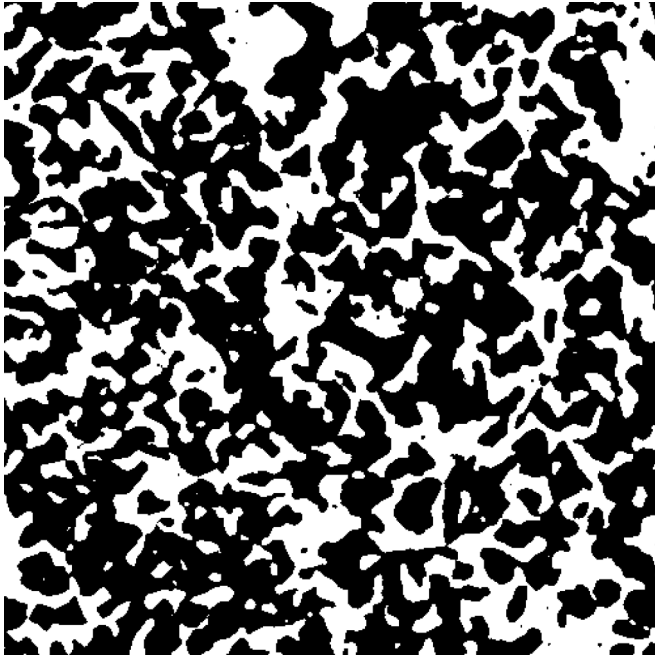
FIG. 9. Binarized SEM image of a ceramic used as reference image for 3D reconstruction (black shows the solid phase, and white shows the void phase).
