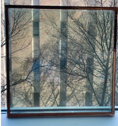
Figure D-2. Digital image of a large-area dynamic window.
