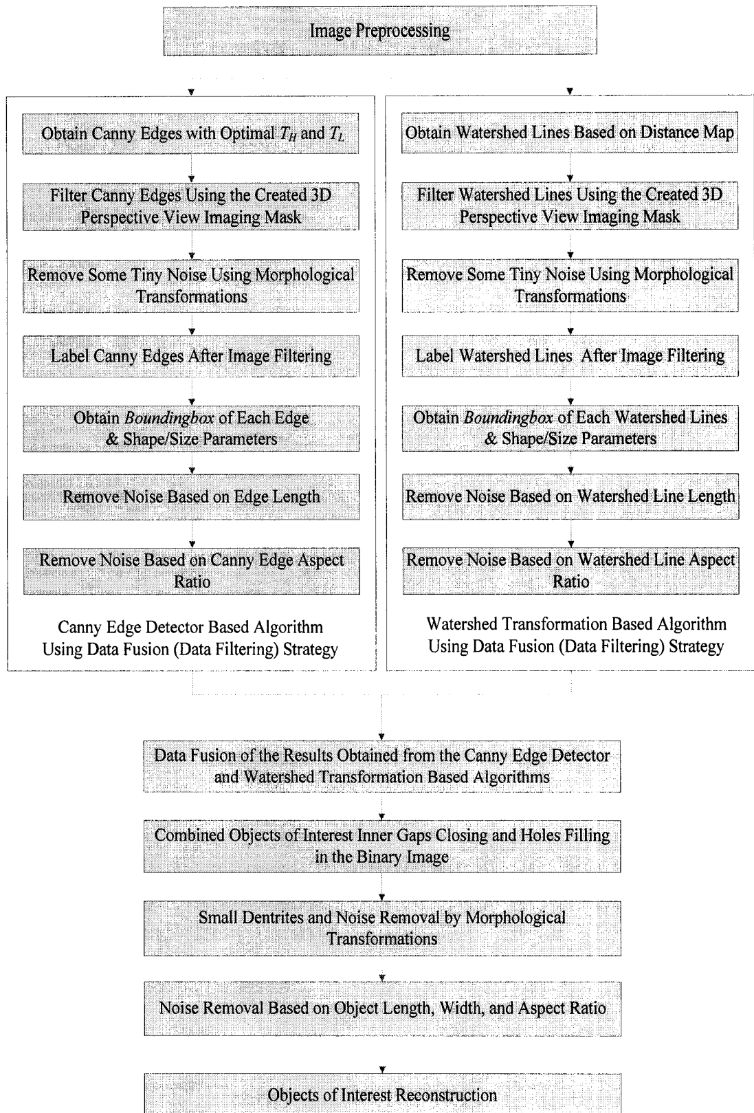
Figure 3.5: The Proposed Image Segmentation Approach Using the Data Fusion Strategy
