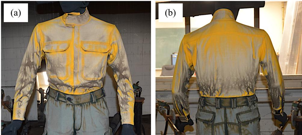
Figure 7.2 Control shirt number 2 after the full-scale flame engulfment for 4 seconds: (a) front view, and (b) back view.
