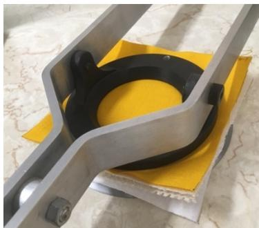
Figure 3.12 Fabric system OL-3D1-BL mounted in clamps of air permeability testing apparatus.
