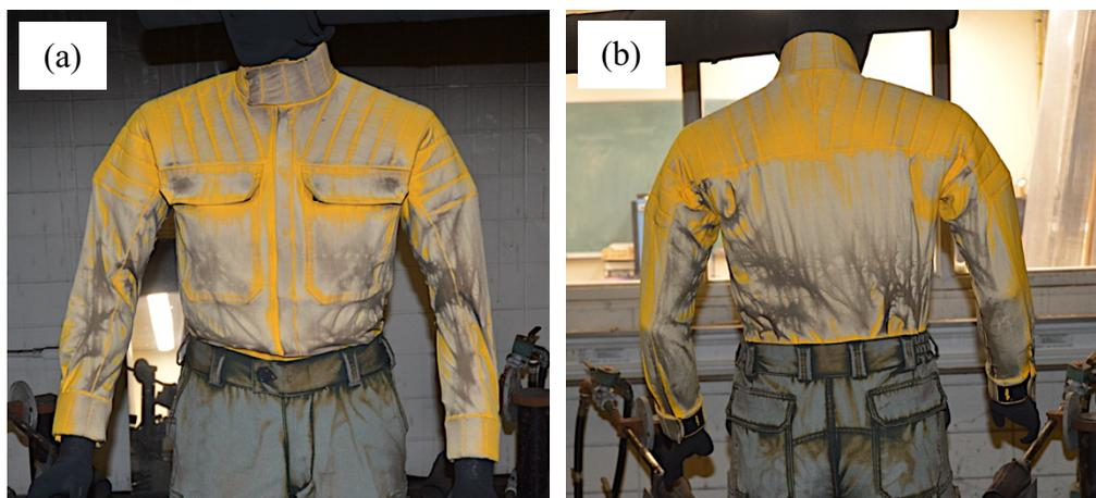
Figure E.8 Prototype shirt number 3 after the full-scale flame engulfment for 4 seconds: (a) front, and (b) back.
