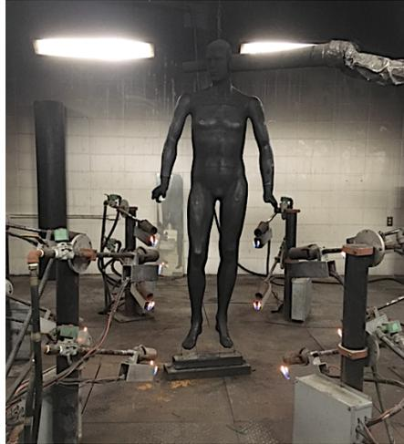
Figure 3.13 Instrumented manikin.
