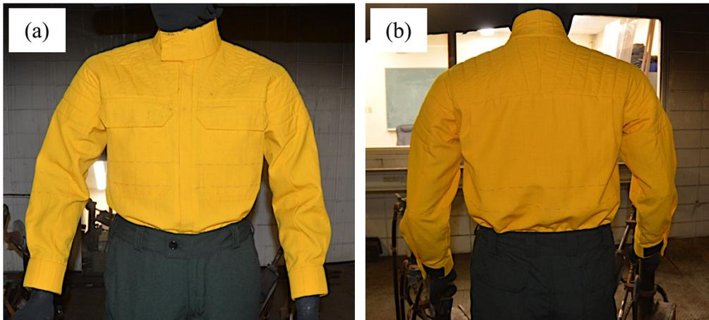
Figure E.5 Prototype shirt number 1 before the full-scale flame engulfment for 4 seconds: (a) front, and (b) back.
