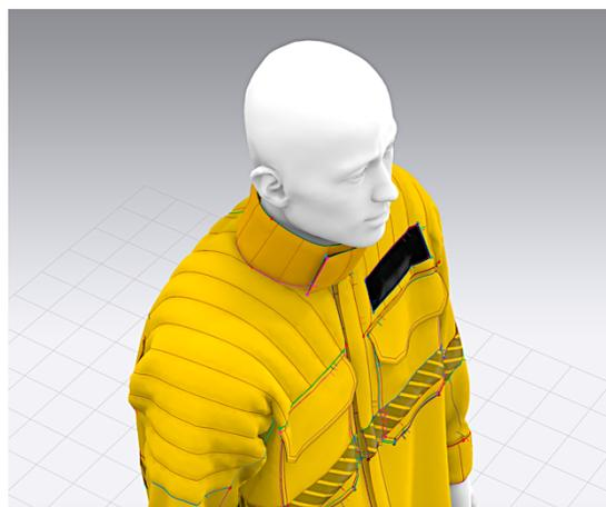
Figure 6.6 Top view of modified yoke in simulated prototype shirt.
