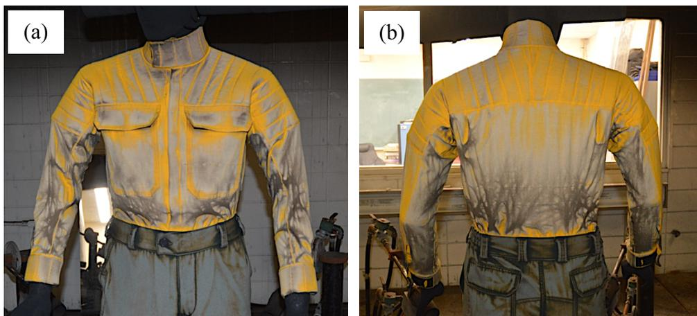
Figure E.6 Prototype shirt number 1 after the full-scale flame engulfment for 4 seconds: (a) front, and (b) back.
