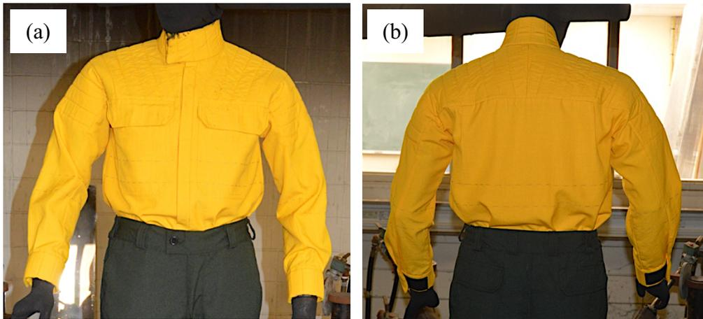
Figure 7.4 Prototype shirt number 2 before the full-scale flame engulfment for 4 seconds: (a) front view, and (b) back view.
