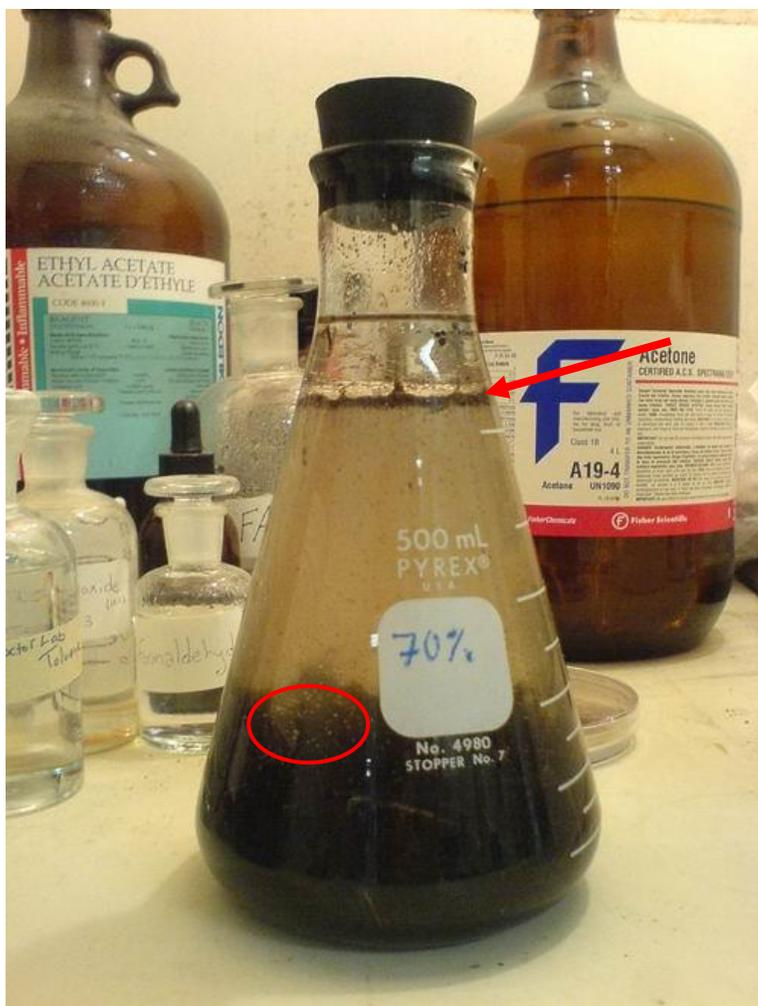
Figure III.1: Notice the small air bubbles inside after 15 minutes in the vacuum chamber. Also, more importantly, the ETOH-kerosene interface is clearly visible (brown muck); this is what you siphon up.
