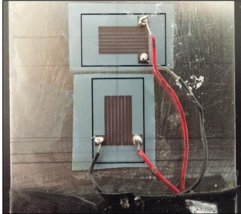
**Figure 3.23 - Resistive PSGs installed on the four points bending specimens.**
