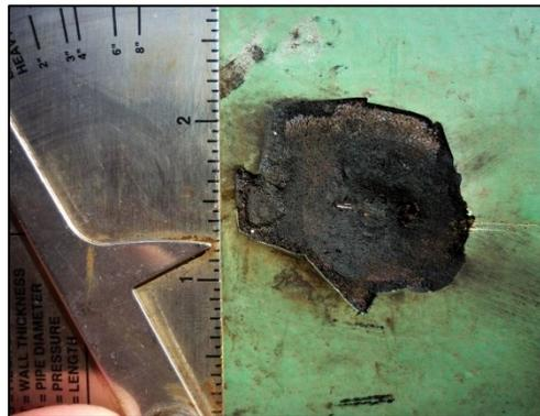
**Figure 2.5 - Local corrosion on pipeline [9].**
