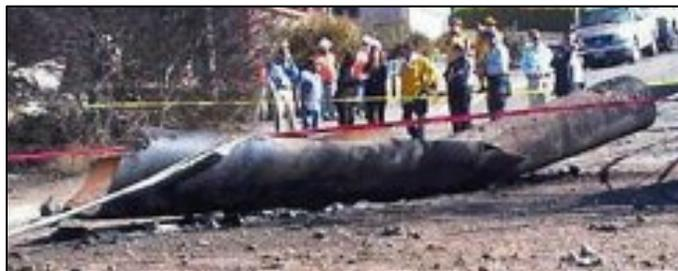
**Figure 2.4 - Rupture of the pipeline [57].**
