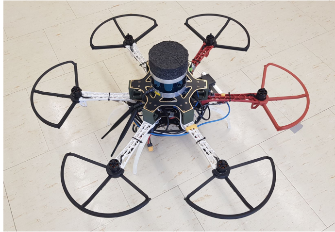
Figure 4.6: DJI FlameWheel F550 hexacopter vehicle equipped with onboard sensors and computing systems.
