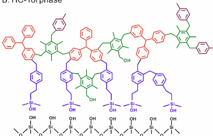
**Figure 1-3** Structure of the hypercrosslinked polystyrene and HC-Tol phase. The colors reflect the individual components and steps within the synthesis. Black signifies the underlying silica, blue means the silanization step, red indicates the primary crosslinking step, green is the secondary crosslinking, and purple is the final derivatization with toluene. A adapted from Ref [42], B adapted from Ref. [43].
