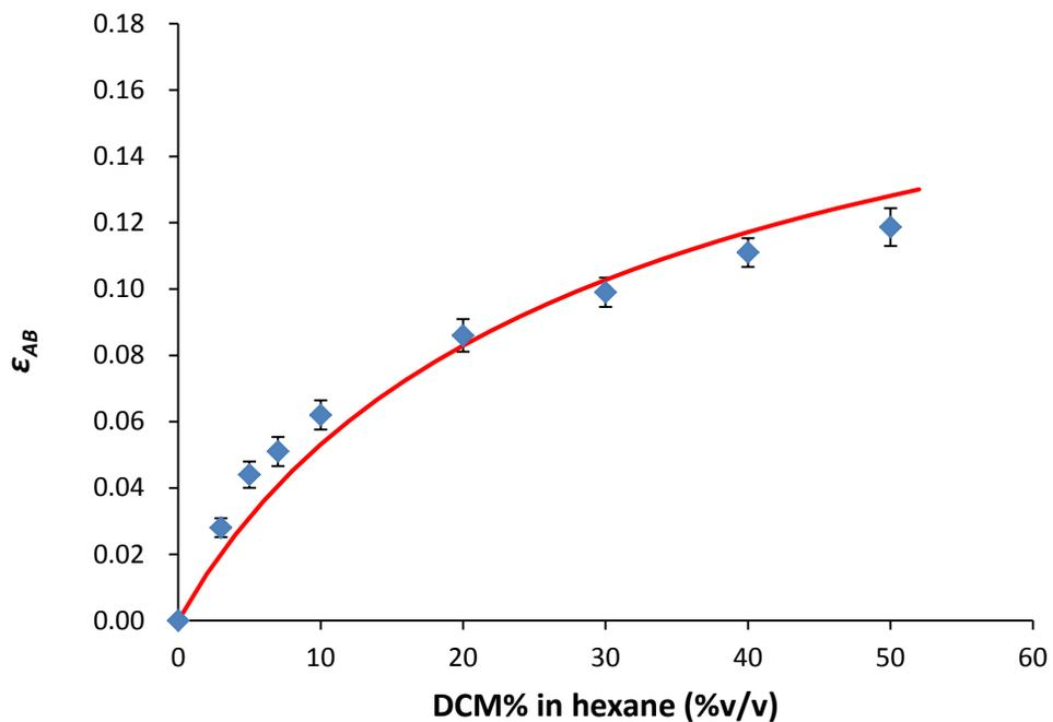
**Figure 2-2** Dependence of solvent strength on mobile phase composition. Conditions: column, HC-Tol, 50×4.6 mm i.d.; temperature, 35 °C; flow rate, 1.0 mL/min; detection, 254 nm; injection volume, 1 μL. Error bar is 95% confidence interval. (◆) experimental; (—) predicted by Eq. 2-2.
