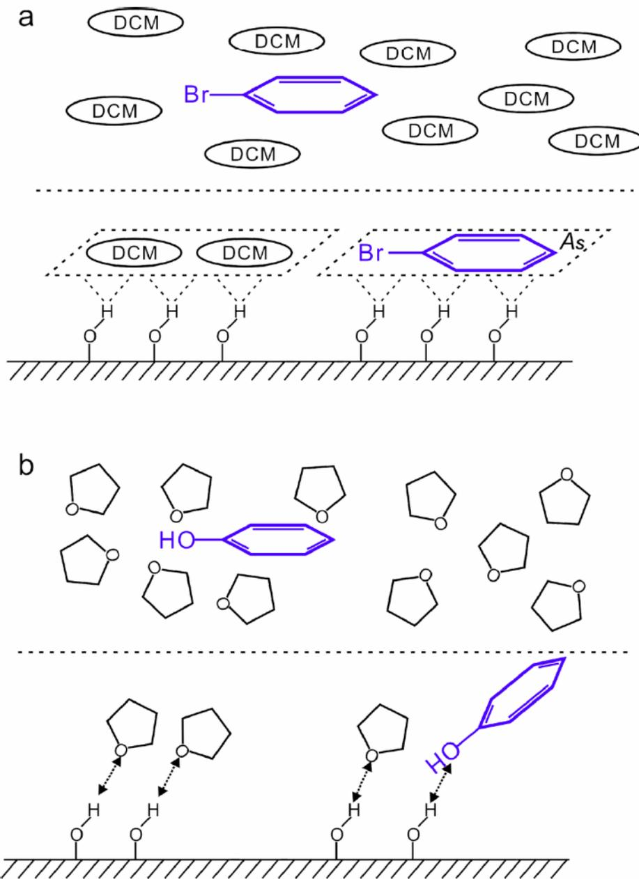
**Figure 2-1** Illustration of solute and solvent localization: a) nonlocalizing solvent dichloromethane (DCM) and nonlocalizing solute bromobenzene; and b) localizing solvent tetrahydrofuran (THF) and localizing solute phenol. Adapted from [39].
