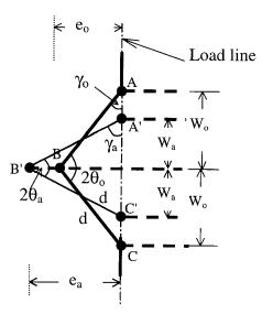
Figure 8.12: Wrinkle of axial pipe specimen under cyclic axial load
