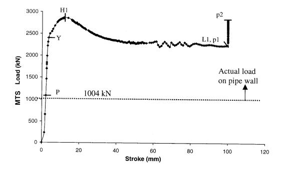
Figure 3.7: MTS Load vs. MTS Stroke for Specimen 1
