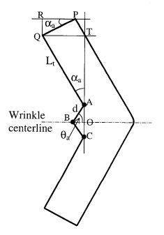
Figure 8.14: Model for deformed shape of a bending pipe specimen
