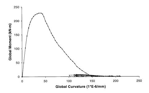
Figure 6.28: Moment-Curvature curve obtained from Test 12
