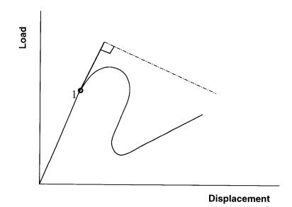
Figure 5.14: Riks method fails at snap-back behavior
