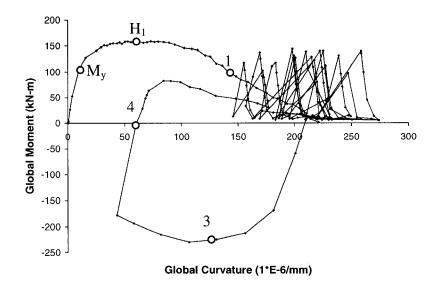
Figure 6.22: Moment-Curvature curve obtained from Test 9
