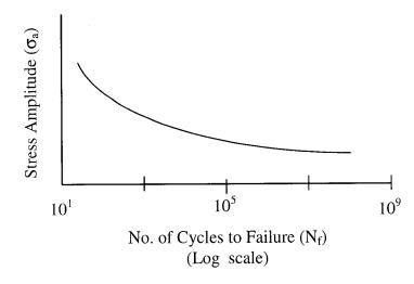
Figure 2.3: Schematic plot for a S-N curve
