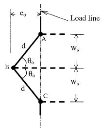
Figure 8.11: Detail Q of pipe wrinkle
