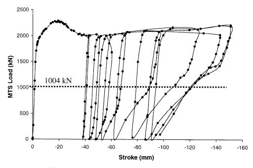
Figure 3.12 : MTS load vs. MTS stroke for Specimen 5
