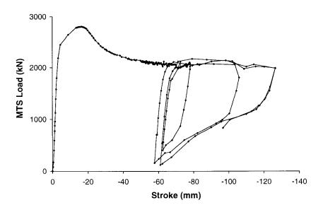
Figure 6.7: Load-Deformation curve obtained from Test 3
