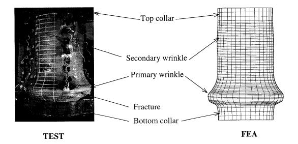
Figure 6.11: Final deformed shape of Specimen 3
