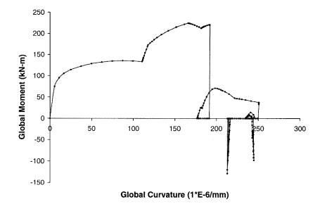
Figure 6.27: Moment-Curvature curve for Specimen 11 obtained from FEA
