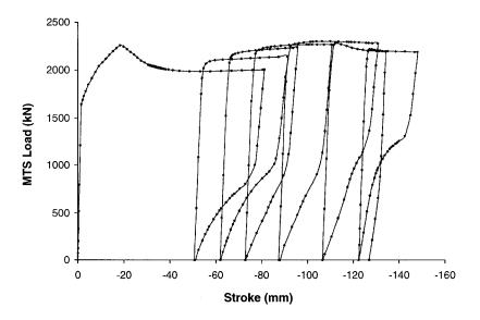
Figure 6.16: Load-Deformation curve of Specimen 7 obtained from FEA
