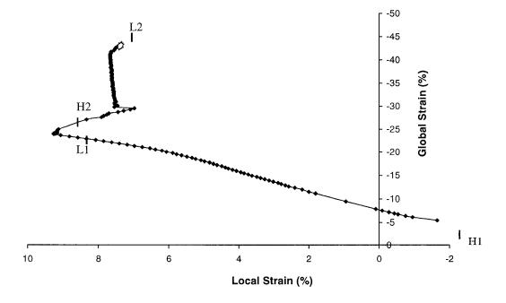
Figure 4.8: Clip-gauge strain vs. Global strain for Specimen 2
