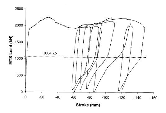
Figure 3.14: MTS Load vs. MTS Stroke for Specimen 7
