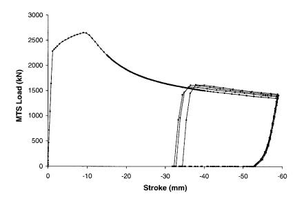
Figure 6.14: Load-Deformation curve for Specimen 6 obtained from FEA
