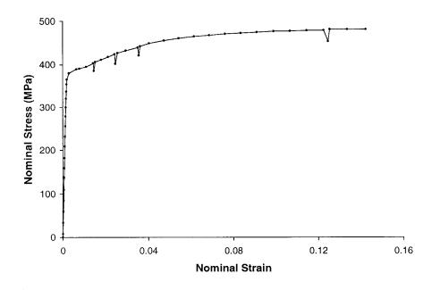
Figure 4.19: Typical engineering stress-strain behavior
