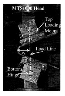
Figure 7.5: Strip specimen mounted on to MTS 1000 machine
