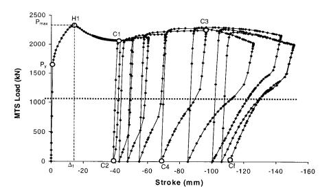
Figure 6.2: Load-Deformation curve for Specimen 5 obtained from FEA
