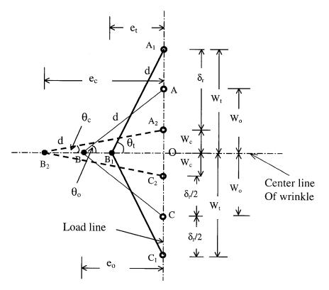
Figure 8.9: Model for strip specimen under cyclic load
