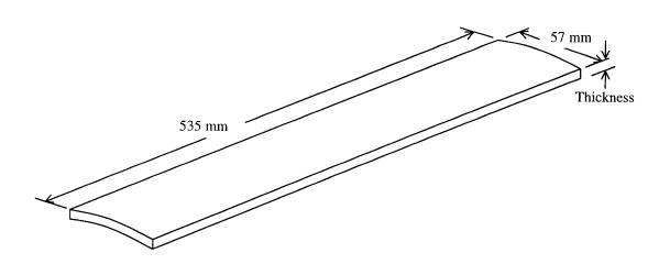
Figure 7.2: Schematic of a strip
