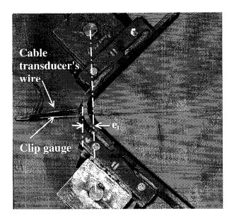
Figure 7.7: Strip specimen subjected to maximum tension
