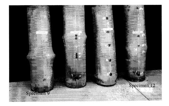
Figure A14b : Family photo for bending Specimens 9 to 12, seen from tension side
