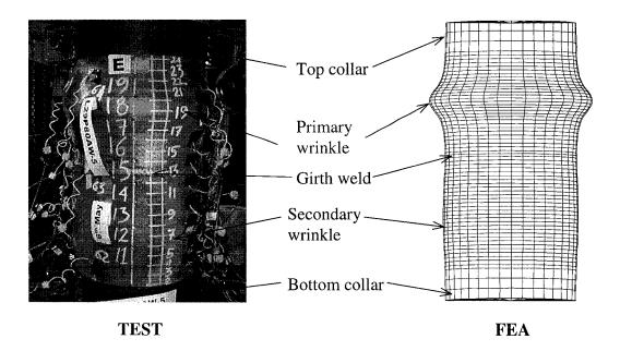
Figure 6.3: Deformed shape of Specimen 5 at Point C1
