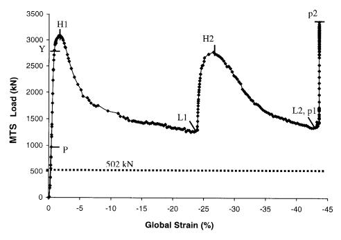
Figure 3.8 : MTS Load vs. MTS Stroke for Specimen 2
