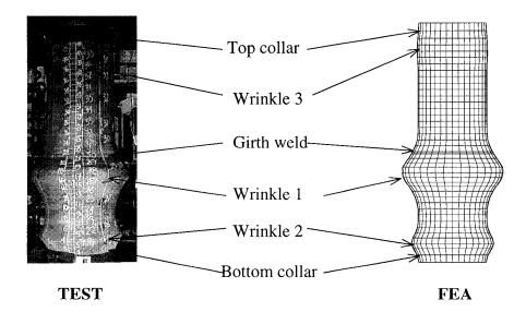
Figure 6.20: Final deformed shape of Specimen 7
