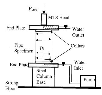
Figure 3.2: A schematic of test setup for axial plane pipe specimens
