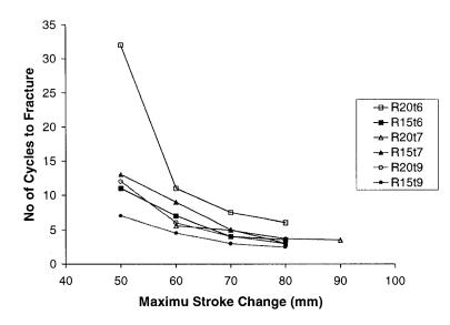
Figure 7.25: Maximum stroke change vs. Number of cycles to fracture from *strip* tests
