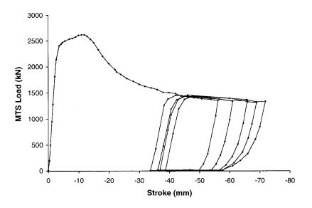
Figure 6.17: Load-Deformation curve obtained from Test 8
