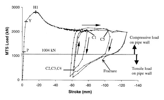
Figure 3.10: MTS Load vs. MTS Stroke for Specimen 3
