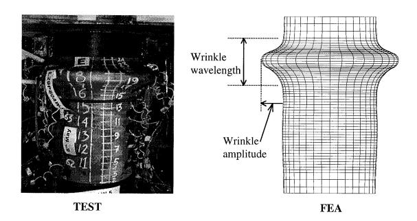
Figure 6.4: Deformed shape of Specimen 5 at Point C3
