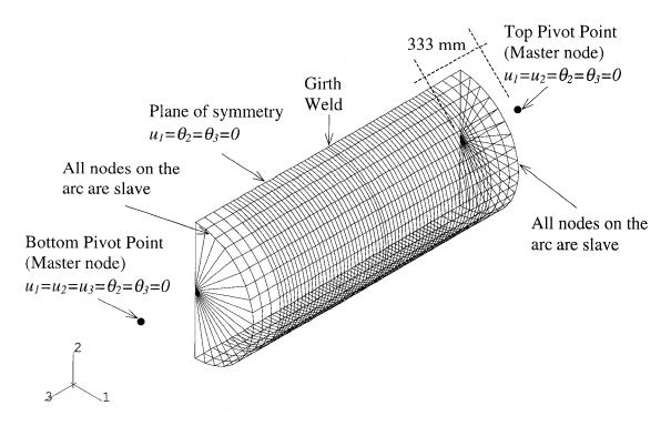
Figure 5.1: Typical geometry and boundary condition for the pipes
