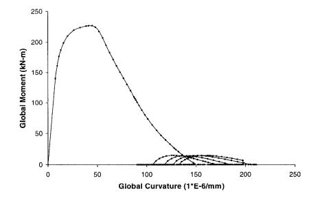
Figure 6.29: Moment-Curvature curve for Specimen 12 obtained from FEA
