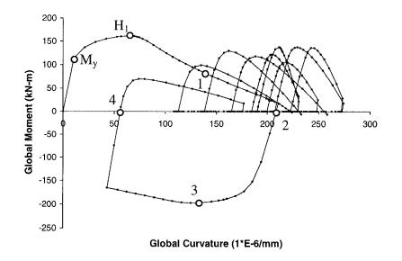
Figure 6.23: Moment-Curvature curve for Specimen 9 obtained from FEA
