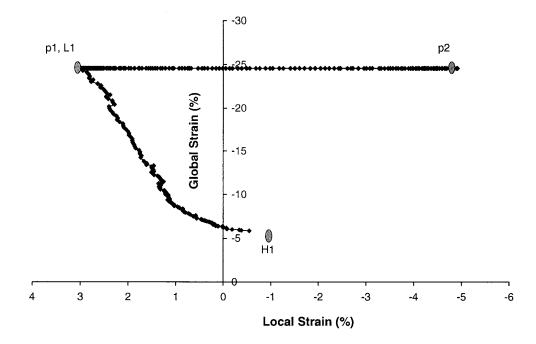
Figure 4.4: Clip-gauge strain vs. Global strain for Specimen 1
