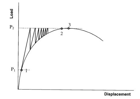
Figure 5.12: Modified Newton's method
