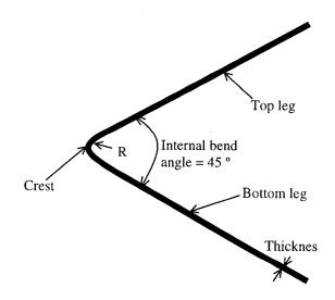
Figure 7.4: Schematic of a bent strip
