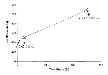
Figure 5.5: True stress-True total strain behavior till fracture
