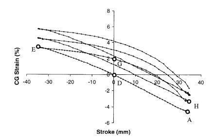
Figure 7.22: A part of CG strain hysteresis for a strip specimen
