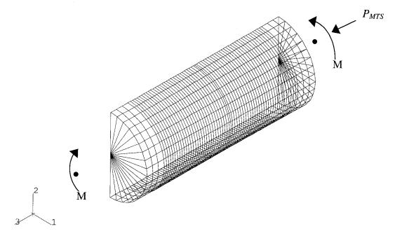
Figure 5.2: Typical concentrated loading for the pipes
