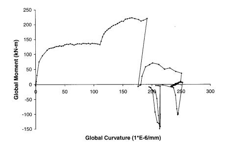
Figure 6.26: Moment-Curvature curve obtained from Test 11
