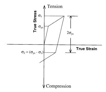
Figure 5.8: Uniaxial kinematic hardening model in ABAQUS
