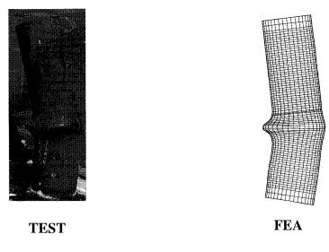
Figure 6.32: Final deformed shape of Specimen 9
