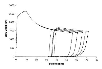
Figure 6.18: Load-Deformation curve of Specimen 8 obtained from FEA
