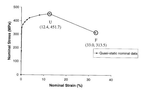
Figure 5.4: Nominal quasi-static stress-strain behavior till fracture
