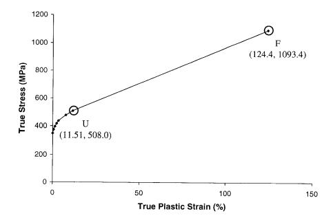
Figure 5.6: True stress-True plastic strain behavior till fracture
