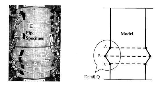
Figure 8.10: Actual wrinkled pipe specimen and its model
