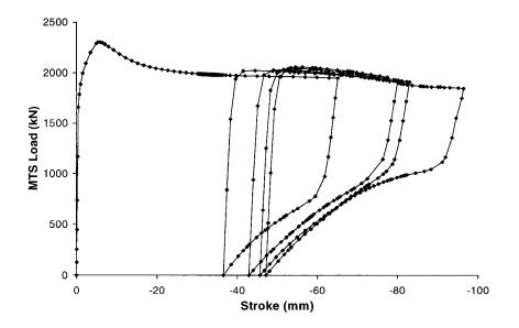
Figure 6.10: Load-Deformation curve of Specimen 4 obtained from FEA
