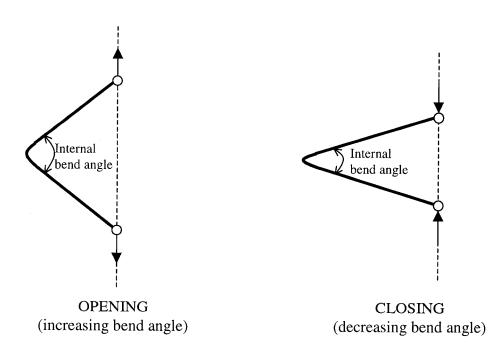
Figure 7.16: Schematic of opening and closing of a strip specimen
