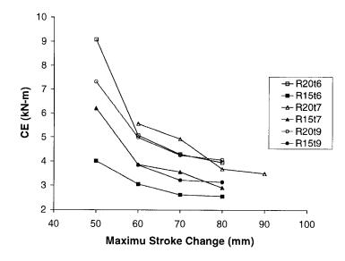
Figure 7.24: Maximum stroke change vs. cumulative energy from *strip* tests
