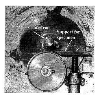
Figure 7.9: Top view of bar bending machine
