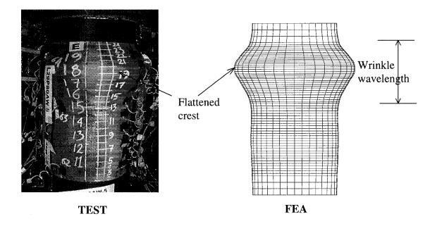
Figure 6.5: Deformed shape of Specimen 5 at Point C4
