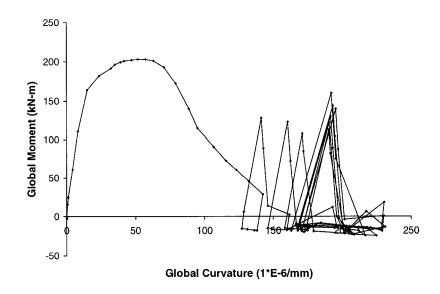
Figure 6.24: Moment-Curvature curve obtained from Test 10
