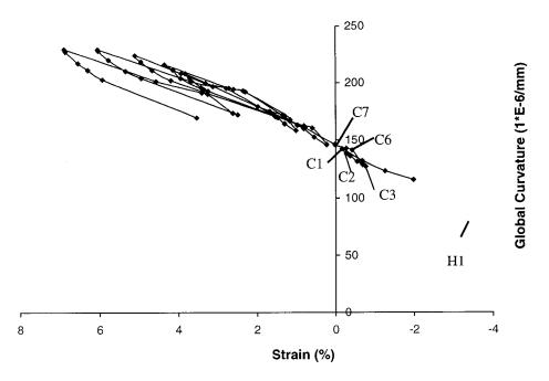
Figure 4.17: Clip-gauge strain vs. Global curvature for Specimen 10
