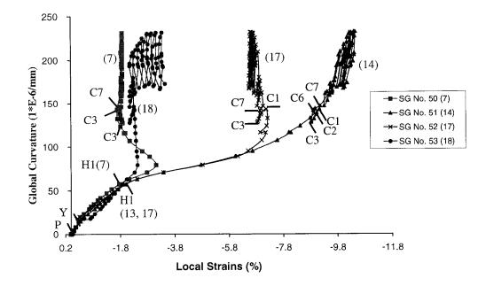
Figure 4.15: Local longitudinal strain vs. Global strain for Specimen 10
