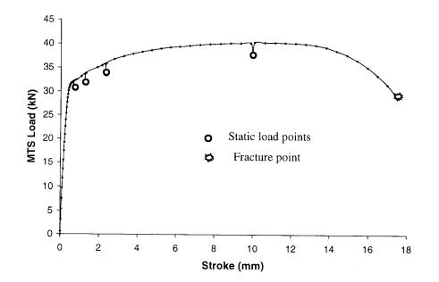
Figure 3.19: Typical load vs. stroke plot for a tension coupon specimen
