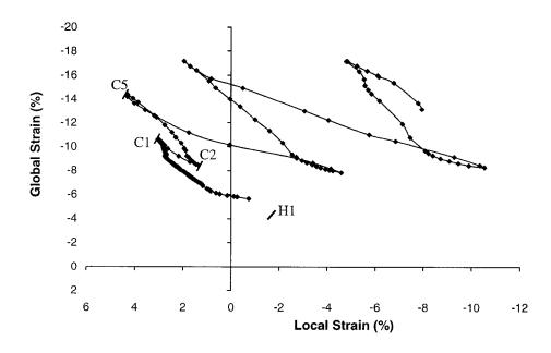
Figure 4.13: Clip-gauge strain vs. Global strain for Specimen 3
