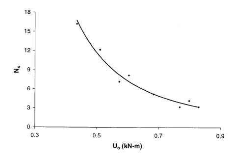
Figure 8.1: U<sub>o</sub> vs. N<sub>s</sub> relationship for 6.84 mm thick strip specimens
