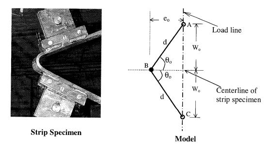
Figure 8.8: Actual strip specimen and its model
