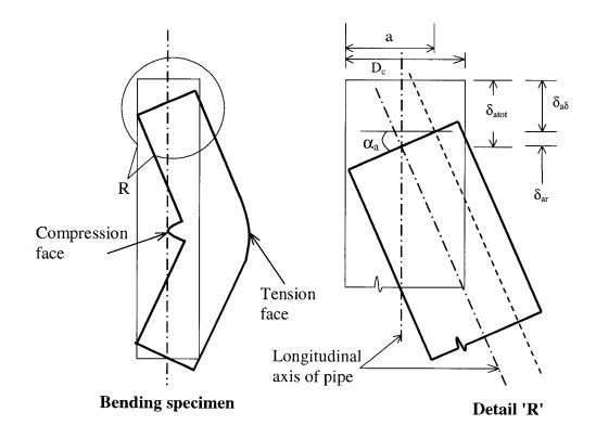
Figure 8.13: Bending pipe specimen and its detail 'R'
