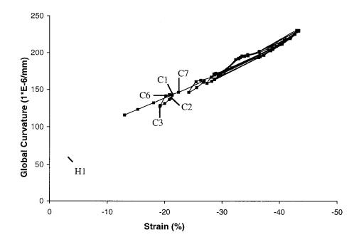
Figure 4.18: Extensometer strain vs. Global curvature for Specimen 10
