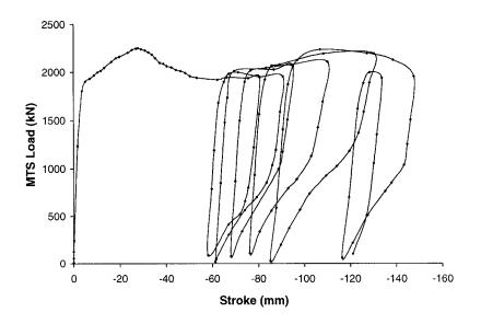
Figure 6.15: Load-Deformation curve obtained from Test 7
