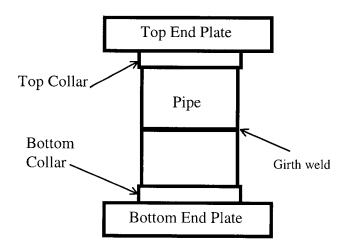
Figure 3.1: A schematic of a girth-welded pipe specimen
