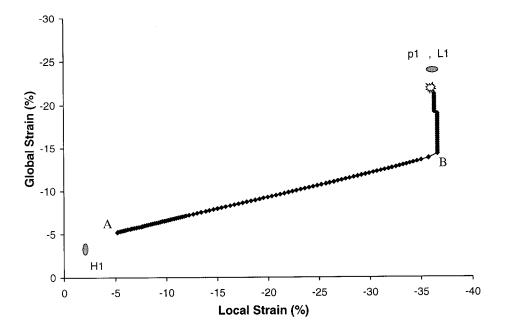
Figure 4.5: Extensometer strain vs. Global strain for Specimen 1
