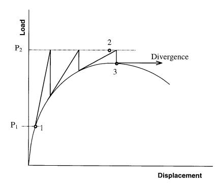
Figure 5.15: Load control process fails at limit point
