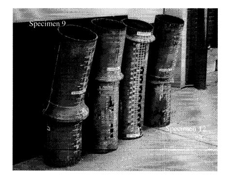
Figure A14a : Family photo for bending Specimens 9 to 12, seen from compression side
