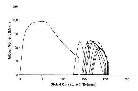
Figure 6.25: Moment-Curvature curve for Specimen 10 obtained from FEA
