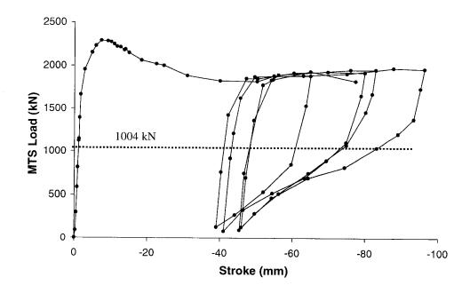
Figure 3.11: MTS Load vs. MTS Stroke for Specimen 4
