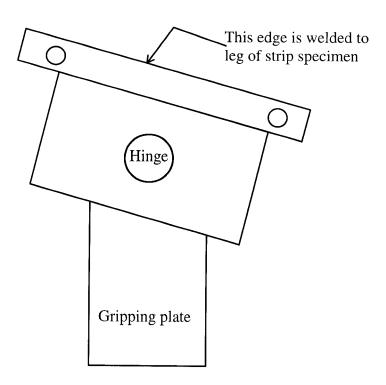
Figure 7.6: Custom made loading mount
