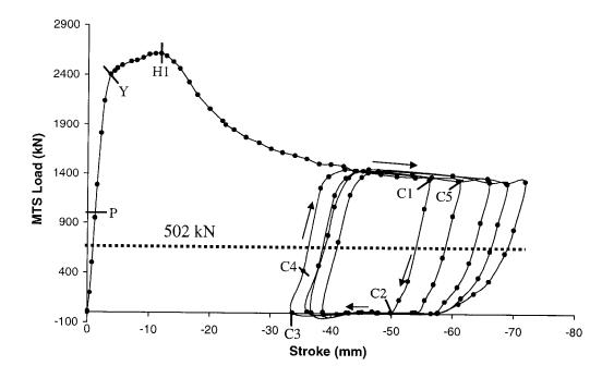
Figure 3.15: MTS load vs. MTS stroke for Specimen 8
