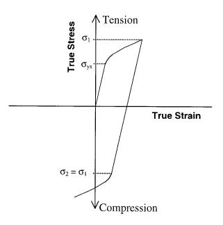
Figure 5.7: Uniaxial isotropic hardening model in ABAQUS
