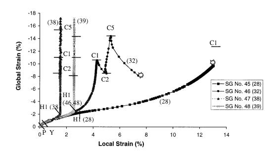
Figure 4.12: Local circumferential strain vs. Global strain for Specimen 3
