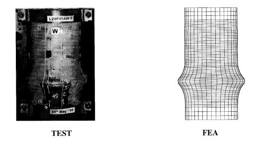
Figure 6.21: Final deformed shape of Specimen 8
