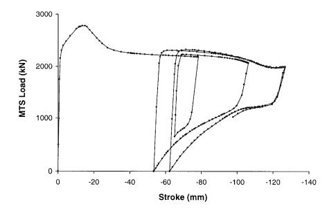
Figure 6.8: Load-Deformation curve of Specimen 3 obtained from FEA
