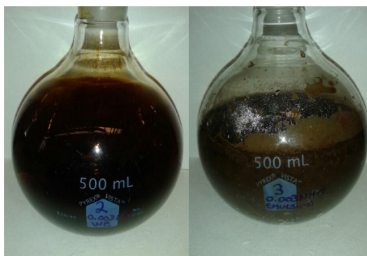
Product 0.003M HCl after acid treatment without emulsion (B-HCl-WE) Separation of emulsion after acid treatment (E)
