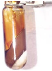
Figure 2-21: After centrifuging, the centrifuge tubes included, dry oil, brine and a middle layer of \sim 90\% emulsion [53].
