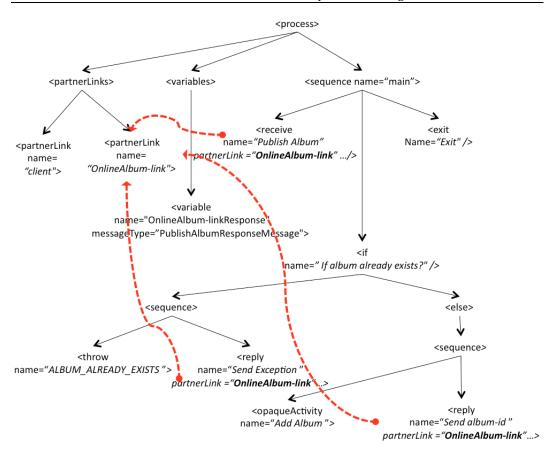
Figure 2-8: A BPEL process workflow represented as a tree
