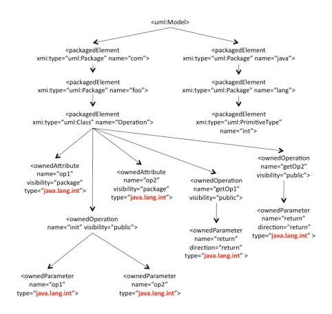
Figure 2-9: A UML/XMI sample represented as a tree structure
