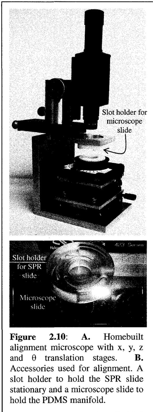
**Figure 2.10:** **A.** Homebuilt alignment microscope with x, y, z and  $\theta$  translation stages. **B.** Accessories used for alignment. A slot holder to hold the SPR slide stationary and a microscope slide to hold the PDMS manifold.
