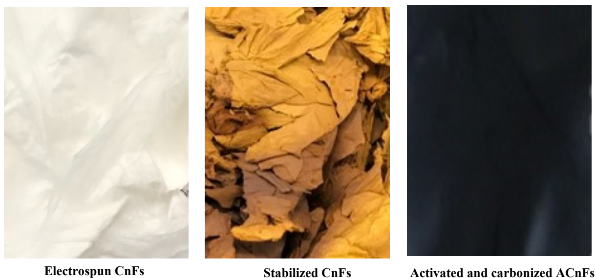
Figure 3.1 Form and shape of electrospun CnFs, stabilized, and activated and carbonized ACnFs
