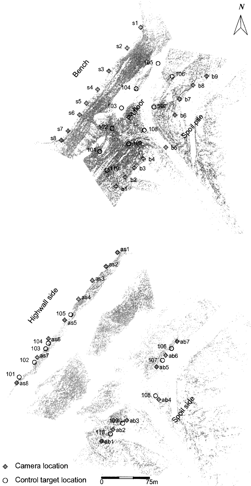
Figure 76 Blast #3: Pre-blast and post-blast point-cloud models - plan view
