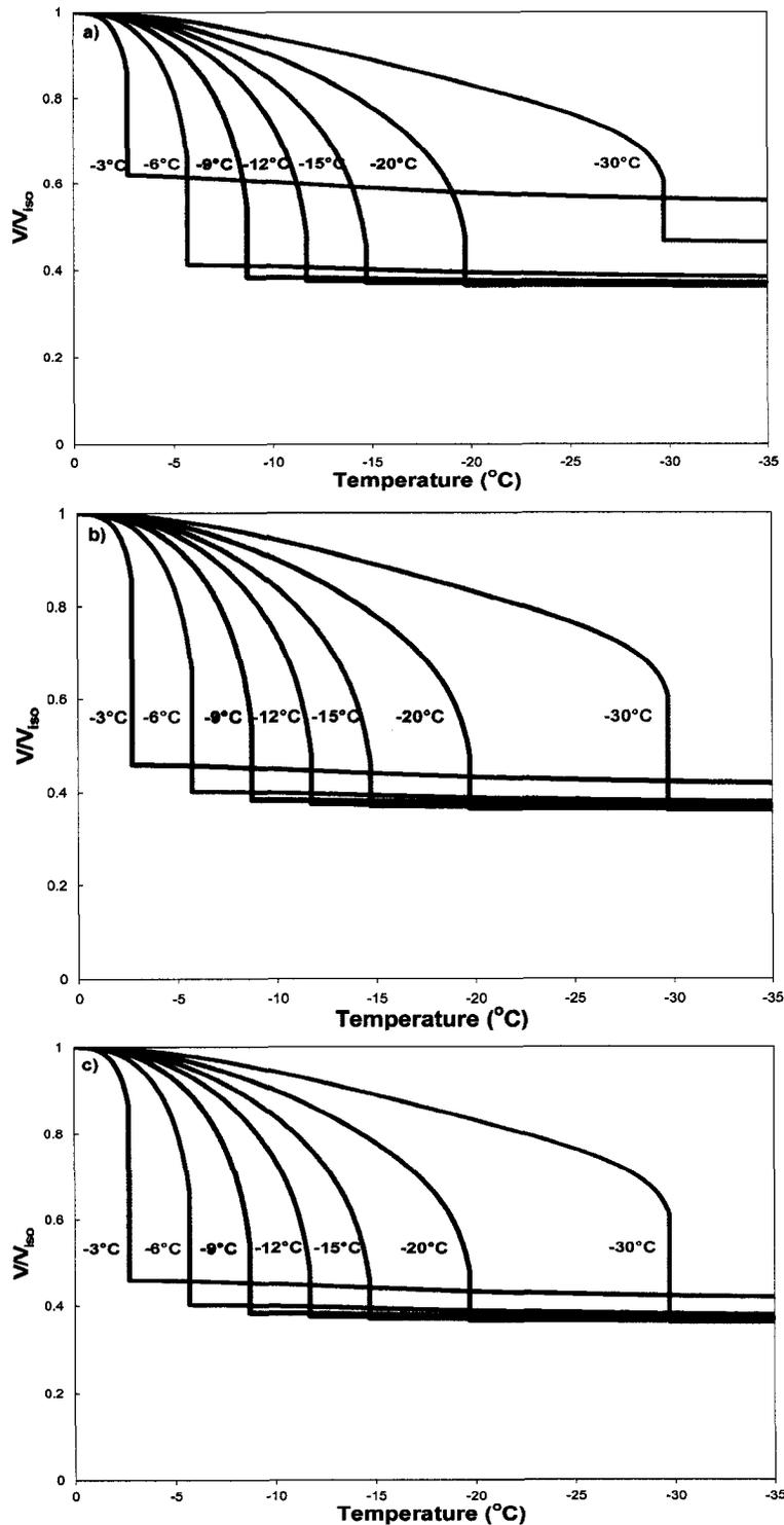
Figure 5-3. Volume as a function of temperature for TF-1 cells using Fourier's Law (constant=7) to various subzero plunge temperatures ( $-3^{\circ}\text{C}$  to  $-40^{\circ}\text{C}$ ) and held at that temperature for (a) 0.5 min., (b) 3 min., and (c) 10 min., prior to being plunged to  $-40^{\circ}\text{C}$  ( $325^{\circ}\text{C}/\text{min}$ ).
