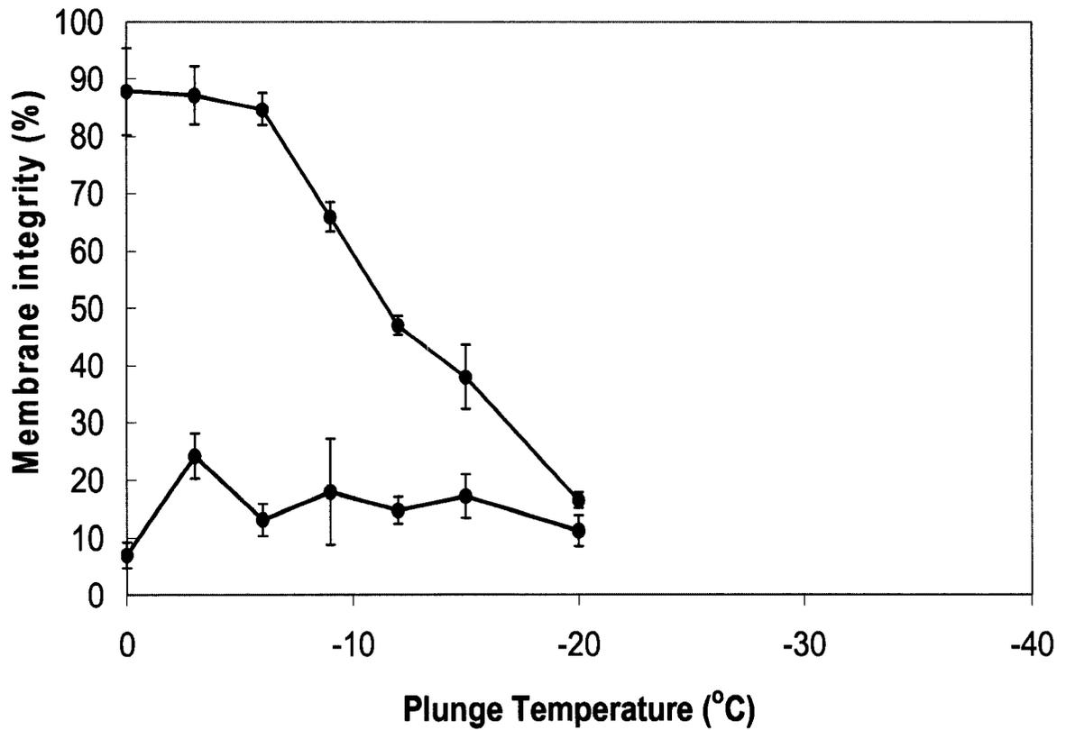
Figure 4-2. Membrane integrity of TF-1 cells ( $\pm$ SEM) in serum-free RPMI media after being cooled at  $0.2^{\circ}\text{C}/\text{min}$  to various subzero plunge temperatures and then either thawed directly (upper curve) or plunge into liquid Nitrogen (lower curve) prior to thawing.
