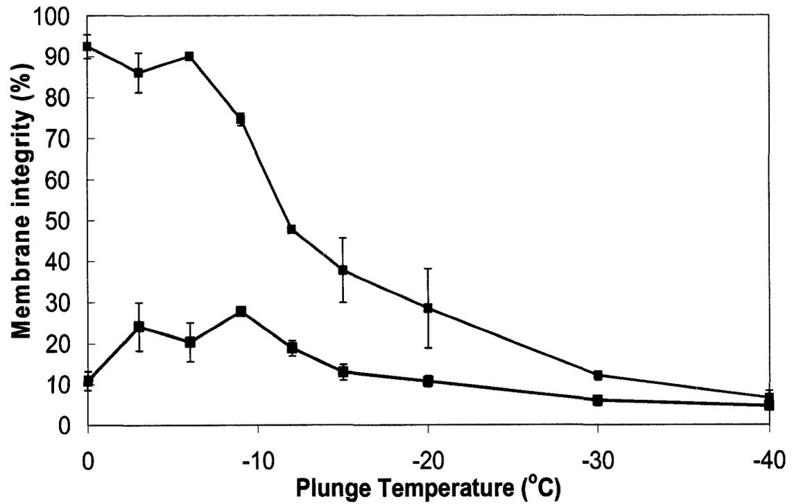
Figure 4-4. Membrane integrity of TF-1 cells ( $\pm$ SEM) in serum-free RPMI media after being cooled at 0.9°C/min to various subzero plunge temperatures and either thawed directly (upper curve) or plunge into liquid Nitrogen (lower curve) prior to thawing.
