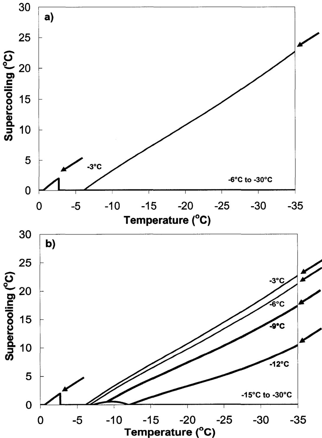
Figure 3-4. A representative graph of supercooling versus temperature for TF-1 cells cooled using Fourier's Law ( $k=7$ ) to  $-3^{\circ}\text{C}$  and then cooled (a) at  $1^{\circ}\text{C}/\text{min}$  and (b) at  $100^{\circ}\text{C}/\text{min}$  to various subzero plunge temperatures ( $-4$  to  $-30^{\circ}\text{C}$ ), prior to being plunged  $-40^{\circ}\text{C}$  ( $325^{\circ}\text{C}/\text{min}$ ). Arrows indicate maximum supercooling.
