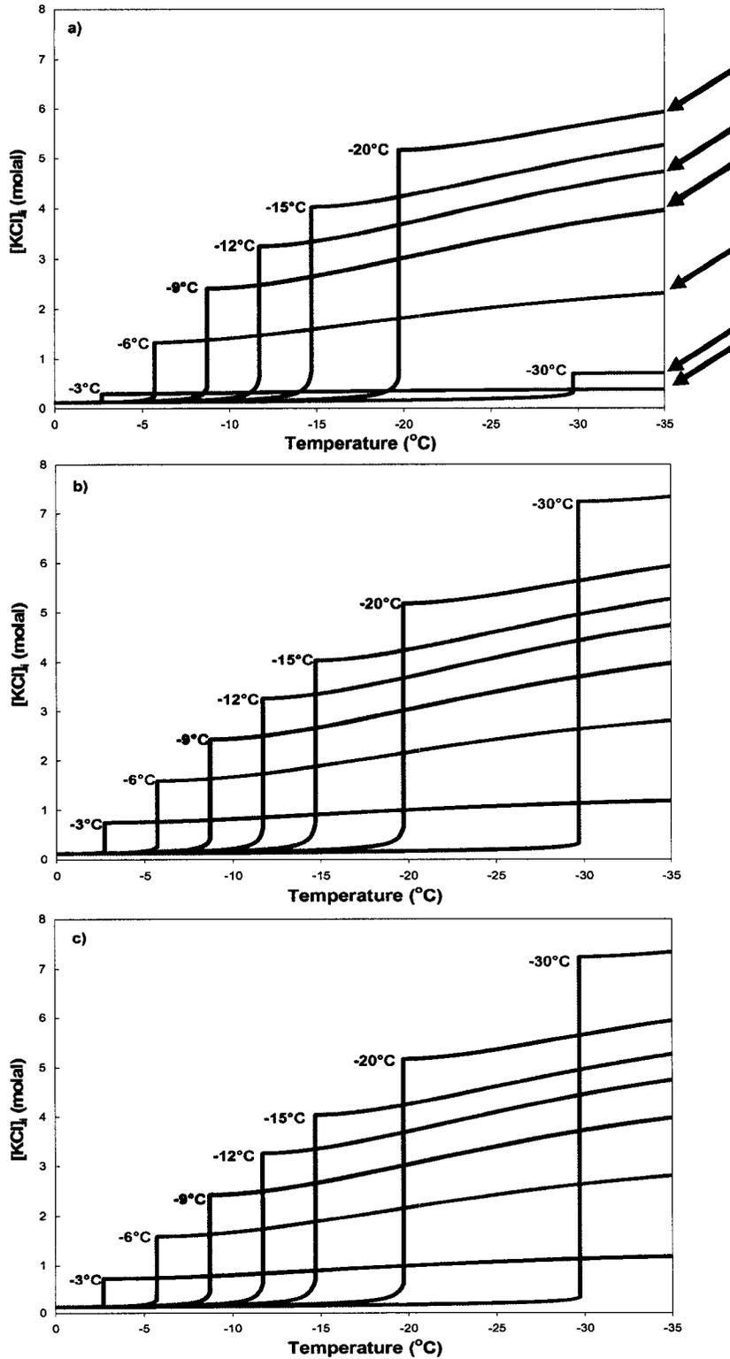
Figure 5-5.  $[KCl]_i$  as a function of temperature for TF-1 cells using Fourier's Law to various subzero plunge temperatures ( $-3^{\circ}\text{C}$  to  $-40^{\circ}\text{C}$ ) and held at that temperature for (a) 0.5 min., (b) 3 min., and (c) 10 min., prior to being plunged to  $-40^{\circ}\text{C}$  ( $325^{\circ}\text{C}/\text{min}$ ). Arrows indicate maximum  $[KCl]_i$ .
