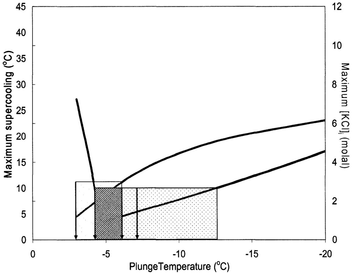
Figure 5-7. Maximum [KCl]<sub>i</sub> and maximum supercooling as a function of temperature for TF-1 cells cooled to various subzero plunge temperatures and held at that temperature for 3 min. prior to being plunged to -40°C (325°C/min). The shaded box indicates the optimal plunge temperature of between -4°C and -6°C based on 10°C supercooling and 3 M [KCl]<sub>i</sub>.
