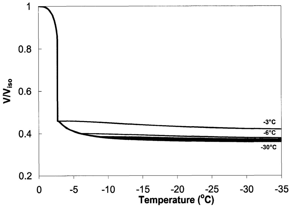
Figure 3-3. A representative graph of volume as a function of temperature for TF-1 cells being cooled using Fourier's Law ( $k=7$ ) to  $-3^{\circ}\text{C}$  and then cooled at  $1^{\circ}\text{C}/\text{min}$  to various subzero plunge temperatures ( $-4^{\circ}\text{C}$  to  $-30^{\circ}\text{C}$ ), prior to being plunged to  $-40^{\circ}\text{C}$  ( $325^{\circ}\text{C}/\text{min}$ ).
