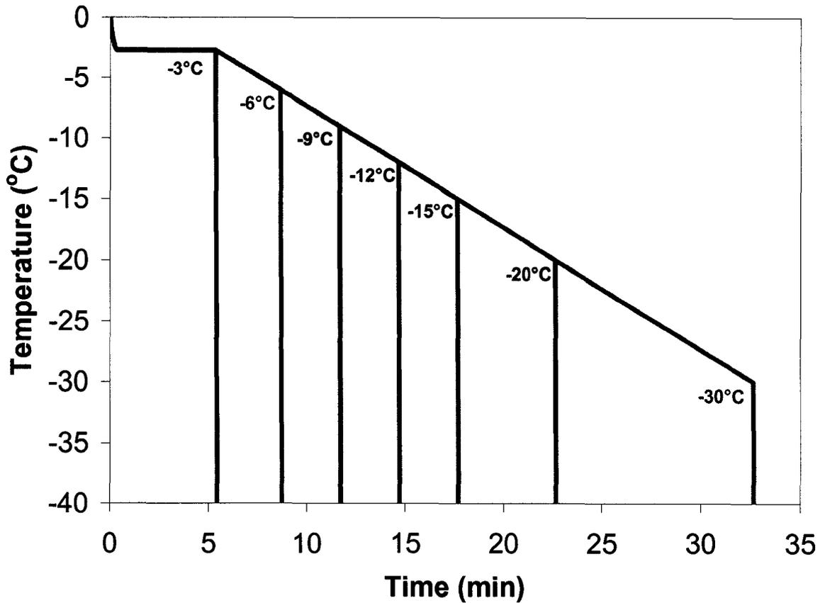
Figure 3-2. A representative graph of the cooling profile for TF-1 cells cooled using Fourier's Law ( $k=7$ ) to  $-3^{\circ}\text{C}$ , held for 5 minutes, cooled at  $1^{\circ}\text{C}/\text{min}$  to various subzero plunge temperatures ( $-4^{\circ}\text{C}$  to  $-30^{\circ}\text{C}$ ) and then plunged to  $-40^{\circ}\text{C}$  ( $325^{\circ}\text{C}/\text{min}$ ).
