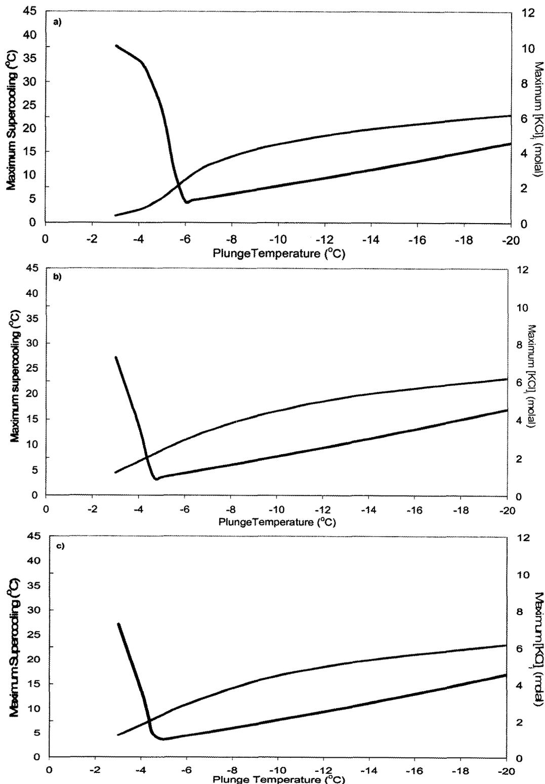
Figure 5-6. Maximum [KCl]<sub>i</sub> and maximum supercooling as a function of temperature for TF-1 cells cooled to various subzero plunge temperatures and held at that temperature for 0.5 min. (a), 3 min. (b), and 10 min. (c), prior to being plunged to -40°C (325°C/min).
