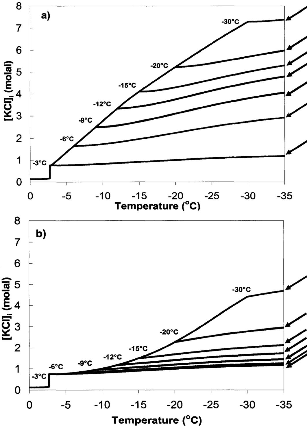
Figure 3-5. A representative graph of  $[KCl]_i$  versus temperature for TF-1 cells cooled using Fourier's Law ( $k=7$ ) to  $-3^{\circ}C$  and then cooled (a) at  $1^{\circ}C/min$  and (b) at  $100^{\circ}C/min$  to various subzero plunge temperatures ( $-4^{\circ}C$  to  $-30^{\circ}C$ ), prior to being plunged to  $-40^{\circ}C$  ( $325^{\circ}C/min$ ). Arrows indicating maximum  $[KCl]_i$ .
