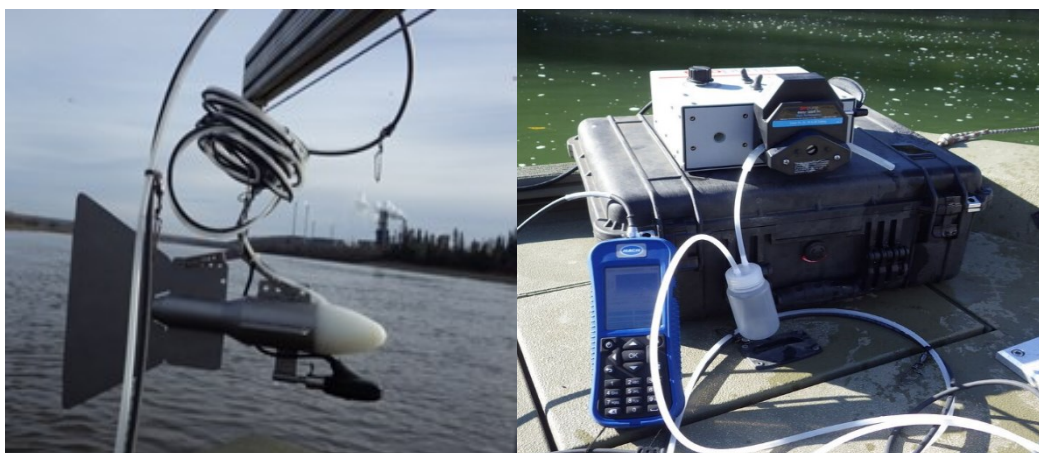
Fig. 2. The SWAMP lab fish, a metal-free depth sampler (left), connected to a peristaltic pump and the velocity meter (right).
