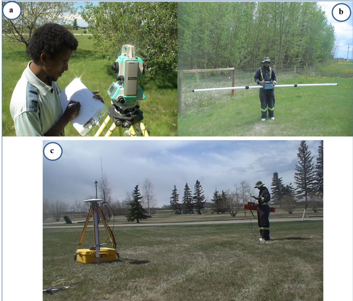
Figure 2-11: Topographic survey (a) and subsurface bulk electrical conductivity (EC) survey (b) EM31 and c) EM38.
