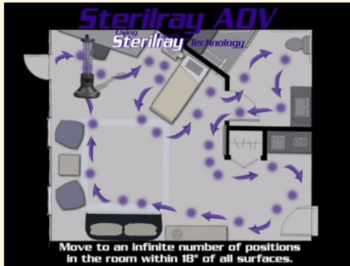
Figure 14. Movement of a Sterilray ADV within a room. 21
