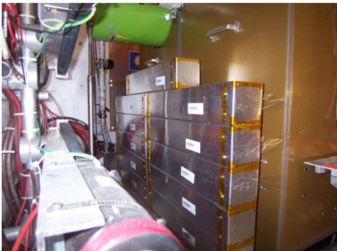
**Figure 2.5:** A photograph of the prototype MMT detector deployed at IP8.
