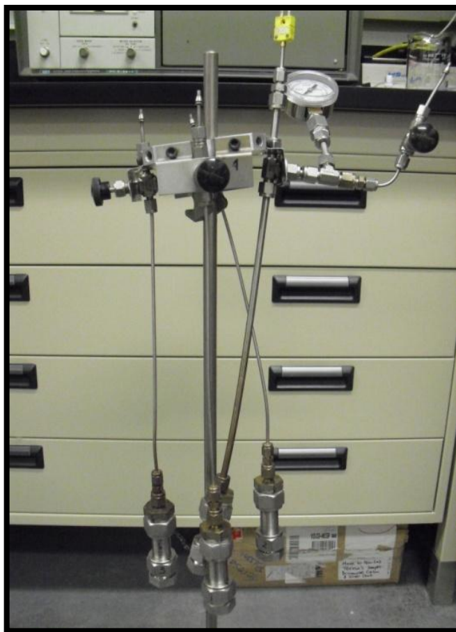
Figure 6-1 The reaction setup, micro-reactors and the holder
