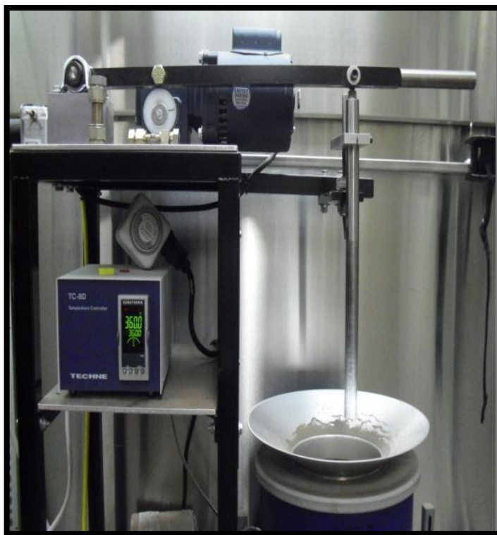
Figure 6-2 the sand bath, agitator and the controller
