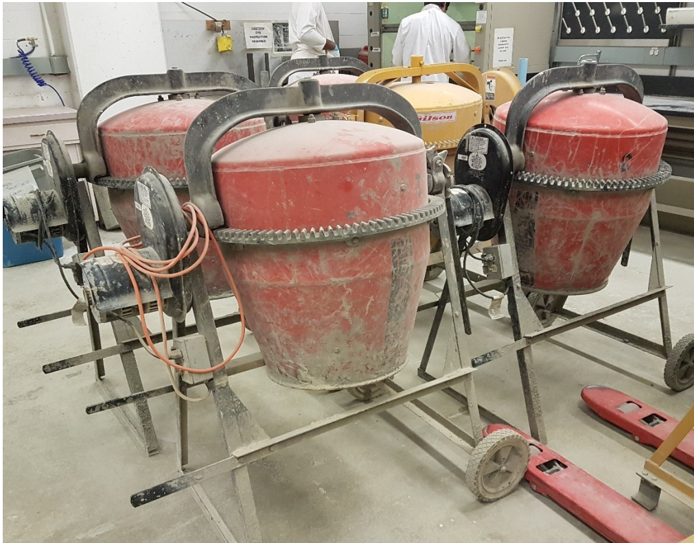
Figure 2.4. Rotary drum concrete mixers for CRF mixing
