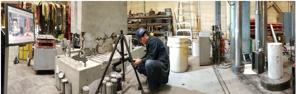
Figure 4.4a. Placement of 3D-DIC instruments, specimen, and load frame
