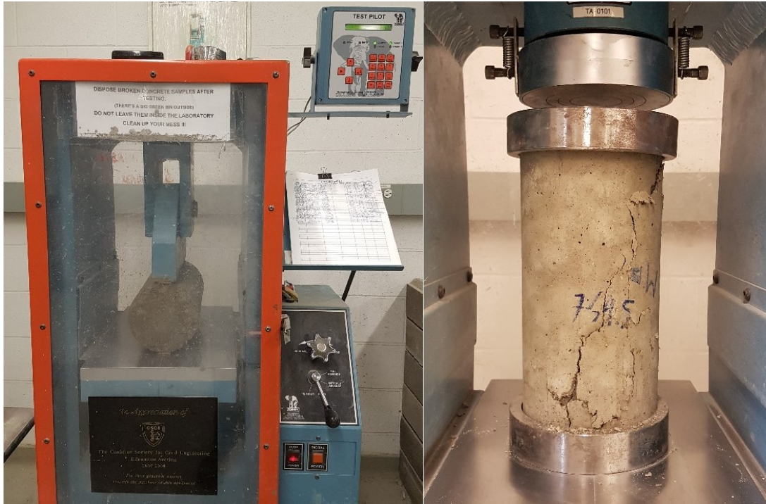
Figure 3.3. Load frame on UTS test setup and UCS test setup
