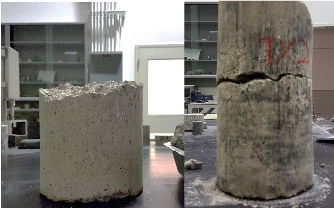
Figure 5.8. Mode of failure of CRF under triaxial test
