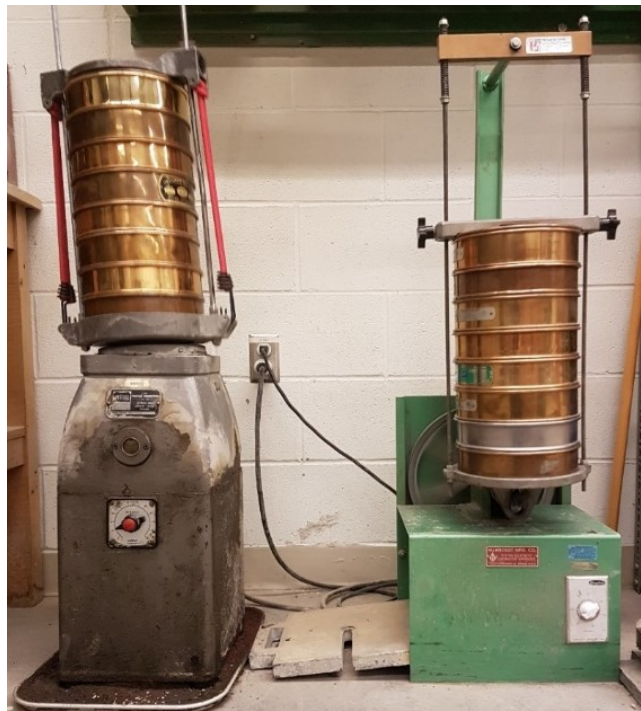
Figure 2.1. Sieve shakers and the set of standard sieve frames
