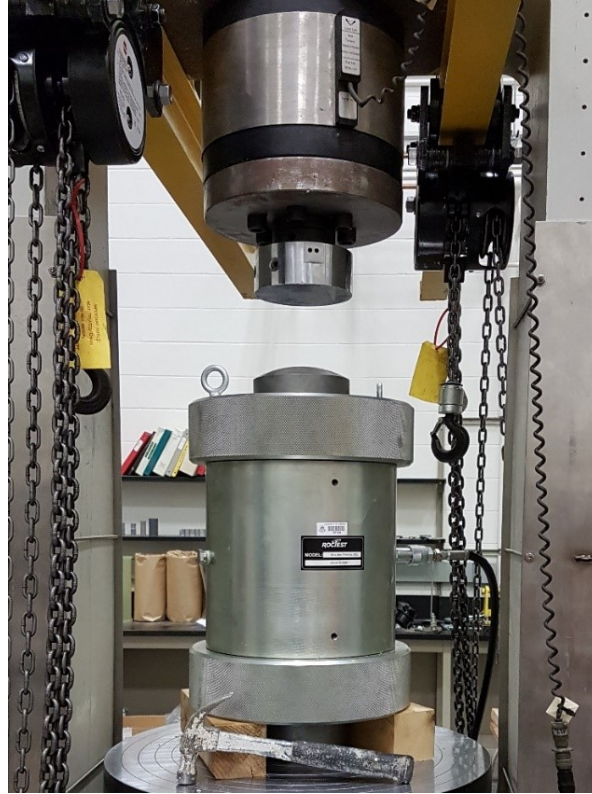
Figure 5.3. 154.2 mm Diameter Hoek triaxial cell and 1,000 ton capacity loading frame INSTRON
