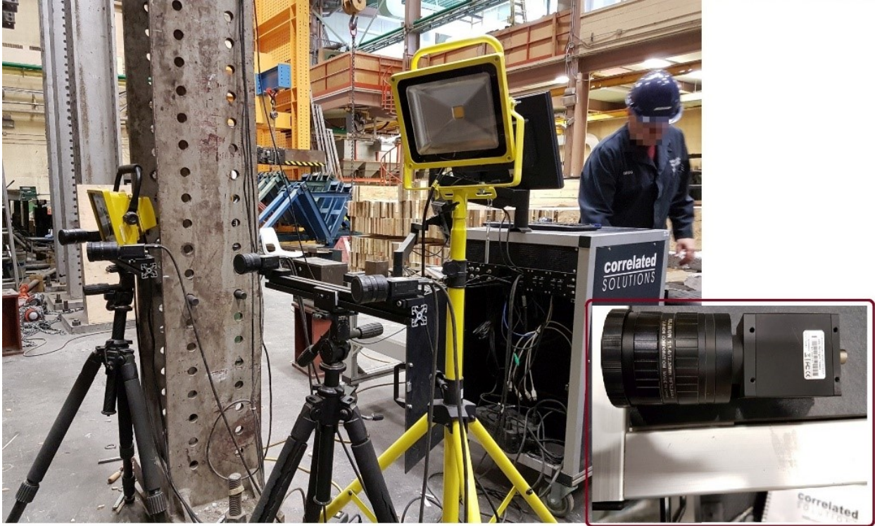
Figure 4.4b. Detailed setup of 3D-DIC instruments, camera, and lens
