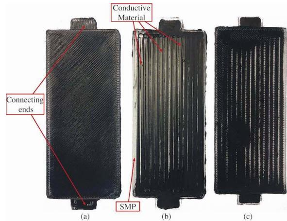
Figure 6.2: a) Sample with an entire layer in between representing 30 *wt.*% content of Graphene/PLA b) Sample showing the surface of printed Graphene/PLA layer with 20 *wt.*% embedded Graphene/PLA and c) Sample showing the embedded printed Graphene/PLA layer of 20 *wt.*% inside the SMP.
