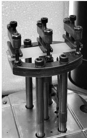
Figure 5.5: Picture of a double cantilever mode DMA set-up
