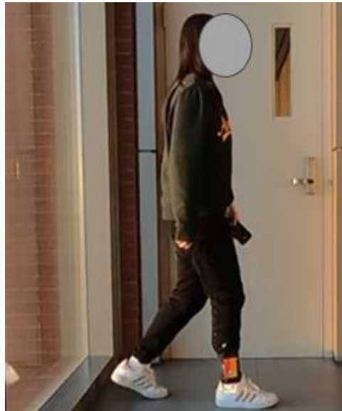
Figure 3.12. Immobilization of smartphone for GRF acceleration estimation.
