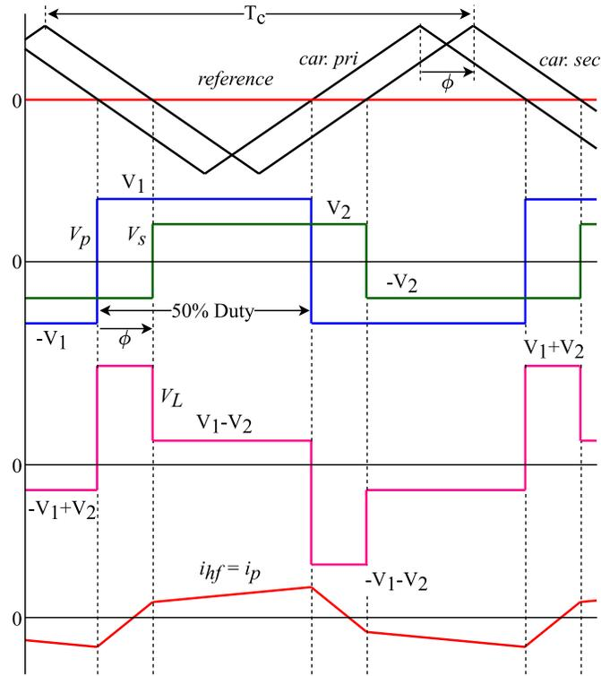
Fig. 3. 2. Switching waveforms of the DAB converter.
