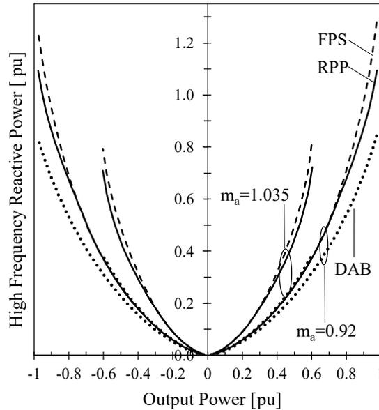
Fig. 3. 37. Simulated high frequency Var plotted against output power. Results per-unitized with  $4.3kW$ .
