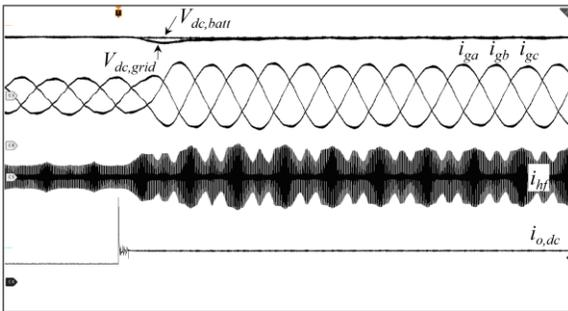
Fig. 5. 20. Experimental transients load change 83 - 40 $\Omega$ .  $V_{LL} = 104V$ ;  $V_{dc} = 180V$ . Scope settings: time 10ms/div;  $i_{g,abc}$ ,  $i_{hf}$  10A/div;  $i_{out,dc}$  5A/div;  $V_{dc,batt}$ ,  $V_{dc,grid}$  50V/div.
