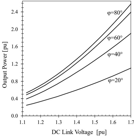
Fig. 3. 40. Simulated output power change with dc link voltage.  $V_{LL} = 208 \text{ V}$ ,  $P_{base} = 5 \text{ kW}$ ,  $V_{base} = 208 \cdot \sqrt{2}$ .
