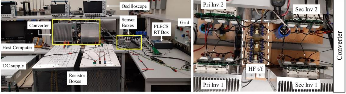
Fig. 5. 1. The experimental setup.
