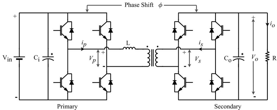
Fig. 2. 3. Phase-shifted dc-dc DAB converter.
