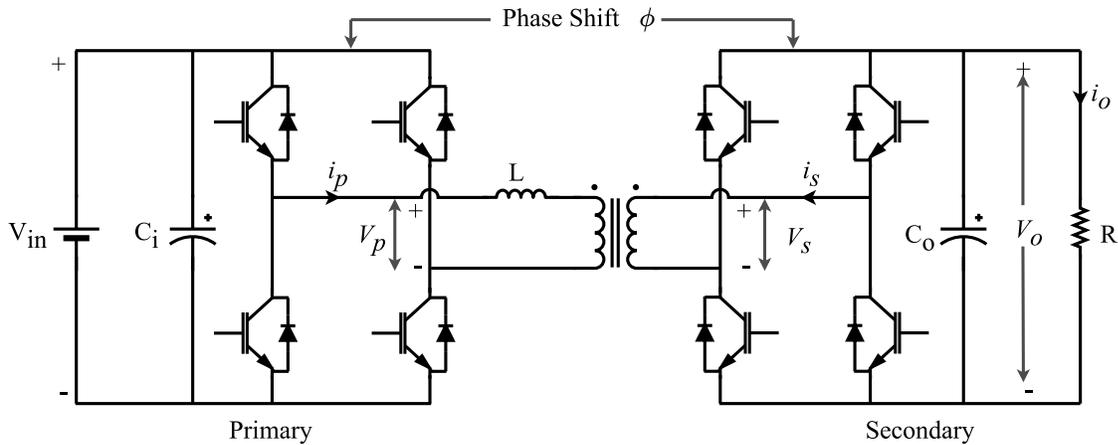
Fig. 1. 2. Single phase dual active bridge converter.
