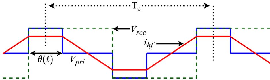
Fig. 3. 22. High frequency pwm waveforms of square-wave pulse position modulation.
