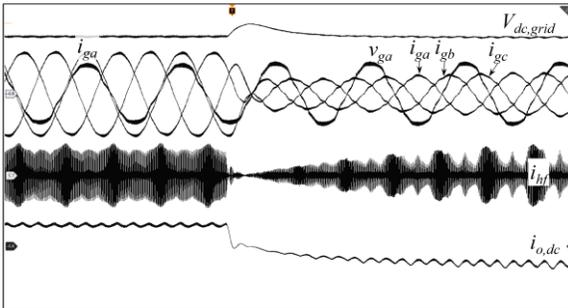
Fig. 5. 22. Experimental power reversal  $P_{out}$  1.6 to -1.6kW.  $V_{LL} = 124V$ ;  $V_{dc} = 230V$ . Scope settings: time 10ms/div;  $i_{g,abc}$ ,  $i_{hf}$ ,  $i_{out,dc}$  10A/div;  $V_{dc,grid}$  50V/div;  $V_{ga}$  100V/div.
