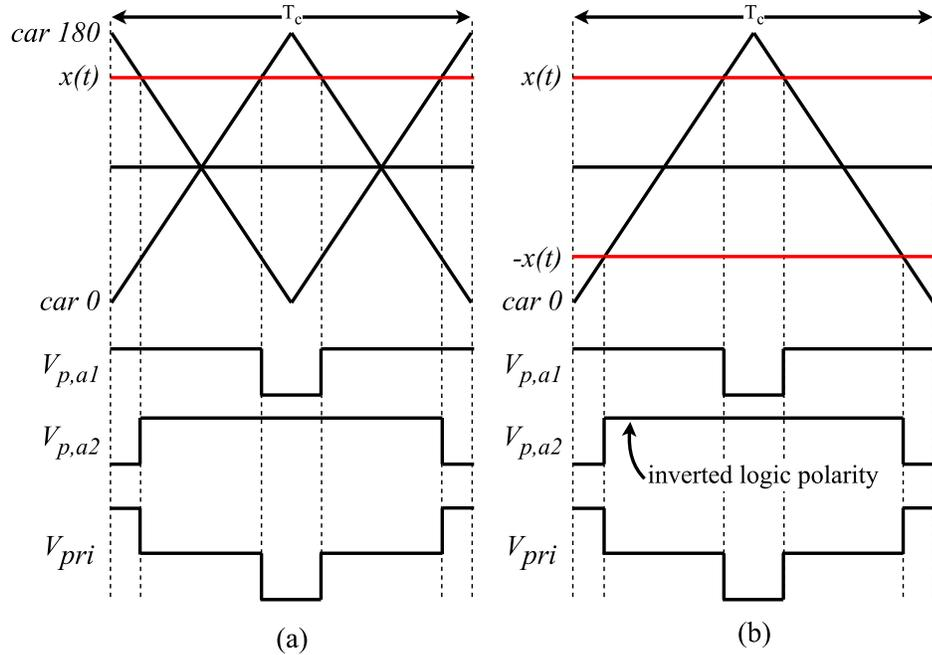
Fig. 3. 15. Single carrier pwm operation. (a) dual carrier operation with  $0^\circ/180^\circ$  carriers, (b) single carrier operation with only  $0^\circ$ . The pwm logic for the negative reference ( $-x(t)$ ) is inverter in the single carrier pwm method.
