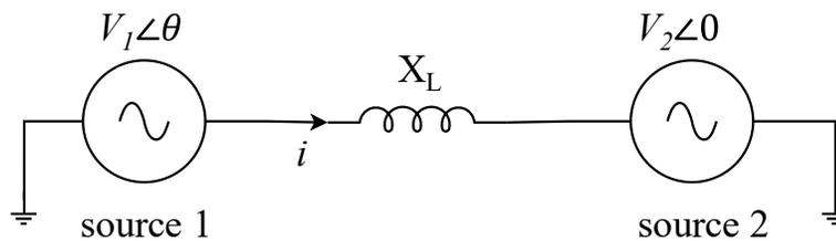
Fig. 3. 7. The active power flows in the direction from higher voltage angle to the lower voltage angle through the impedance  $X_L$ .
