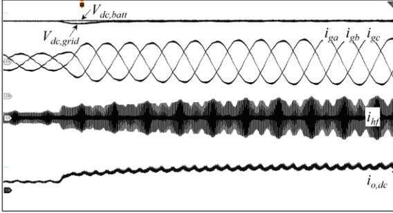
Fig. 5. 18. Experimental transient  $i_{out,dc}$  2A - 5.8A.  $V_{LL} = 104V$ ;  $V_{dc} = 180V$ . Scope settings: time 10ms/div;  $i_{g,abc}$ ,  $i_{hf}$  10A/div;  $i_{out,dc}$  5A/div;  $V_{dc,batt}$ ,  $V_{dc,grid}$  50V/div.
