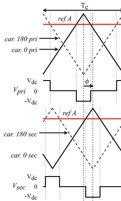
Fig. 1. 7. Phase shifting the secondary carriers only by angle  $\phi$  to implement the same phase shift in the voltage waveforms.
