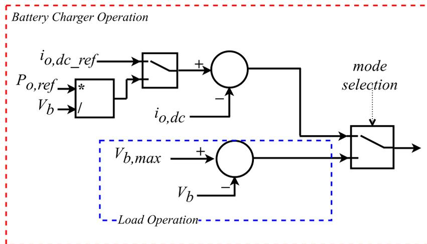
Fig. 4. 10. Output modes of operation.
