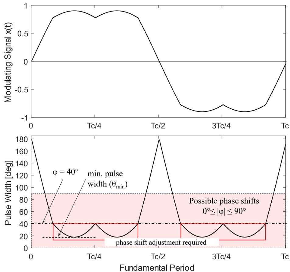
Fig. 3. 17. Change in pulse width with grid fundamental period.
