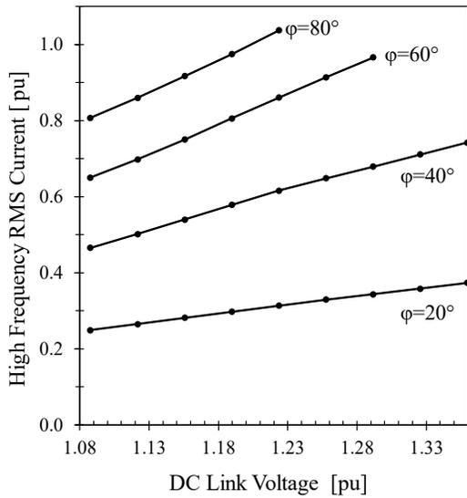
Fig. 5. 7. Experimental high frequency rms current change with dc link voltage.  $V_{base} = 104\sqrt{2}$ ;  $P_{base} = 1\text{kW}$ .
