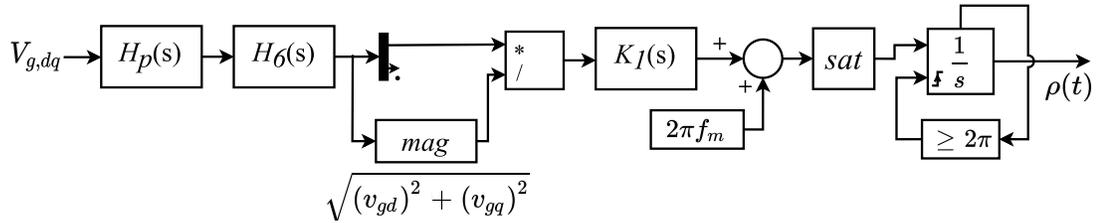
Fig. 4. 11. Schematic of the designed PLL controller.
