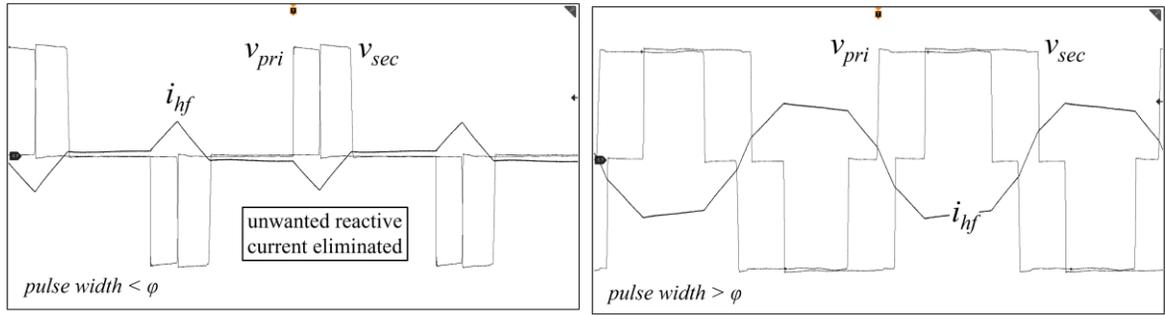
Fig. 5. 11. Experimental RPP operation for pulse width  $< \phi$ .  $V_{LL} = 104$ ;  $V_{dc} = 180V$ ;  $\phi = 60^\circ$ .
