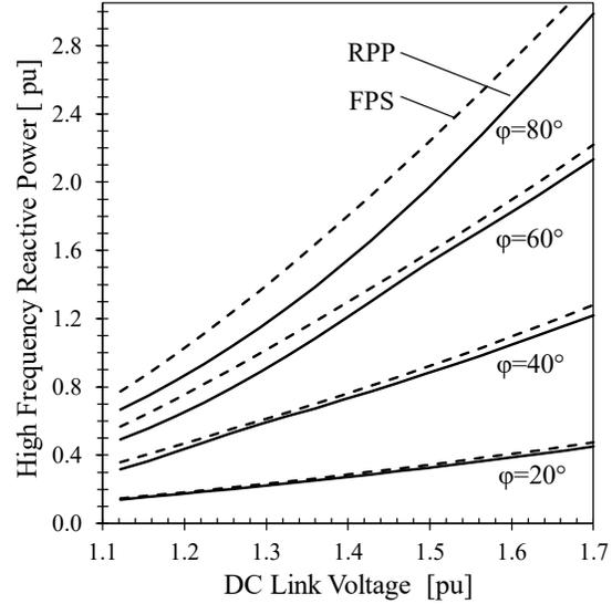
Fig. 3. 39. Simulated high frequency Var change against dc link voltage.  $V_{LL} = 208V$ ,  $P_{base} = 5kW$ ,  $V_{base} = 208*\sqrt{2}$ .
