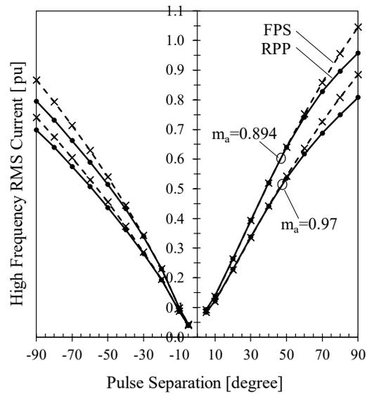
Fig. 5. 3. Experimental high frequency rms current against pulse separation. VLL = 104V; Vdc = 175V (0.97 $m_a$ ), 190V (0.894 $m_a$ ); Pbase = 1.3kW.
