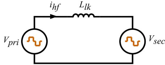
Fig. 1. 8. The power transfer model of the converter topology can be simplified into a transformer equivalent as shown.  $V_{pri}$ ,  $V_{sec}$ : high frequency pulse voltages at the primary and the secondary of the transformer,  $L_{lk}$ : equivalent series inductance through which the power is being transferred,  $i_{hf}$ : high frequency current.
