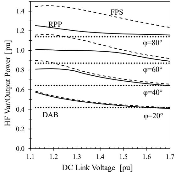
Fig. 3. 41. Simulated HF Var to output power ratio with dc link voltage.  $V_{LL} = 208 \text{ V}$ ,  $P_{base} = 5 \text{ kW}$ ,  $V_{base} = 208 \cdot \sqrt{2}$ .
