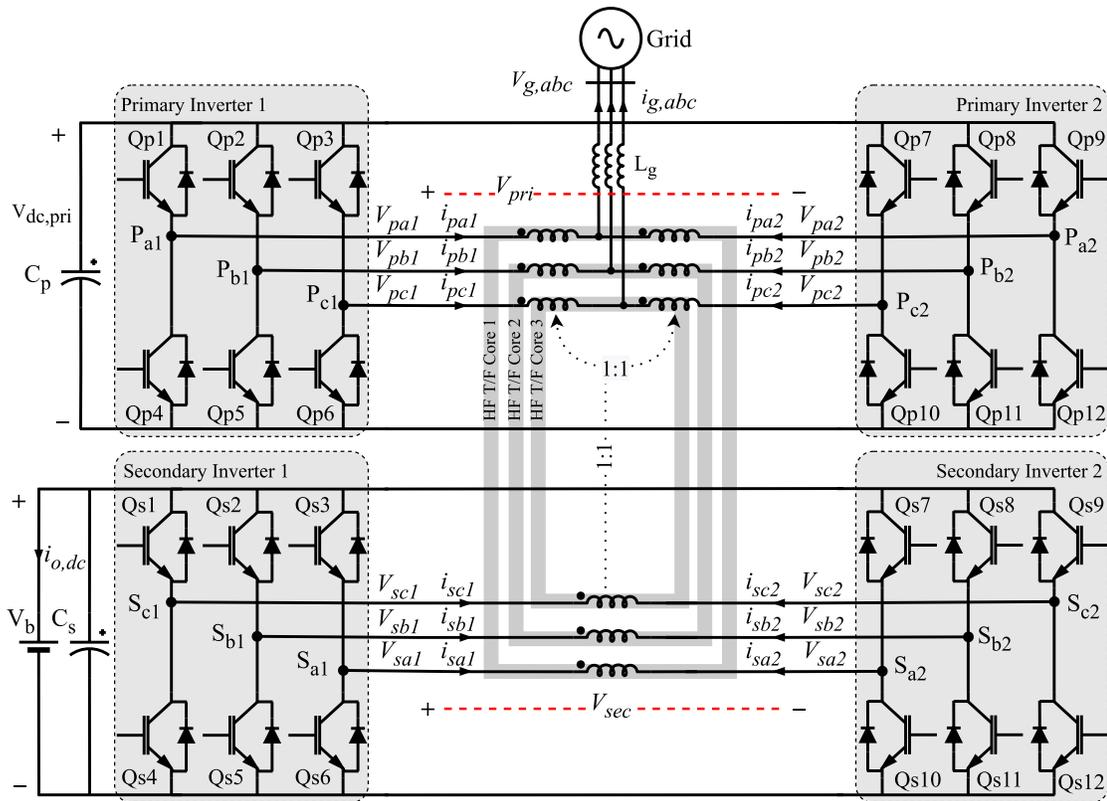
Fig. 1. 4. Selected converter topology – Three phase bidirectional single stage isolated ac-dc converter.
