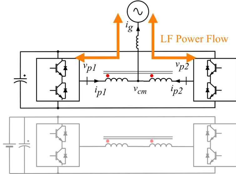
Fig. 3. 8. The common mode circuit of the converter for the phase A. The circuit is the same for phases B, C.
