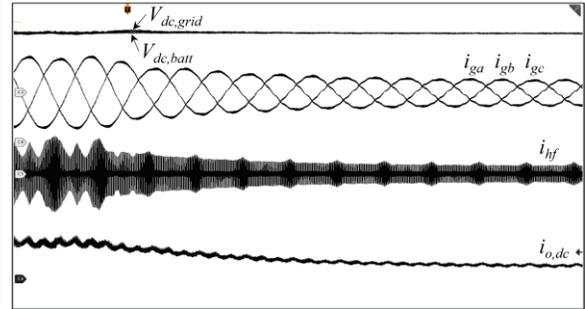
Fig. 5. 19. Transients  $i_{out,dc}$  5.8A - 2A.  $V_{LL} = 104V$ ;  $V_{dc} = 180V$ . Scope settings: time 10ms/div;  $i_{g,abc}$ ,  $i_{hf}$  10A/div;  $i_{out,dc}$  5A/div;  $V_{dc,batt}$ ,  $V_{dc,grid}$  50V/div.
