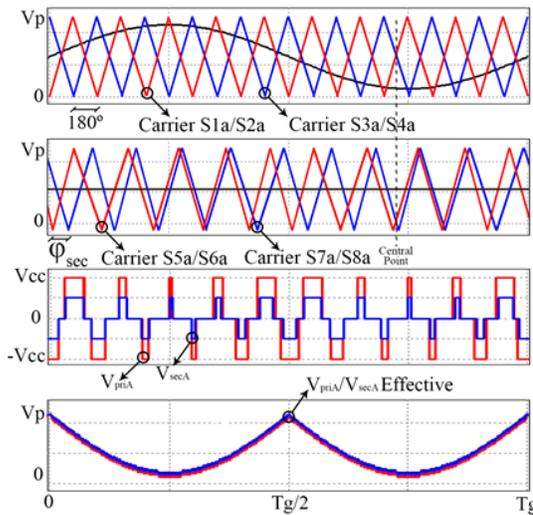
Fig. 1. 6. Illustration of main and secondary phase shift of [2]. A secondary phase shift  $\phi_{sec}$  is implemented on the secondary carriers in order to align the primary and secondary voltages. Source [2]
