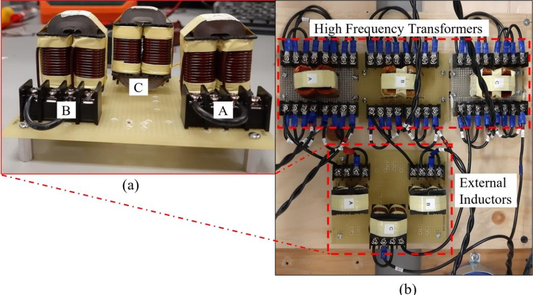
Fig. 3. 24. External inductors used with high frequency transformers. Each inductor is 100uH, 9.4A rms rated.
