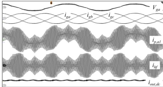
Fig. 5. 17. Experimental 80 degrees.  $i_{g,abc}$  20A/div;  $i_{pa1}$ ,  $i_{hf}$  10A/div;  $i_{out,dc}$  10A/div; time 4ms/div;  $V_{ga}$  200V/div.  $V_{LL} = 104V$ ;  $V_{dc} = 180V$ .
