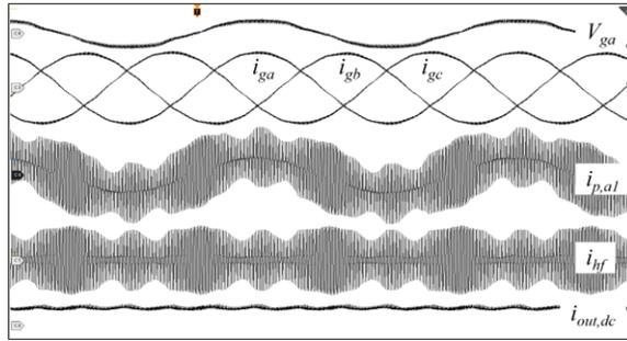
Fig. 5. 16. Experimental 60 degrees.  $i_{g,abc}$  10A/div;  $i_{pa1}$ ,  $i_{hf}$  10A/div;  $i_{out,dc}$  10A/div; time 4ms/div;  $V_{ga}$  200V/div.  $V_{LL} = 104V$ ;  $V_{dc} = 180V$ .
