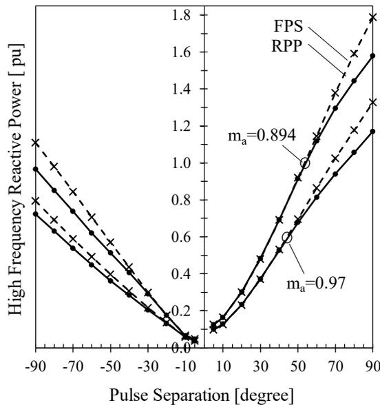
Fig. 5. 4. Experimental high frequency reactive power change with pulse separation. VLL = 104V; Vdc = 175V (0.97 $m_a$ ), 190V (0.894 $m_a$ ); Pbase = 1.3kW.
