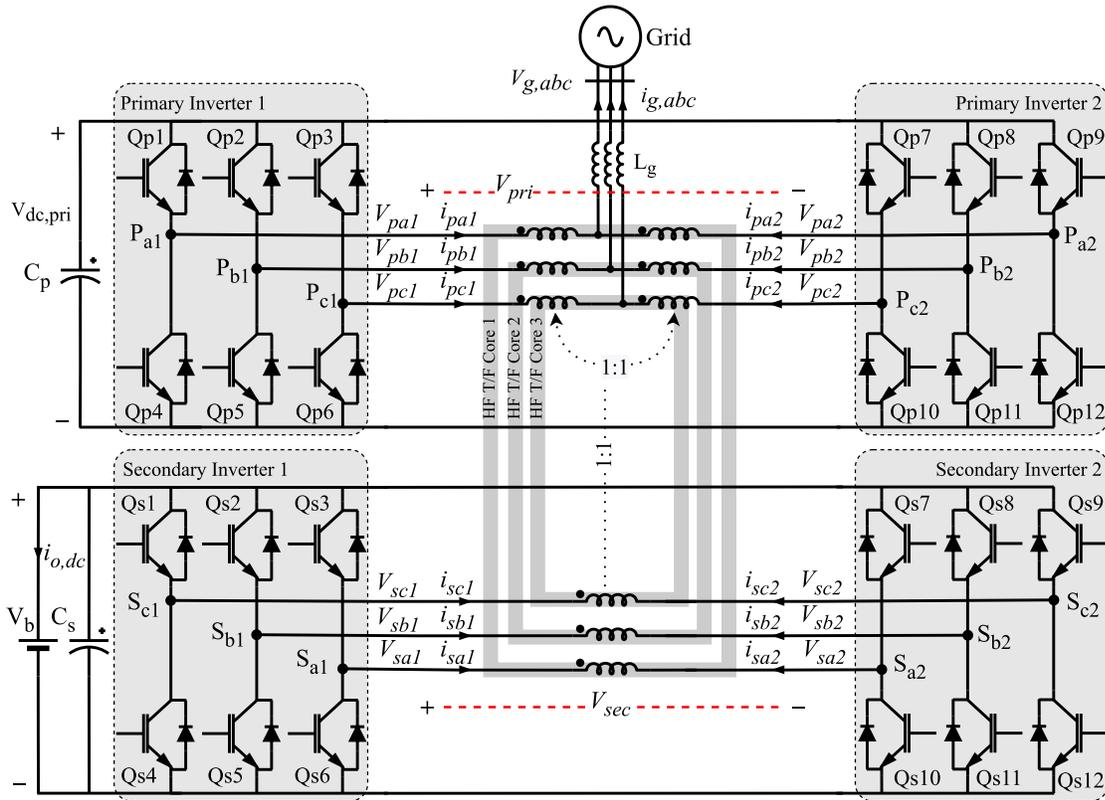
Fig. 2. 1 Converter topology discussed in the thesis. Each phase can be considered as a single-phase DAB (Fig. 2. 3) transferring power between primary and secondary by phase shifting.
