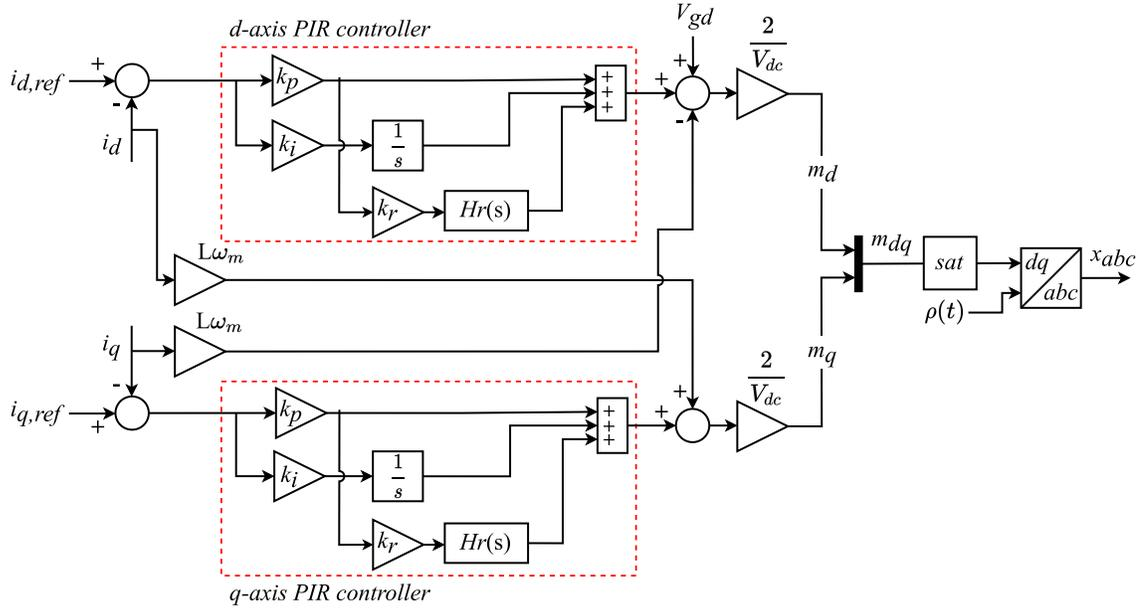
Fig. 4. 5. Schematic of the grid current controller in the dq-axis.
