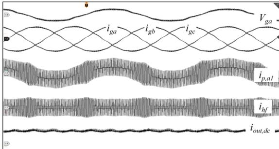
Fig. 5. 15. Experimental 40 degrees.  $i_{g,abc}$  10A/div;  $i_{pa1}$ ,  $i_{hf}$  10A/div;  $i_{out,dc}$  5A/div; time 4ms/div;  $V_{ga}$  200V/div.  $V_{LL} = 104V$ ;  $V_{dc} = 180V$ .
