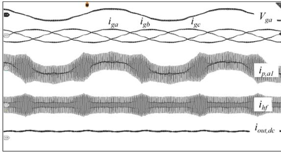
Fig. 5. 14. Experimental 20 degrees.  $i_{g,abc}$  10A/div;  $i_{pa1}$ ,  $i_{hf}$  5A/div;  $i_{out,dc}$  5A/div; time 4ms/div;  $V_{ga}$  200V/div.  $V_{LL} = 104V$ ;  $V_{dc} = 180V$ .
