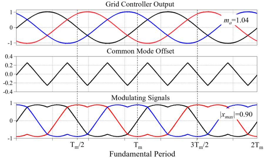
Fig. 4. 1. Space vector modulation by the addition of common mode offset. Fundamental modulation index ( $m_a$ ) = 1.04. Maximum value of modulating signals with CMO ( $x_{max}$ ) = 0.9. The peak of the reference signals is decreased by a factor of 1.15 due to SVPWM.
