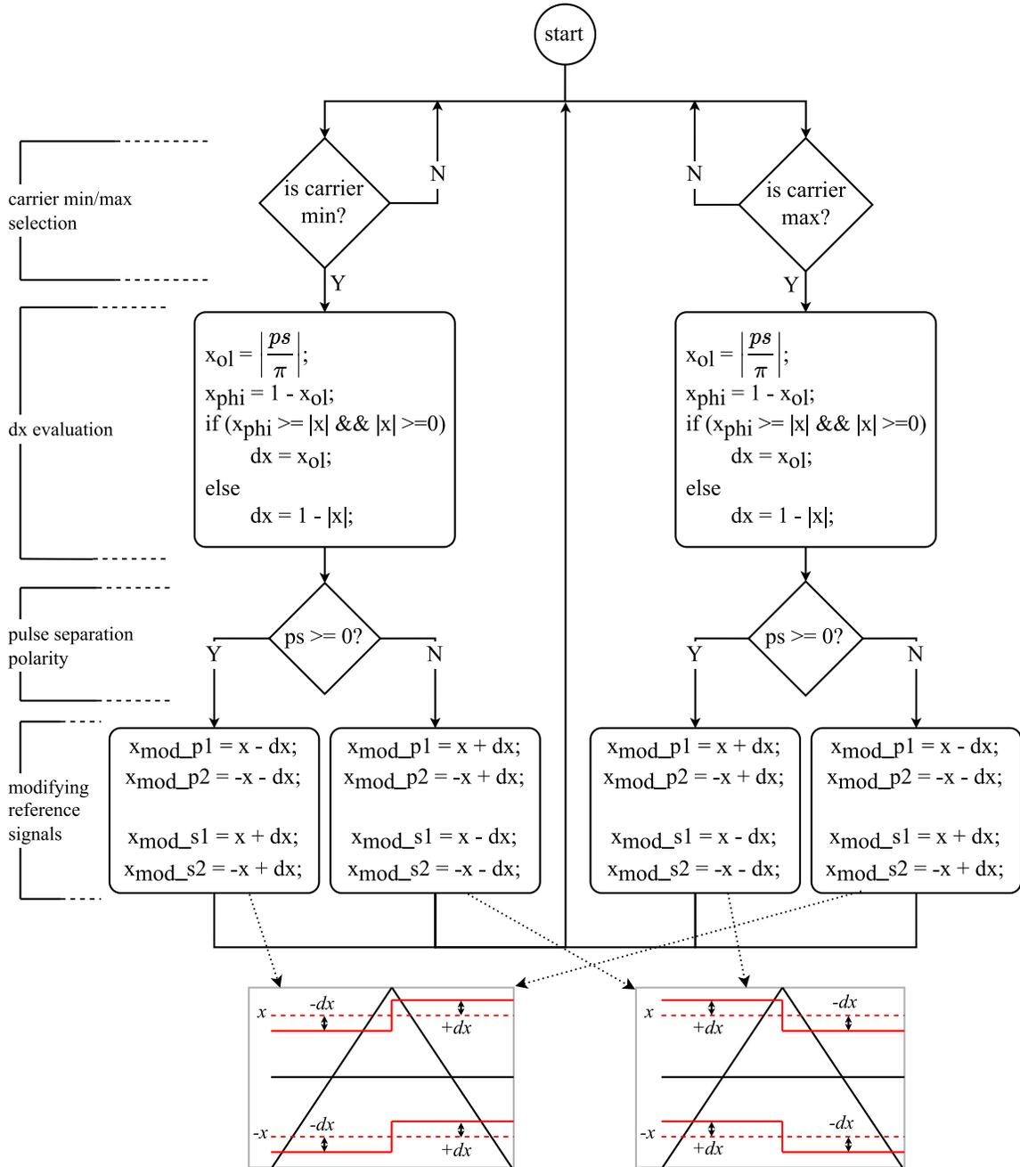
Fig. 4. 2. Reference modification algorithm.
