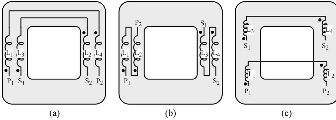
Fig. 3. 27. Physical winding arrangements corresponding to Fig. 3. 25, Fig. 3. 26.
