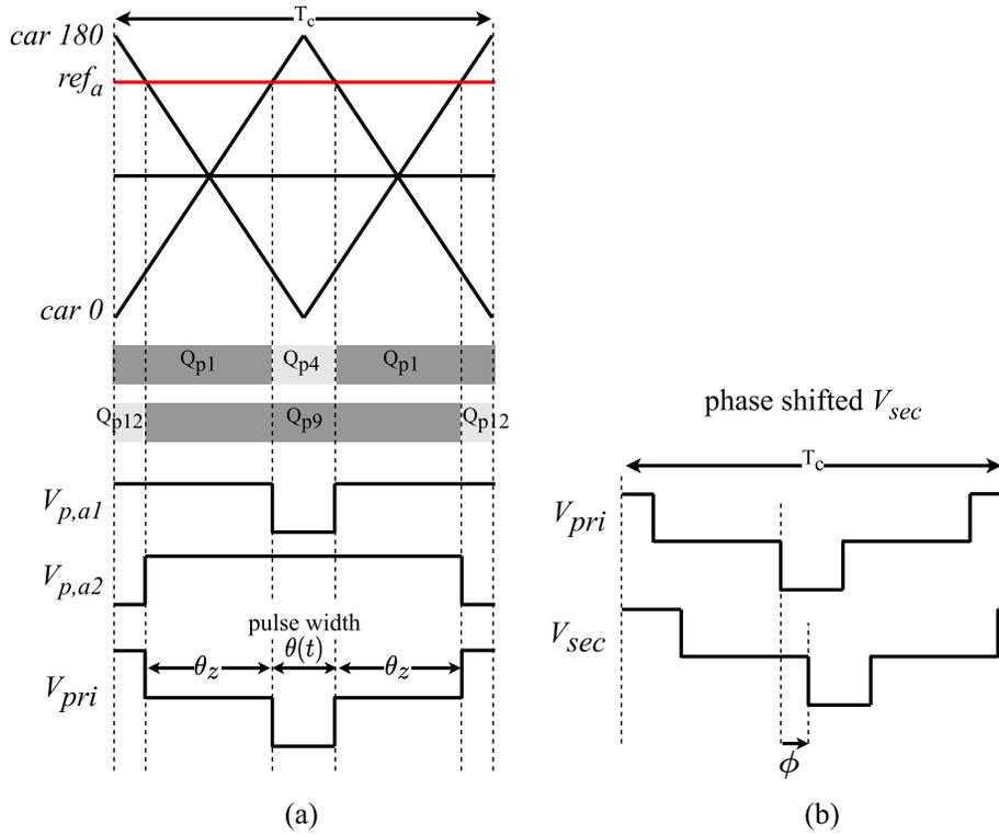
Fig. 3. 5. Switching waveforms and phase shift of primary phase A (a) primary side switching pwm waveforms, (b) phase shift  $\phi$  implemented on the secondary voltage  $V_{sec}$ .
