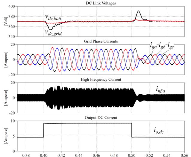
Fig. 3. 44. Load change.  $80\text{-}40\text{-}80\ \Omega$ .  $V_{LL} = 208\text{V}$ ,  $V_{dc} = 370\text{V}$ .
