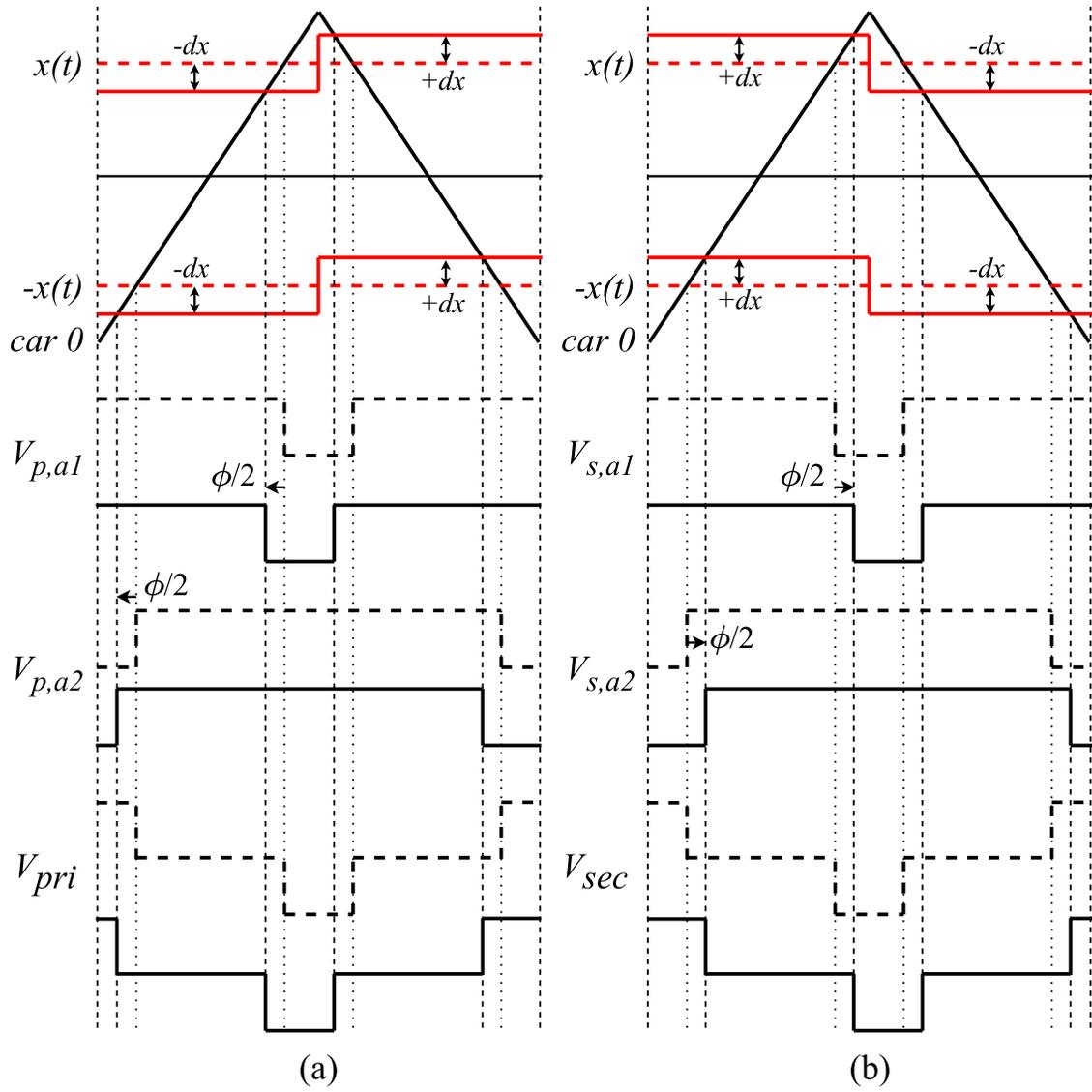
Fig. 3. 19. Pulse separation achieved through reference modification (a) modification for the primary side, (b) modification for the secondary side. The dashed signals represent waveforms of original unmodified reference, whereas the solid signals represent phase shifted waveforms of modified reference.
