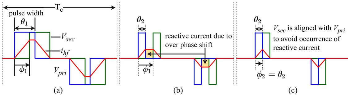
Fig. 3. 14. Concept illustration of the RPP method.
