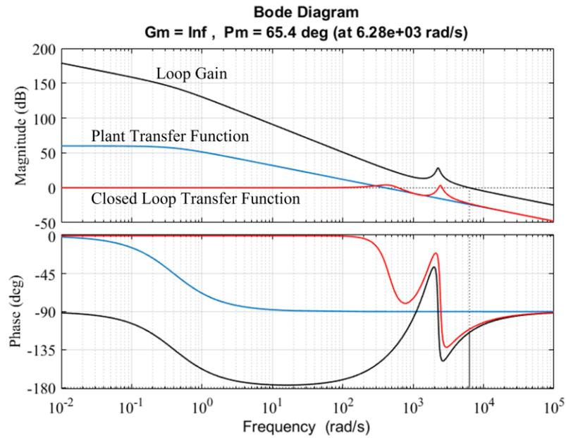
Fig. 4. 6. Bode diagram of the current controller.
