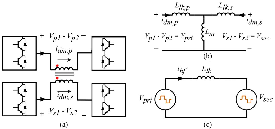
Fig. 3. 10. Simplification of the DM circuit into an equivalent transformer model.
