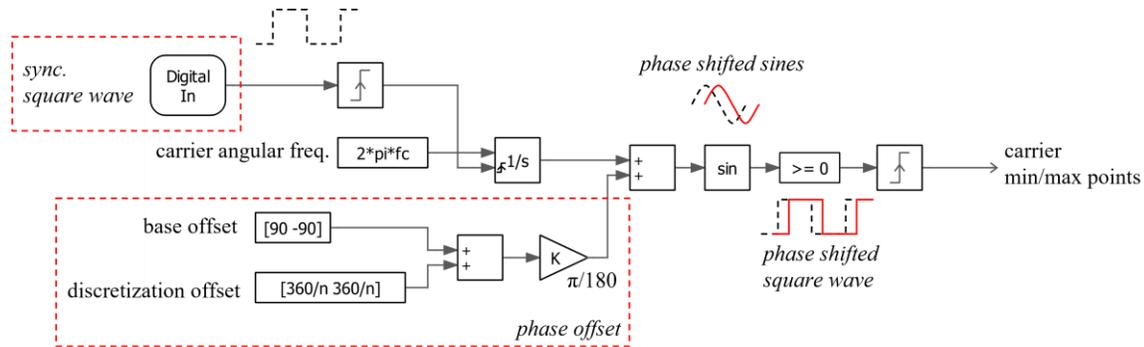
Fig. 4. 13. Synchronizing the simulation with carrier minimum and maximum.
