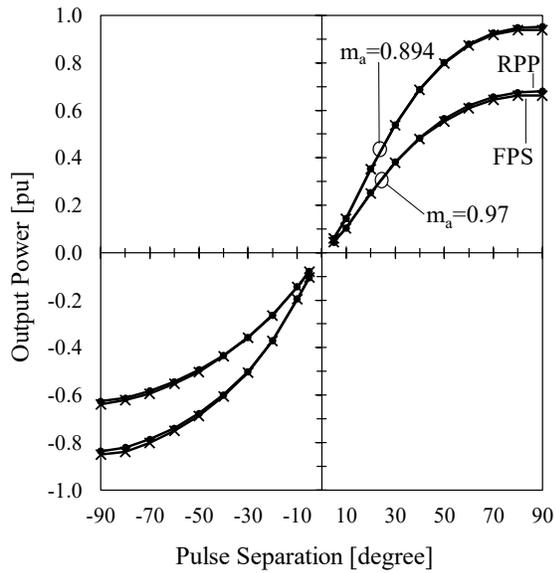
Fig. 5. 2. Experimental output power change against pulse separation. VLL = 104V; Vdc = 175V (0.97 $m_a$ ), 190V (0.894 $m_a$ ); Pbase = 1.3kW.
