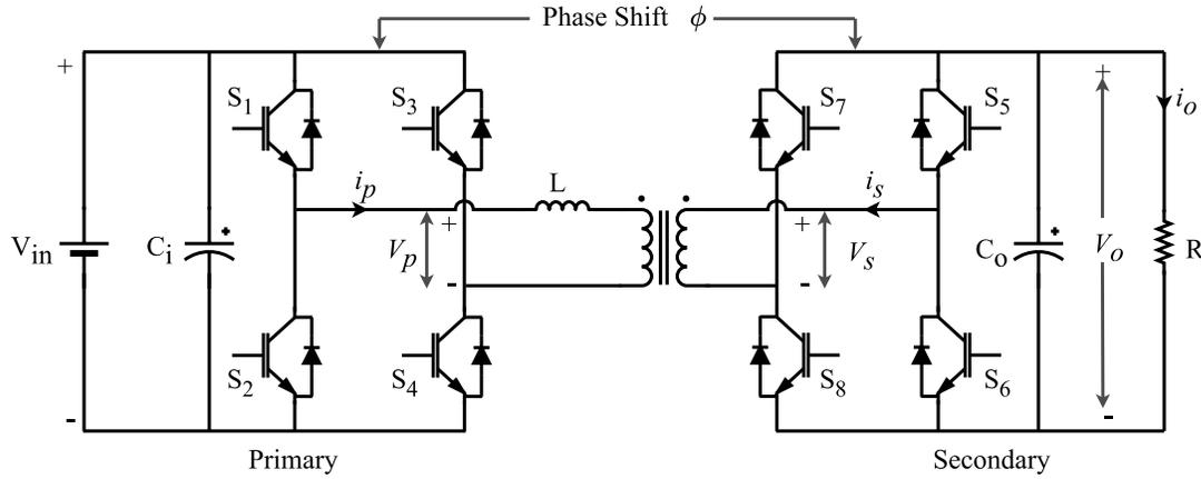
Fig. 3. 1. Circuit schematic of a DAB dc-dc converter.
