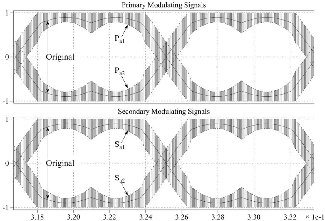
Fig. 4. 3. Final modulating signals generated by the algorithm for the phase A for  $m_a=0.9$ .  $P_{a1}$ ,  $P_{a2}$  are the modulating signals for the primary respective inverter legs while  $S_{a1}$ ,  $S_{a2}$  are for the secondary.
