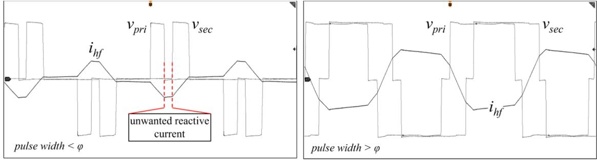
Fig. 5. 10. Experimental FPS operation for pulse width  $< \phi$ .  $V_{LL} = 104$ ;  $V_{dc} = 180V$ ;  $\phi = 60^\circ$ .
