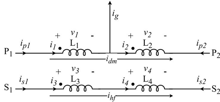
Fig. 3. 28. Winding placement for the arrangement (b).
