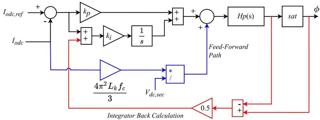
Fig. 4. 9. Control schematic of the pulse separation controller.
