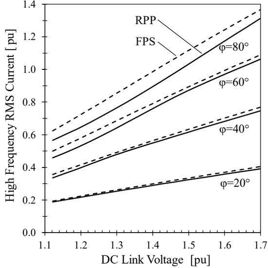
Fig. 3. 38. Simulated high frequency rms current change against dc link voltage.  $V_{LL} = 208V$ ,  $P_{base} = 5kW$ ,  $V_{base} = 208*\sqrt{2}$ .
