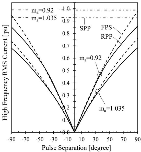
Fig. 3. 33. Simulated high frequency rms current change with pulse separation.  $V_{dc} = 329V$  ( $1.035m_a$ ),  $370V$  ( $0.92m_a$ ).  $P_{base} = 4.45kW$ .
