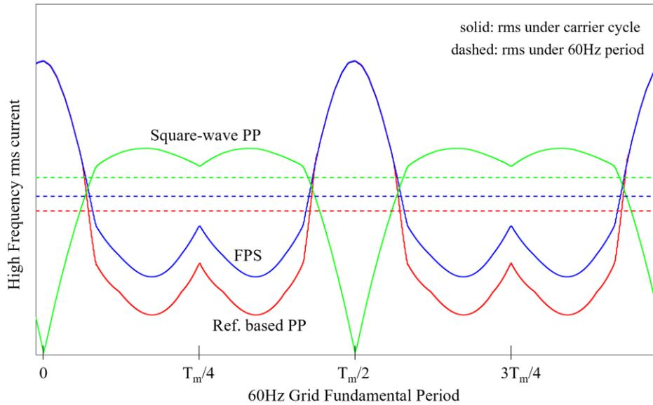
Fig. 3. 32. Simulated variation of rms of the high frequency current under a 60Hz grid fundamental period plotted for a constant power level.
