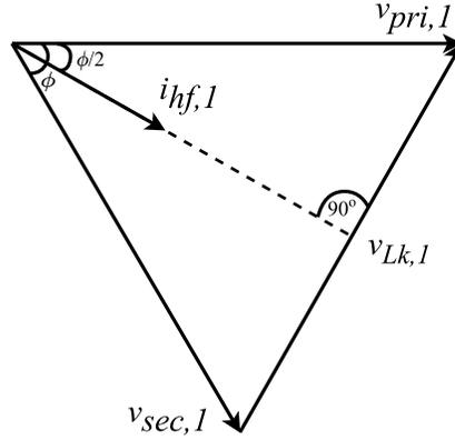
Fig. 3. 31. High frequency voltage current phasor diagram.
