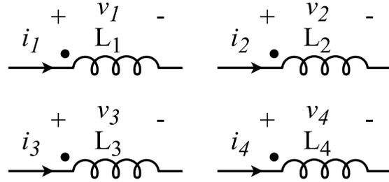
Fig. 3. 26. Notation of current and voltage of each element of the winding matrix.
