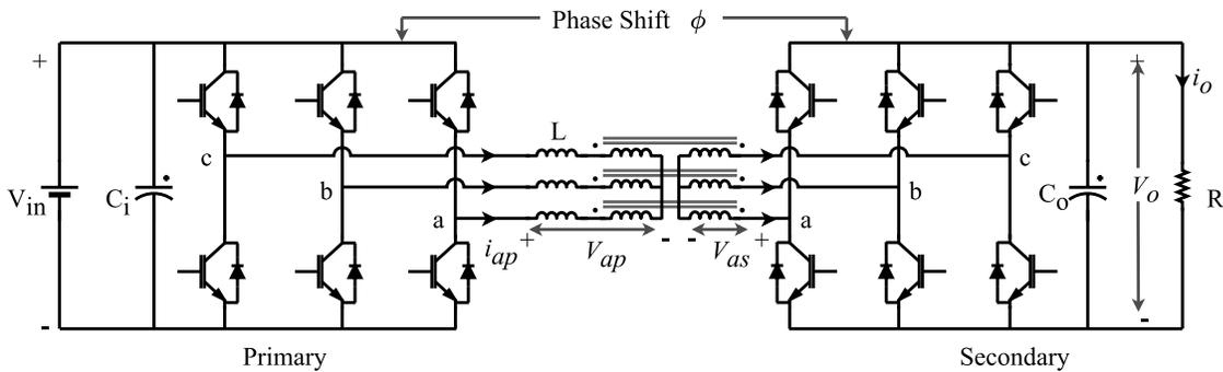
Fig. 1. 3. Three phase dual active bridge converter.
