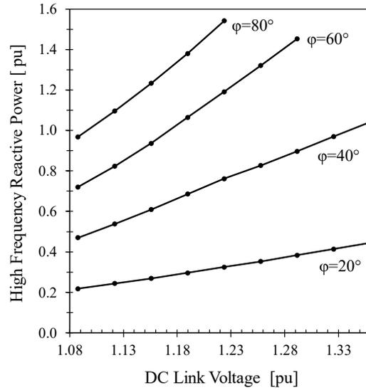
Fig. 5. 8. Experimental high frequency reactive power change with dc link voltage.  $V_{base} = 104\sqrt{2}$ ;  $P_{base} = 1\text{kW}$ .
