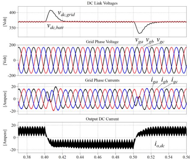
Fig. 3. 42. Power reversal  $\pm 4\text{kW}$ .  $V_{LL} = 208\text{V}$ ,  $V_{dc} = 370\text{V}$ .
