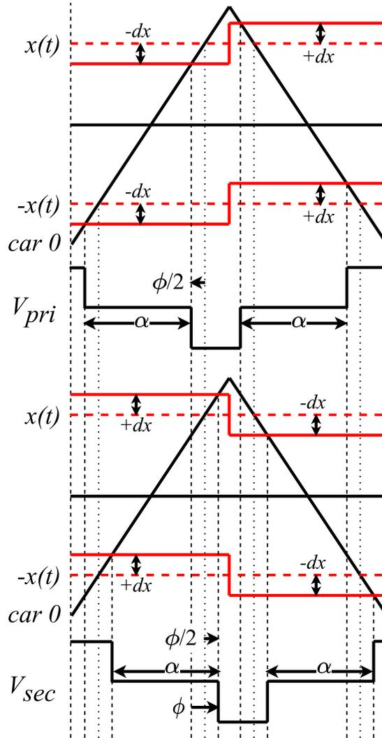
Fig. 3. 20. Total pulse separation is achieved by implementing half the separation on each side in opposite phase angle polarity.
