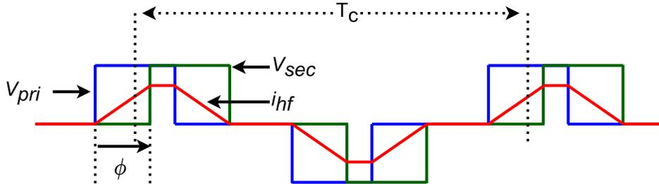
Fig. 1. 9. Characteristic waveforms of the FPS method.
