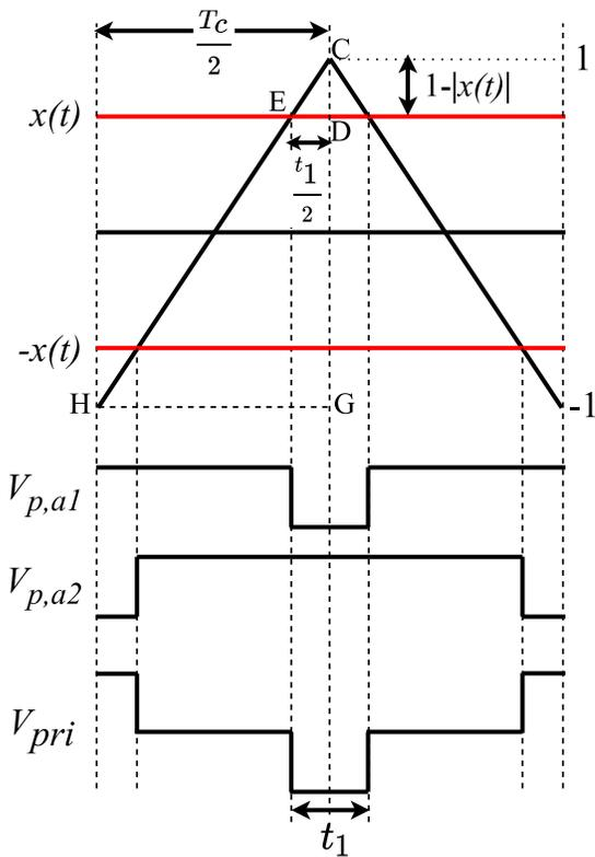
Fig. 3. 16. Pulse width and reference relationship.
