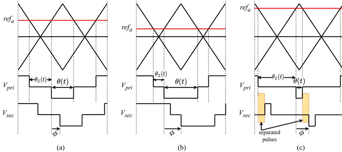
Fig. 3. 6. The three operating regions (a)  $\varphi < \theta$ ;  $\varphi < \theta_z$ , (b)  $\varphi < \theta$ ;  $\varphi > \theta_z$ , (c)  $\varphi > \theta$ . Phase shift in (a) and (b) is less than the pulse width while in (c) phase shift is larger than pulse width.
