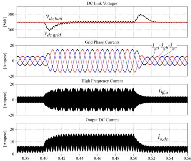
Fig. 3. 43. Output current step change  $4\text{-}10\text{-}4\ \text{A}$ .  $V_{LL} = 208\text{V}$ ,  $V_{dc} = 370\text{V}$ .
