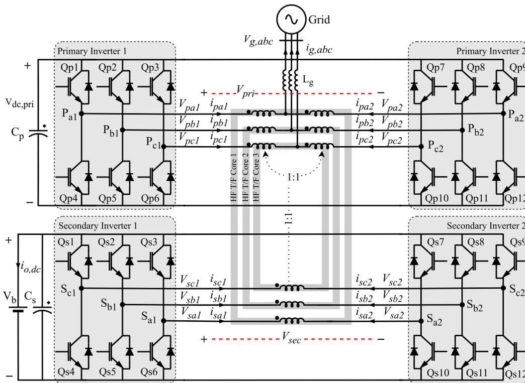
Fig. 3. 3. Schematic of the converter.
