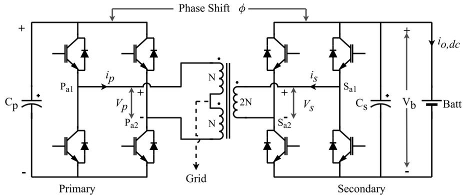
Fig. 2. 2. Single-phase circuit of the converter described in Fig. 2. 1 for the high frequency power transfer. The power transfer inductance can be an externally placed inductor or the interlimb leakage inductance of the high frequency isolation transformer.
