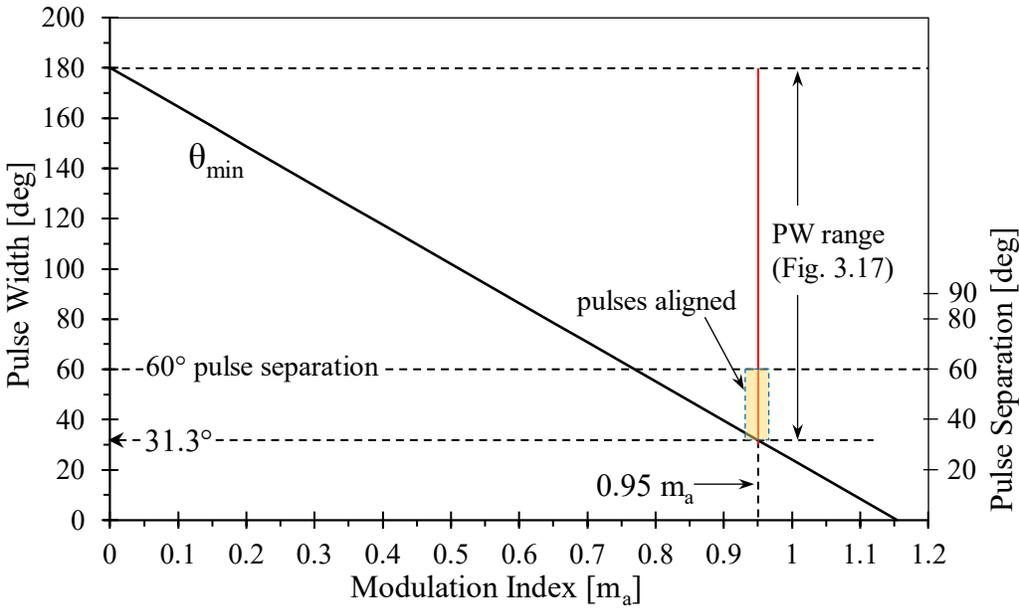
Fig. 3. 18. Pulse width variation with the modulation index.
