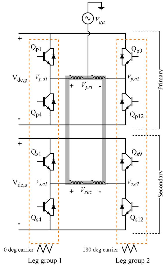
Fig. 3. 4. Phase A equivalent circuit.
