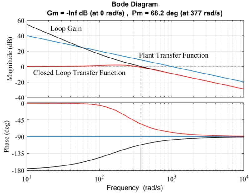
Fig. 4. 8. Bode diagram of the Voltage controller.
