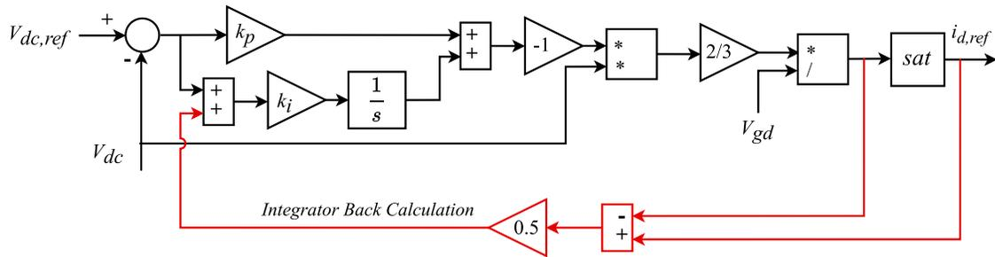
Fig. 4. 7. Control schematic of the grid dc link voltage controller.
