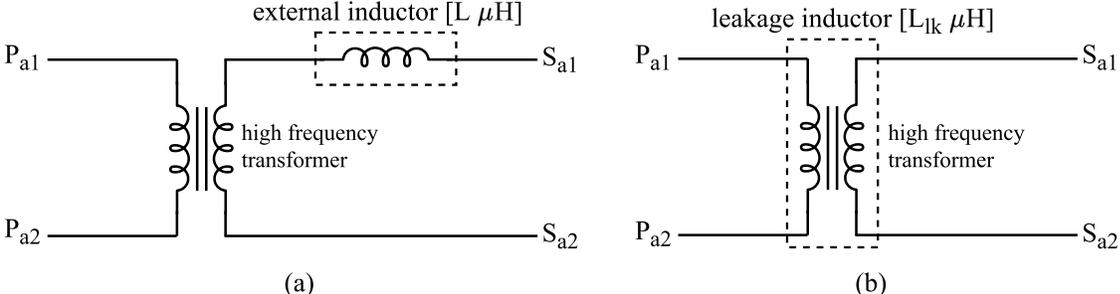
Fig. 3. 23. Power transfer inductance placement (a) as an external series inductor, (b) integrating with the transformer to form an interlimb leakage inductance.
