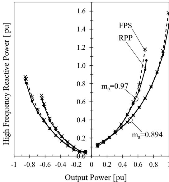
Fig. 5. 5. Experimental high frequency reactive power change with output power.  $V_{LL} = 104V$ ;  $V_{dc} = 175V (0.97m_a)$ ,  $190V (0.894m_a)$ ;  $P_{base} = 1.3kW$ .
