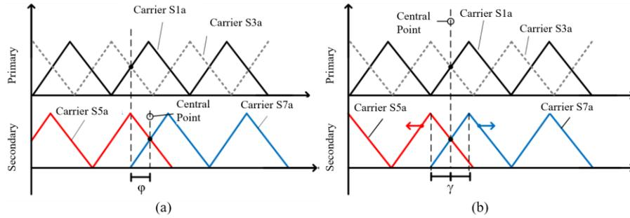
Fig. 1. 5. Carrier phase shift strategy presented in [2]. (a) Main phase shift  $\phi$  implemented on the secondary carriers, (b) secondary phase shift implemented on the secondary carriers by moving the carriers. Source [2].
