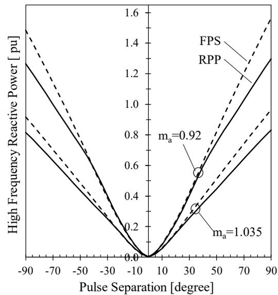
Fig. 3. 34. Simulated high frequency Var variation with pulse separation.  $V_{dc} = 329V$  ( $1.035m_a$ ),  $370V$  ( $0.92m_a$ ).  $P_{base} = 4.45kW$ .
