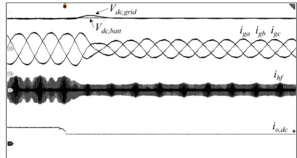
Fig. 5. 21. Experimental transients load change 40 - 83 $\Omega$ .  $V_{LL} = 104V$ ;  $V_{dc} = 180V$ . Scope settings: time 10ms/div;  $i_{g,abc}$ ,  $i_{hf}$  10A/div;  $i_{out,dc}$  5A/div;  $V_{dc,batt}$ ,  $V_{dc,grid}$  50V/div.
