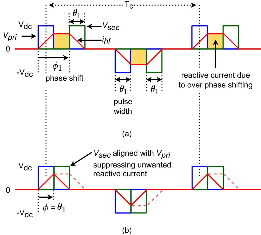
Fig. 1. 10. The concept of pulse alignment when the phase shift is larger than the pulse width.
