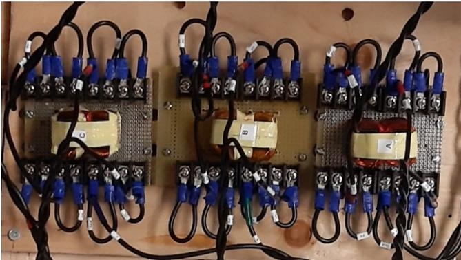
Fig. 3. 30. Integrated leakage inductance wound according to Fig. 3. 25(b)
