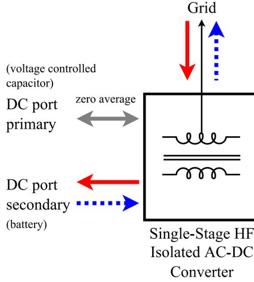
Fig. 3. 11. Power balance of the converter.
