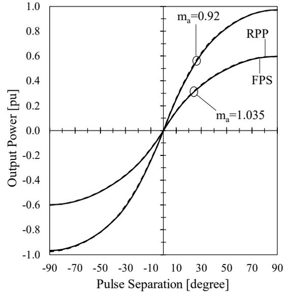
Fig. 3. 36. Simulated output power against pulse separation.  $V_{dc} = 329V$  ( $1.035m_a$ ),  $370V$  ( $0.92m_a$ ).  $P_{base} = 4.45kW$ .
