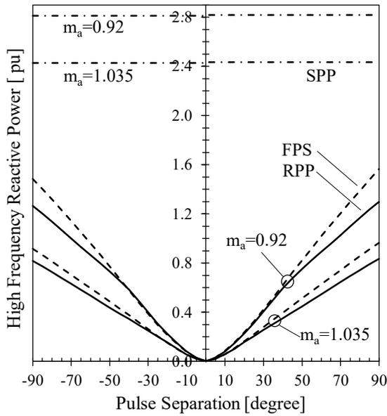
Fig. 3. 35. Simulated high frequency Var change with pulse separation.  $V_{dc} = 329V$  ( $1.035m_a$ ),  $370V$  ( $0.92m_a$ ).  $P_{base} = 4.45kW$ .
