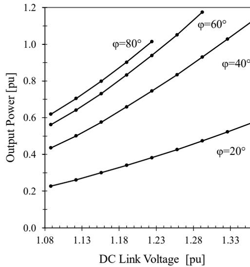
Fig. 5. 9. Experimental output power change with dc link voltage.  $V_{base} = 104\sqrt{2}$ ;  $P_{base} = 1\text{kW}$ .
