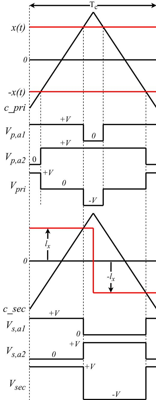
Fig. 3. 21. SPP pwm operation. Secondary reference signal is a square wave with amplitude  $l_x = x$  at carrier minimum and maximum.
