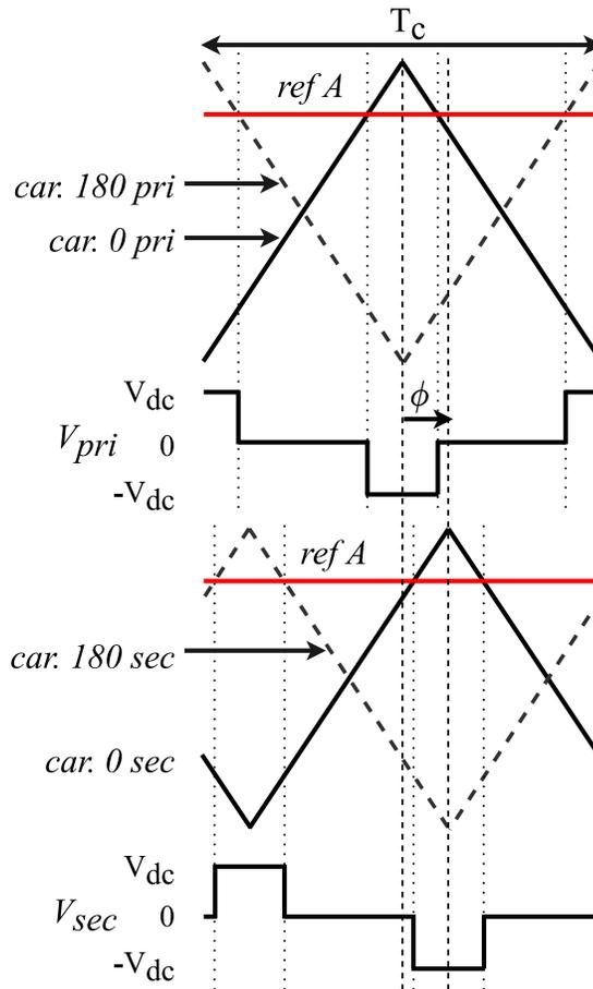
Fig. 3. 13. A typical carrier phase shifted pwm method. both the primary and secondary have the same reference.
