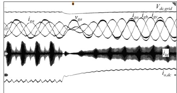
Fig. 5. 23. Experimental power reversal  $P_{out}$  -1.6 to 1.6kW.  $V_{LL} = 124V$ ;  $V_{dc} = 230V$ . Scope settings: time 10ms/div;  $i_{g,abc}$ ,  $i_{hf}$ ,  $i_{out,dc}$  10A/div;  $V_{dc,grid}$  50V/div;  $V_{ga}$  100V/div.
