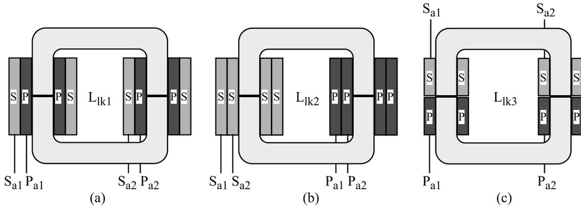
Fig. 3. 25. Different winding arrangements to realize interlimb leakage inductance. The windings ‘S’, ‘P’ represents the secondary and primary windings. Here,  $L_{lik1} < L_{lik3} < L_{lik2}$ .
