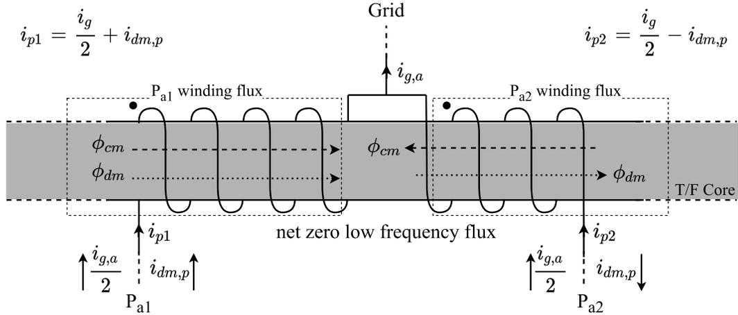
Fig. 3. 12. CM and DM flux inside primary limb of the transformer.
