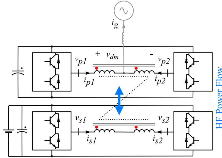
Fig. 3. 9. The differential mode circuit of the converter for the phase A. The circuit is the same for phases B, C.
