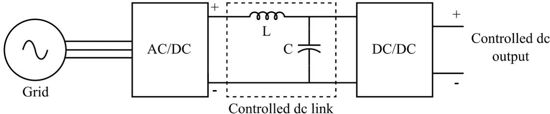
Fig. 1. 1. A generic two stage ac-dc power converter.
