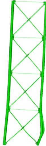
**Figure 2.19: Frame deformed shape at the instant of column buckling (Imanpour et al. 2016a)**
