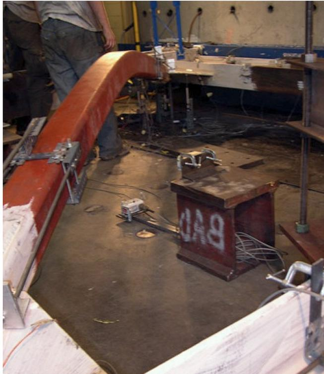
*Figure 2.4: HSS brace out-of-plane buckling (Sabelli et al. 2013)*
