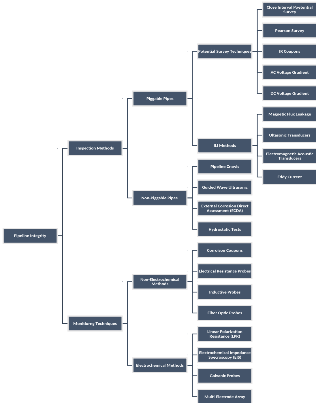
Figure 2.3: Comprehensive Developed Pipeline Integrity Solutions.
