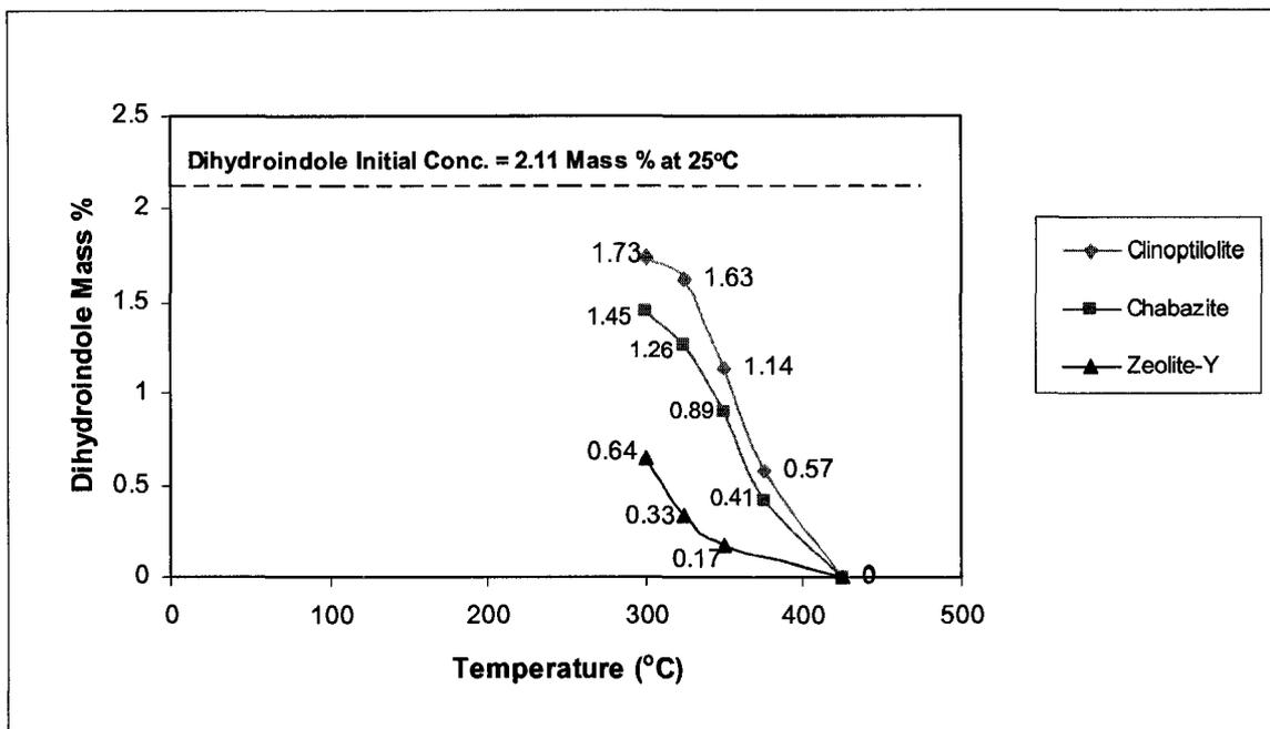
**Figure 4.9 Reduction in Dihydroindole Mass Percent after Reaction**
