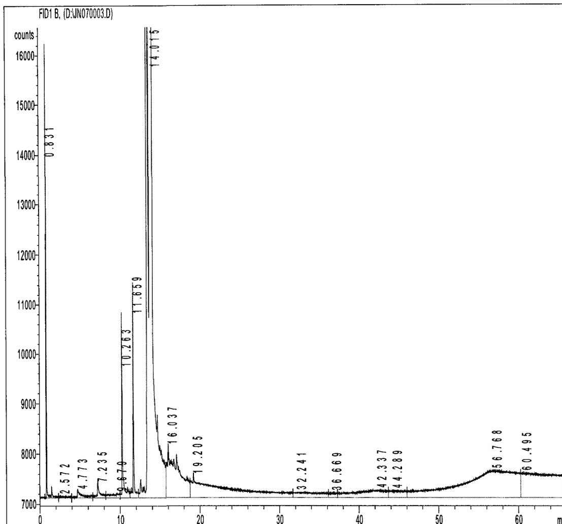
**Figure 4.10 Gas Chromatogram of Dihydroindole in 1-Methylnaphthalene Solution reacted with Clinoptilolite at 425 °C**
