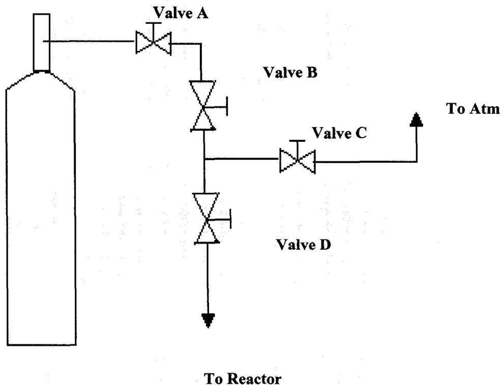
**Figure 3.3 Nitrogen Cylinder Manifold Schematic**
