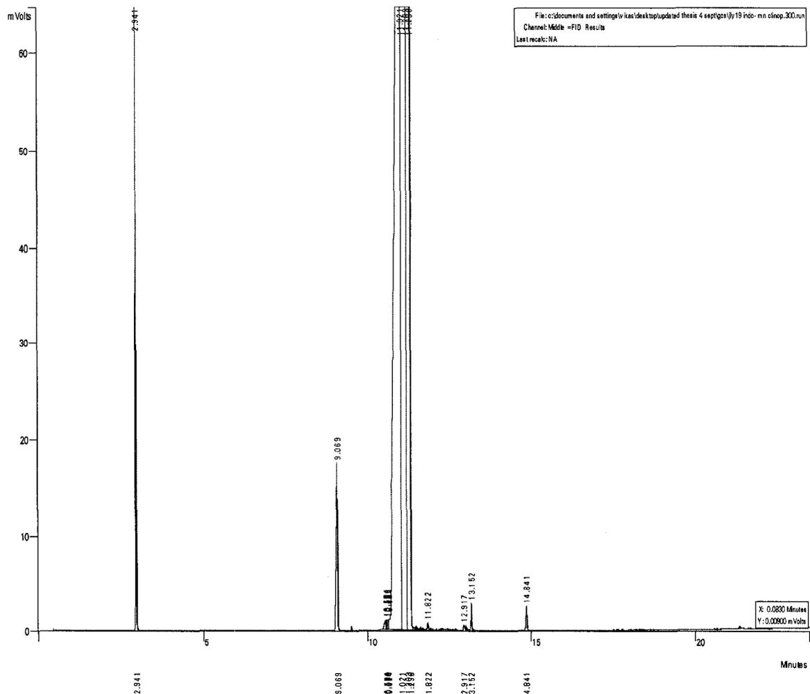
**Figure B.16 Gas Chromatogram of Dihydroindole in 1-Methylphthalene Solution Reacted with Clinoptilolite at 300°C**
