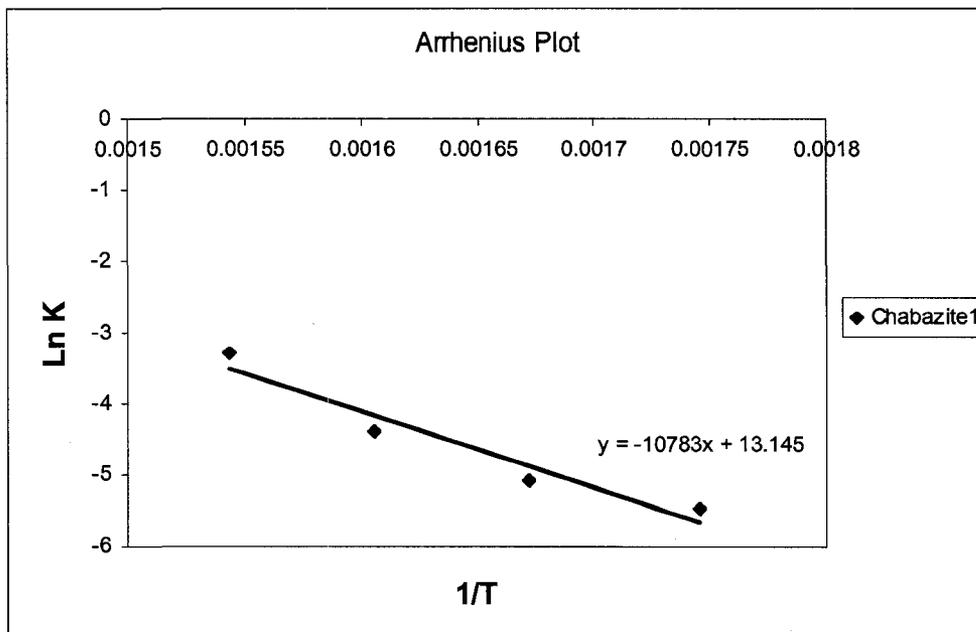
**Figure D.05 Arrhenius plot of ln (K) versus 1/T**
