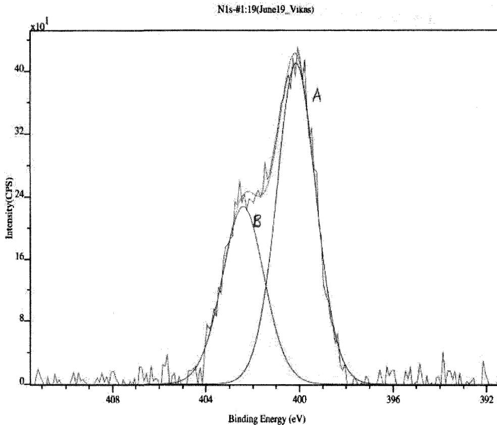
**Figure 4.12 XPS of Dihydroindole Reacted Clinoptilolite**
