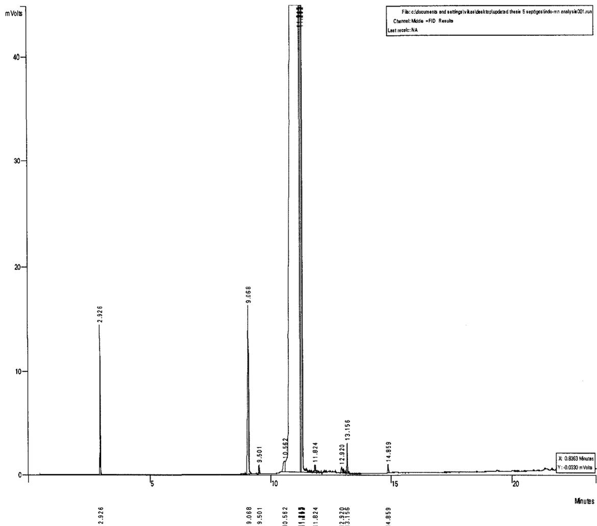
**Figure B.17 Gas Chromatogram of Dihydroindole in 1-Methylnaphthalene Solution Reacted with Clinoptilolite at 325°C**
