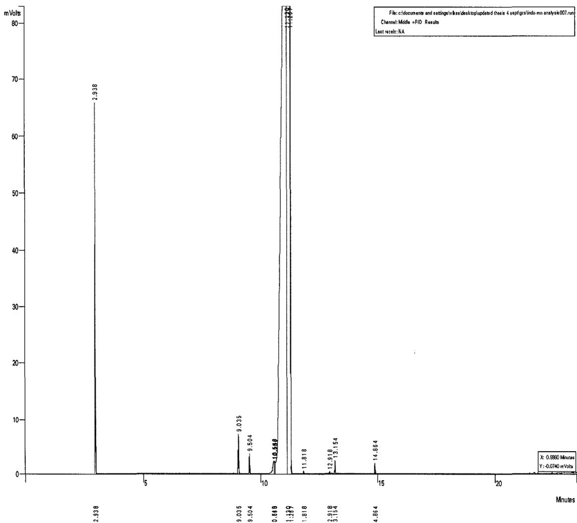
**Figure B.19 Gas Chromatogram of Dihydroindole in 1-Methylnaphthalene Solution Reacted with Clinoptilolite at 375°C**
