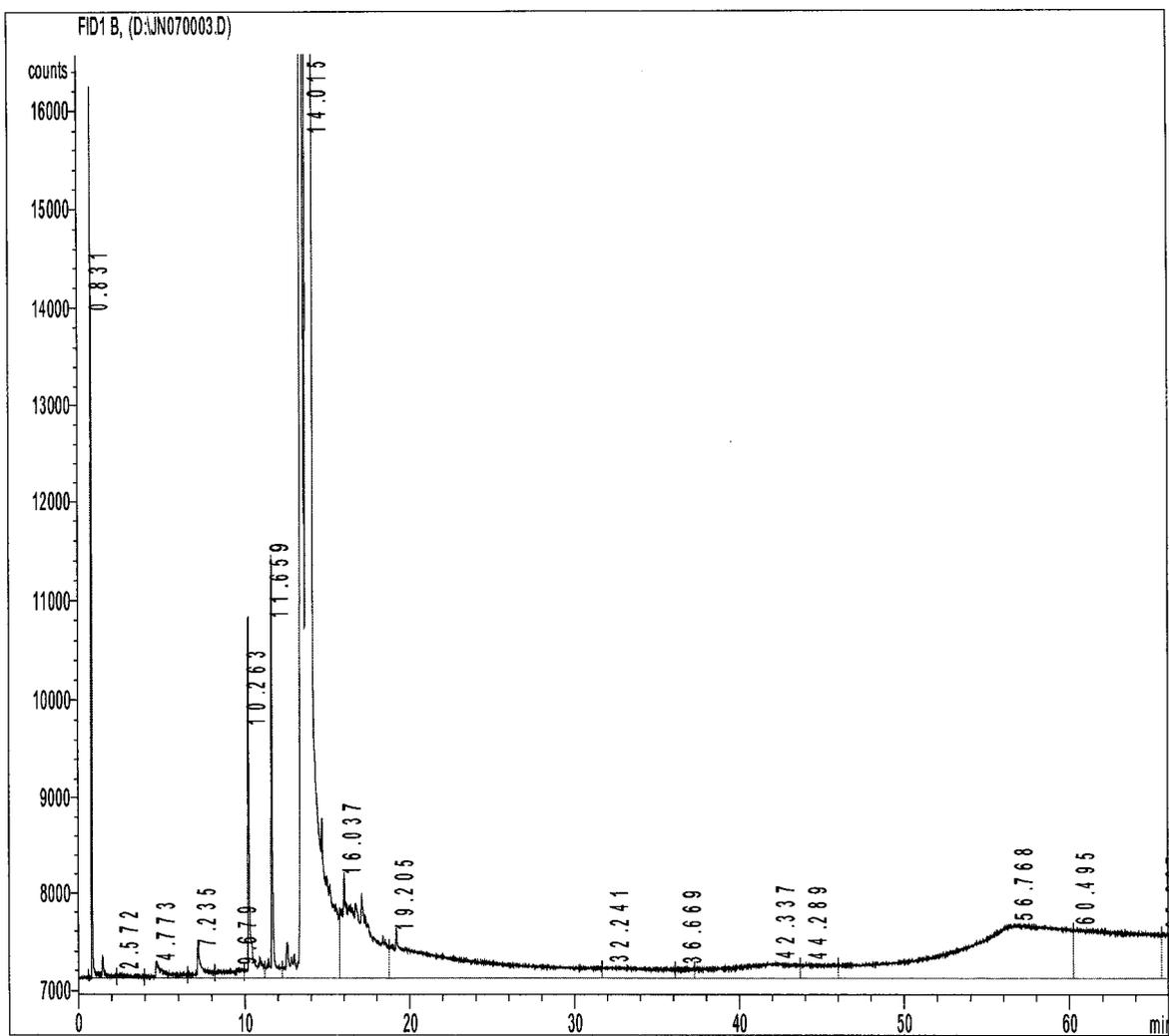
**Figure B.20 Gas Chromatogram of Dihydroindole in 1-Methylnaphthalene Solution Reacted with Clinoptilolite at 425°C**
