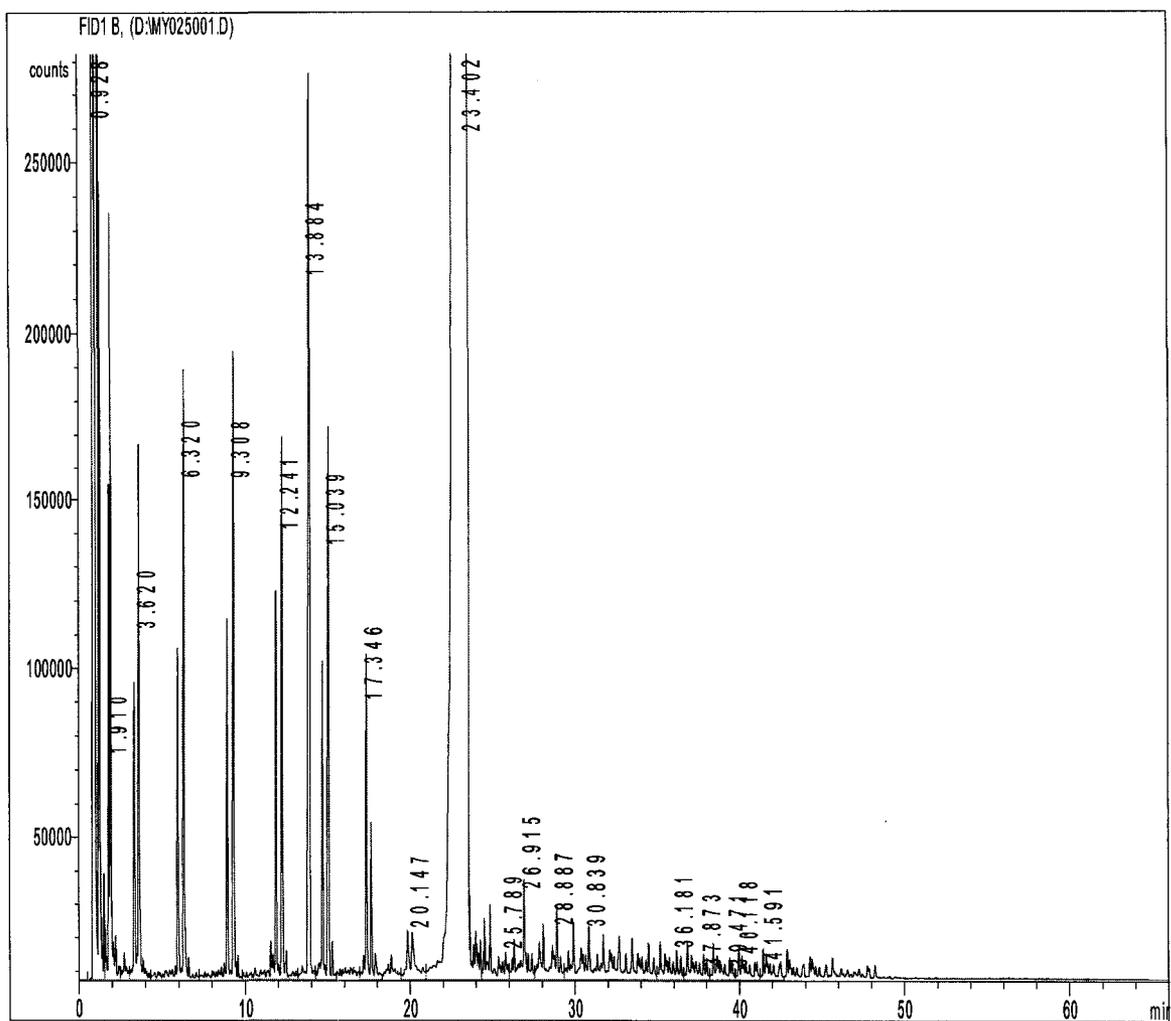
**Figure B.07 Gas Chromatogram of Thermal Cracked n-Hexadecane**
