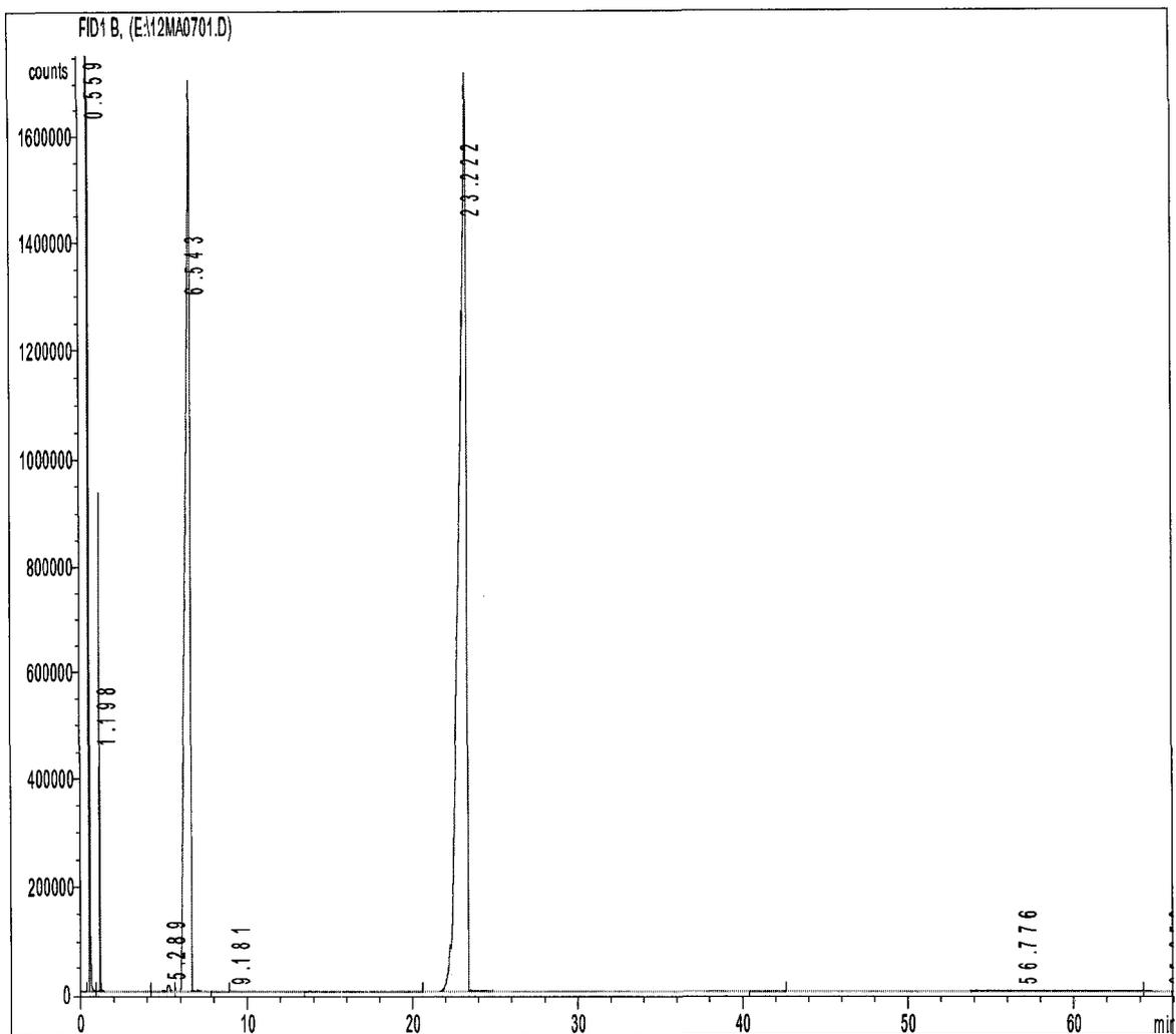
**Figure B.06 Gas Chromatogram of n-Hexadecane with Internal Standard**
