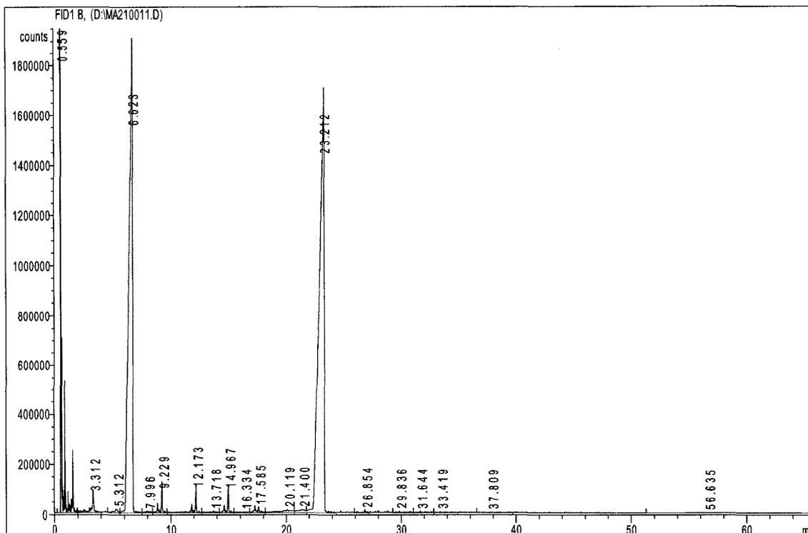
**Figure 4.7 Gas Chromatogram of n-Hexadecane Cracking with Zeolite-Y at 425 °C**
