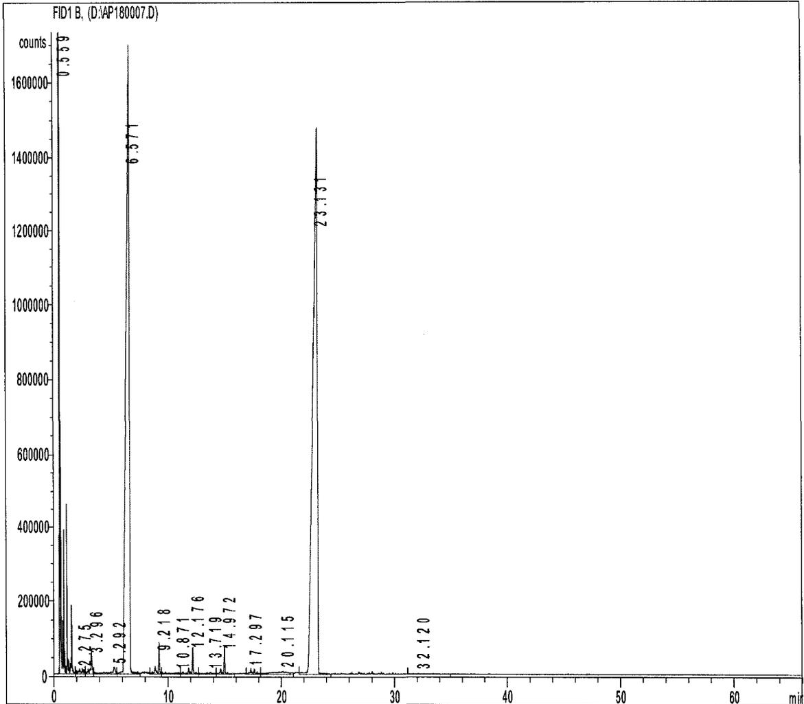
**Figure B.08 Gas Chromatogram of n-Hexadecane Cracking with Clinptilolite at 425°C**
