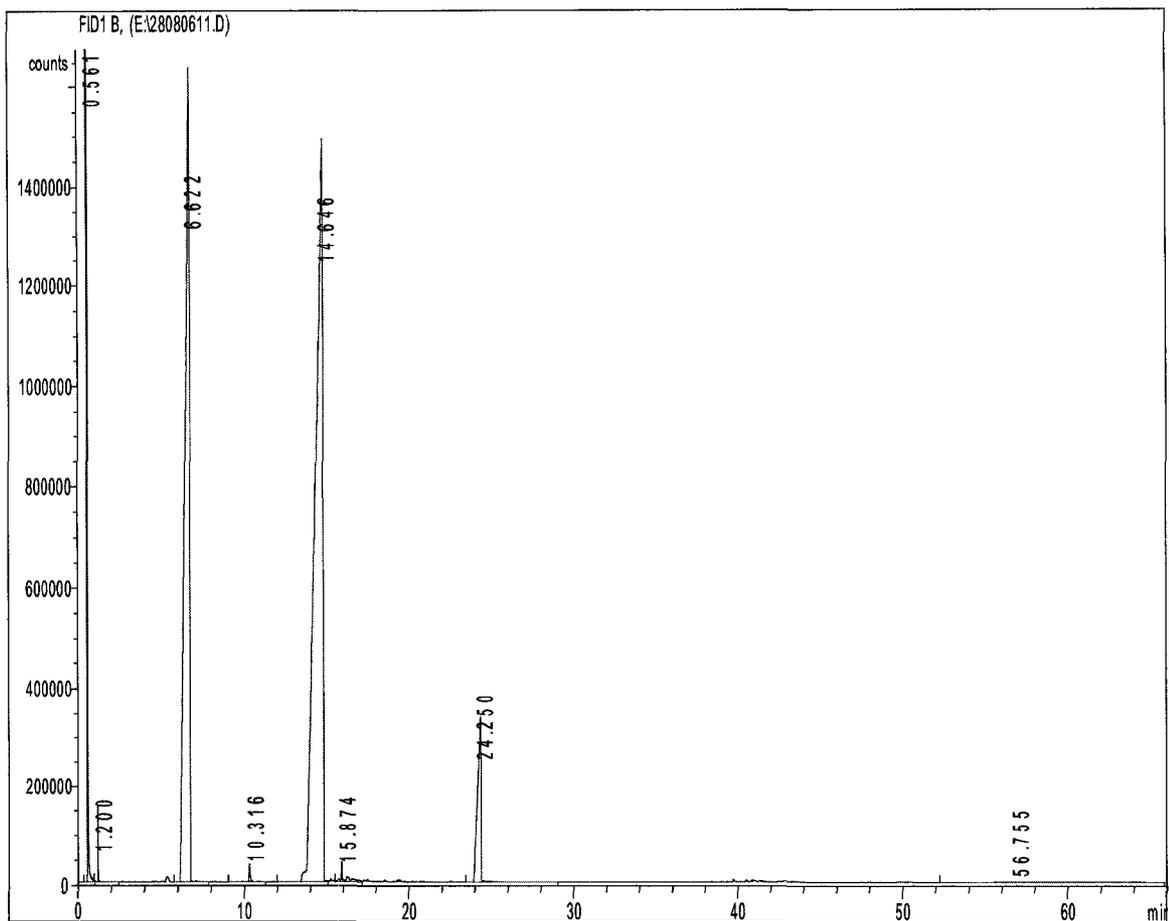
**Figure B.12 Gas Chromatogram of Dibenzothiophene Reacted with Modified Chabazite at 425°C**
