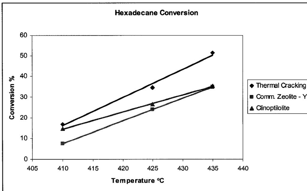
**Figure 4.4 Plot of Temperature versus n-Hexadecane Percent Conversion**
