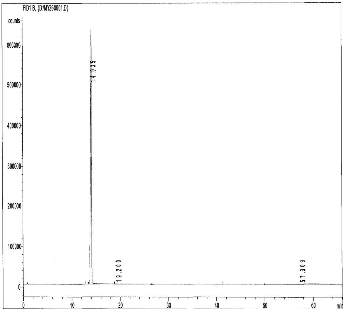
**Figure B.01 Gas chromatogram of 1-Methylnaphthalene**
