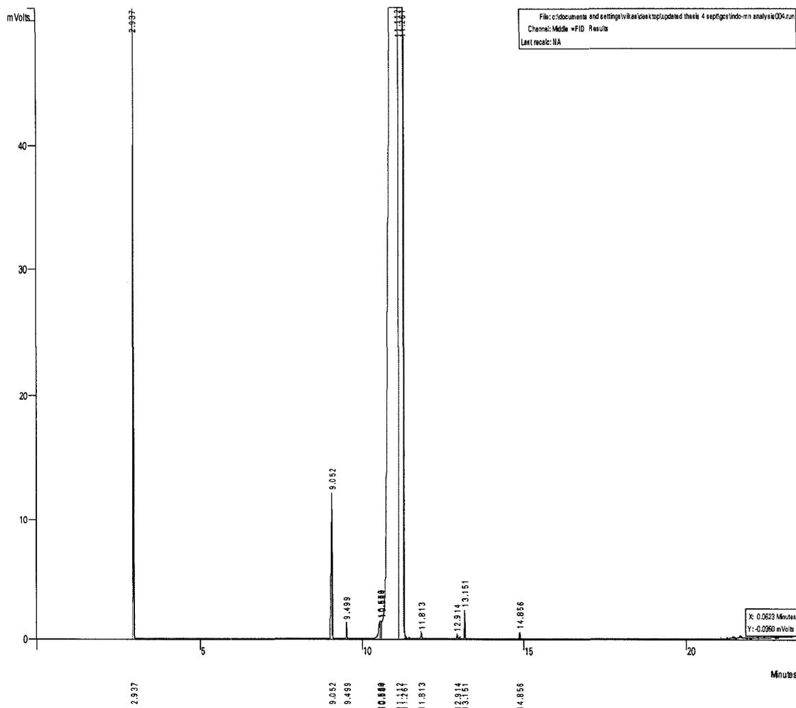
**Figure B.18 Gas Chromatogram of Dihydroindole in 1-Methylnaphthalene Solution Reacted with Clinoptilolite at 350°C**
