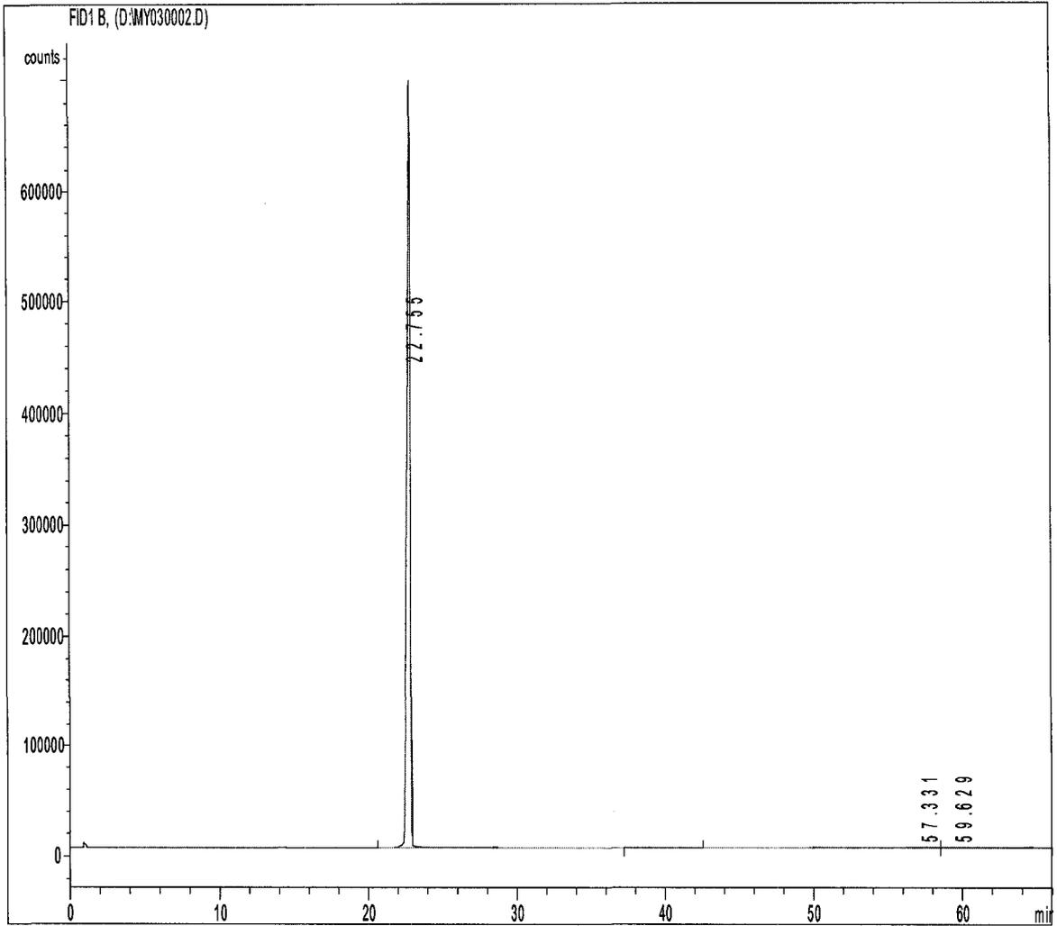
**Figure B.05 GC of Pure n-Hexadecane without Internal Standard**
