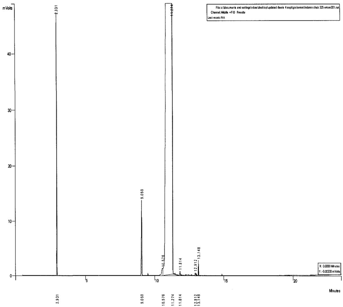
**Figure B.21 Gas Chromatogram of Dihydroindole in 1-Methylnaphthalene Solution Reacted with Chabazite at 325°C (Error Test)**
