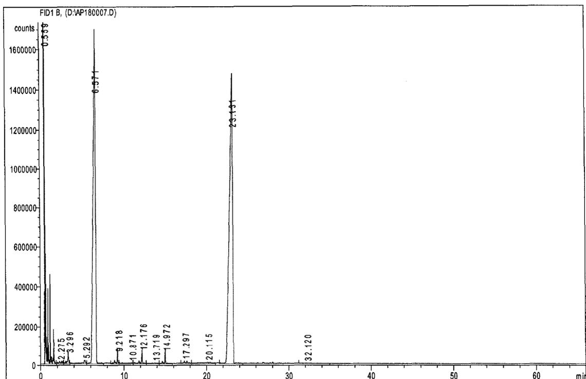
**Figure 4.6 Gas Chromatogram of n-Hexadecane Cracking with Clinptilolite at 425°C**
