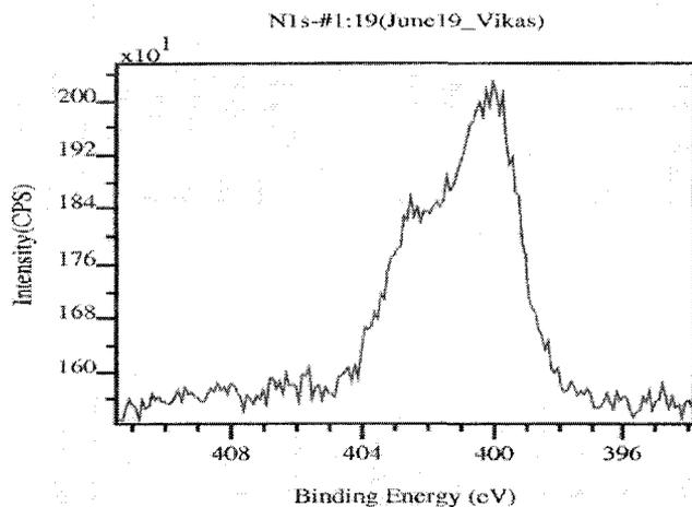
**Figure 4.14 (a) XPS of Dihydroindole reacted Clinoptilolite**
