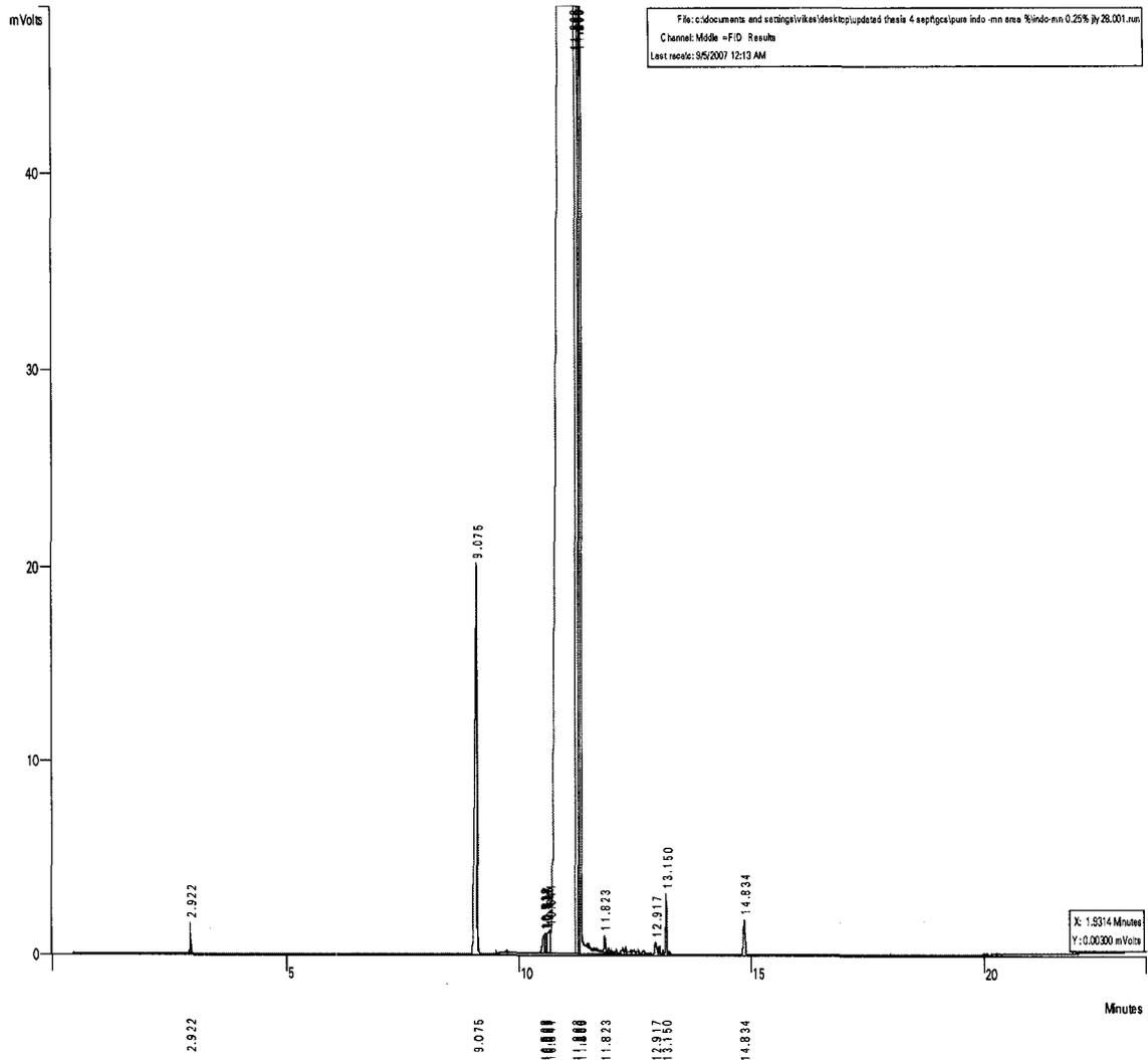
**Figure B.15 Gas Chromatogram of Dihydroindole in 1-Methylnaphthalene Solution**
