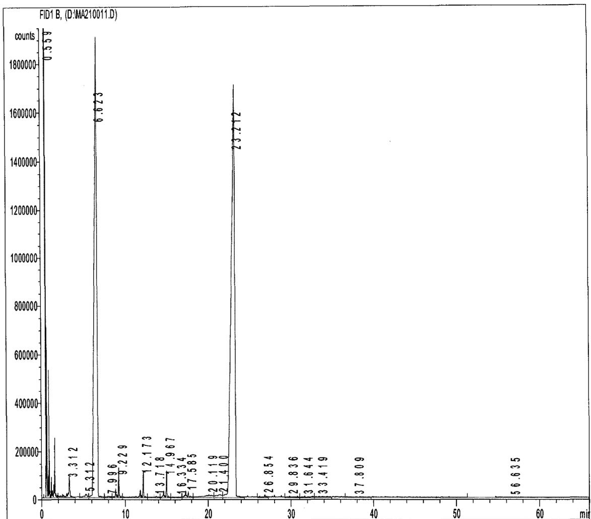
**Figure B.09 Gas Chromatogram of n-Hexadecane Cracking with Zeolite-Y at 425°C**
