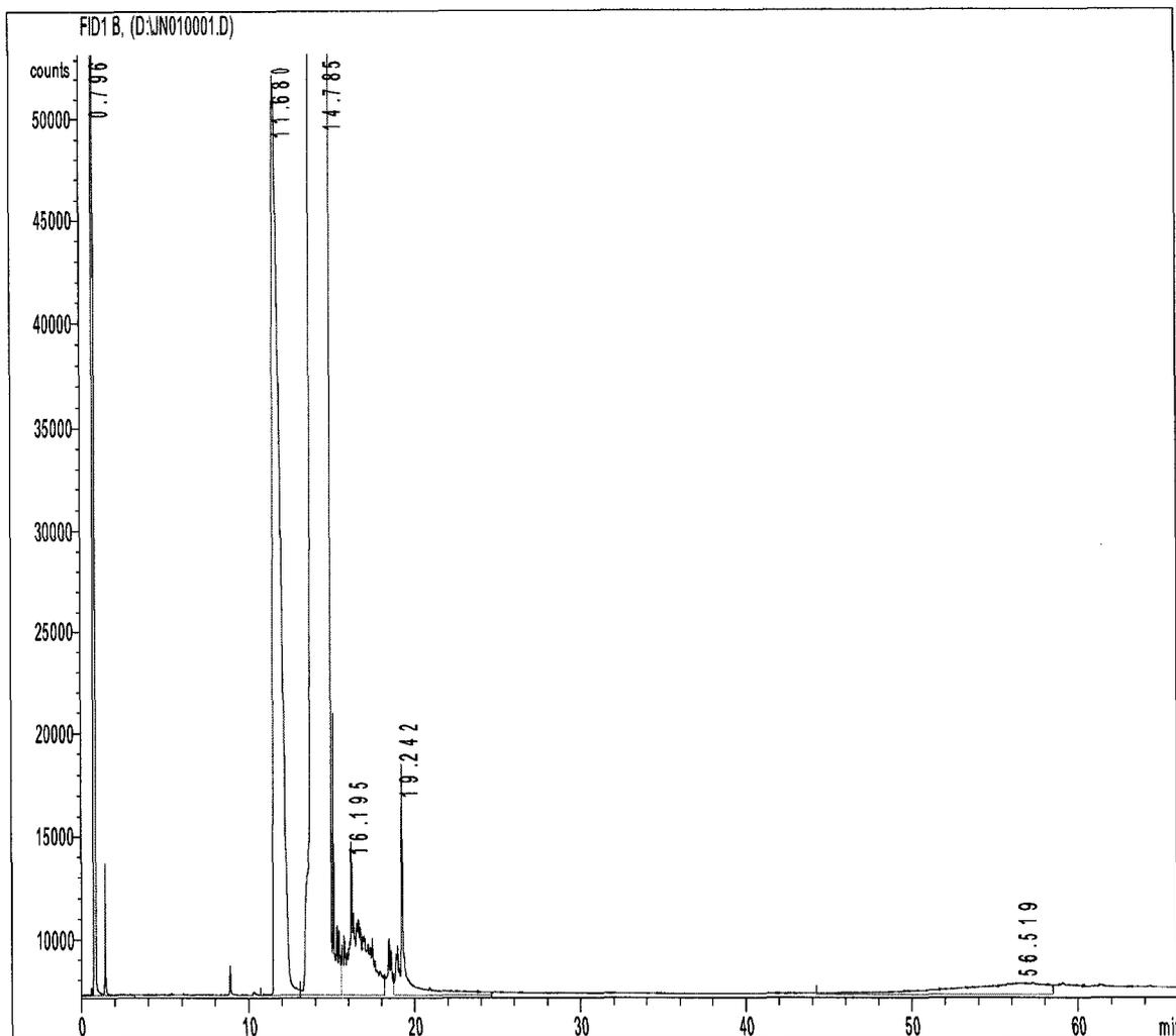
**Figure B.13 Gas Chromatogram of Quinoline in 1-Methylnaphthalene Solution**
