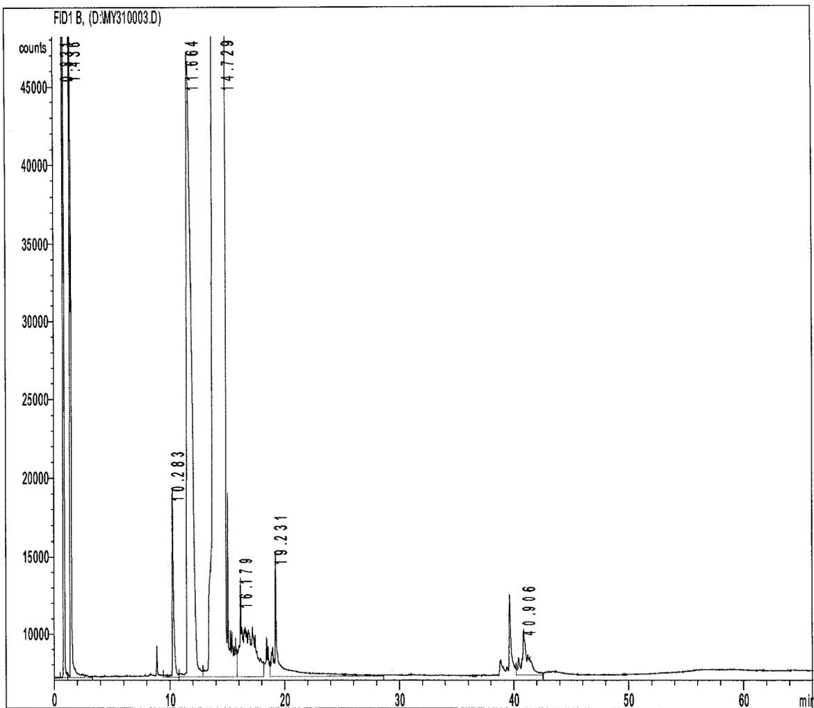
**Figure B.14 Gas Chromatogram of Quinoline in 1-Methylnaphthalene Solution reacted with Clinoptilolite at 425°C**
