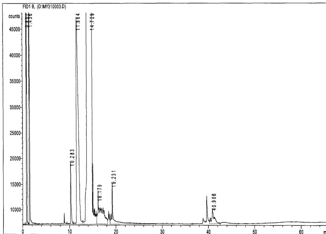
**Figure 4.8 Gas Chromatogram of Quinoline in 1-Methylnaphthalene Solution reacted with Clinoptilolite at 425 °C**
