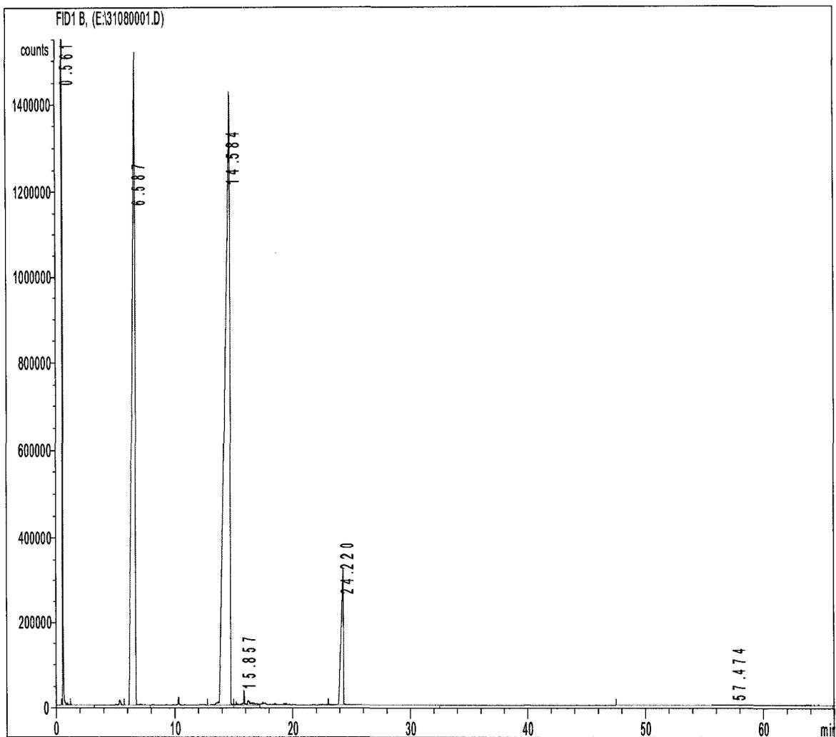
**Figure B.11 Gas Chromatogram of Dibenzothiophene Thermally Reacted at 425°C**
