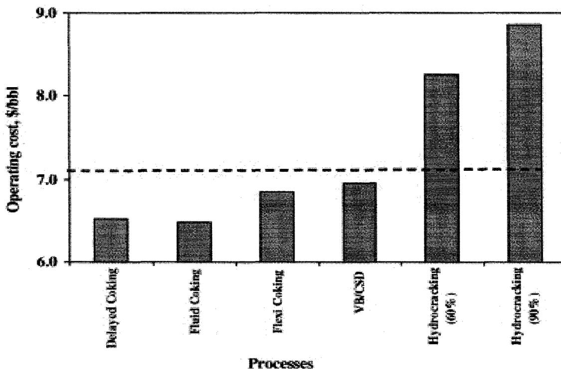
**Figure 2.1: Operating cost for hydrocarbon upgrading processes, Courtesy Rana et.al (2007)**
