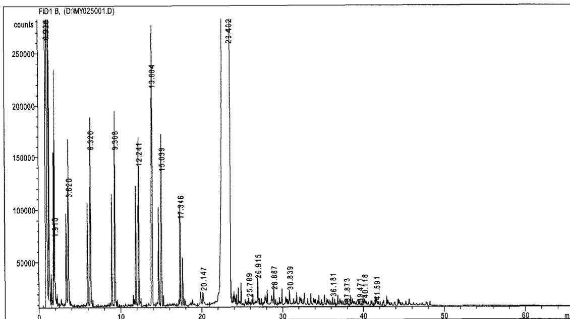
**Figure 4.5 Gas Chromatogram of Thermal Cracked n-Hexadecane**
