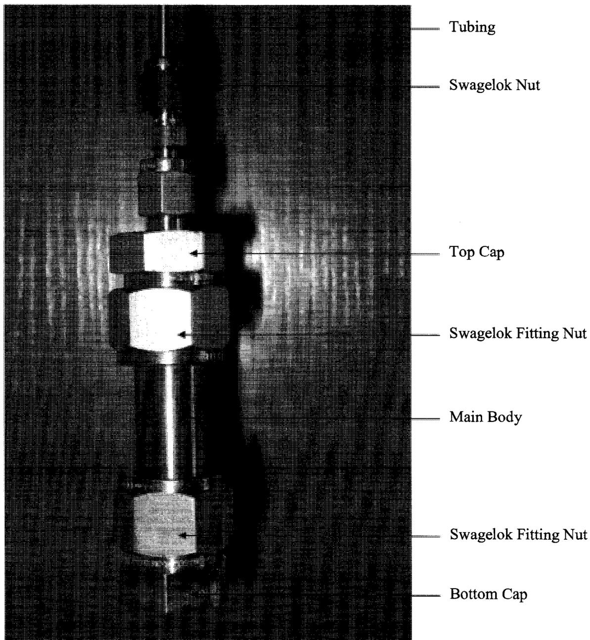
**Figure 3.1 Microbatch Reactor**
