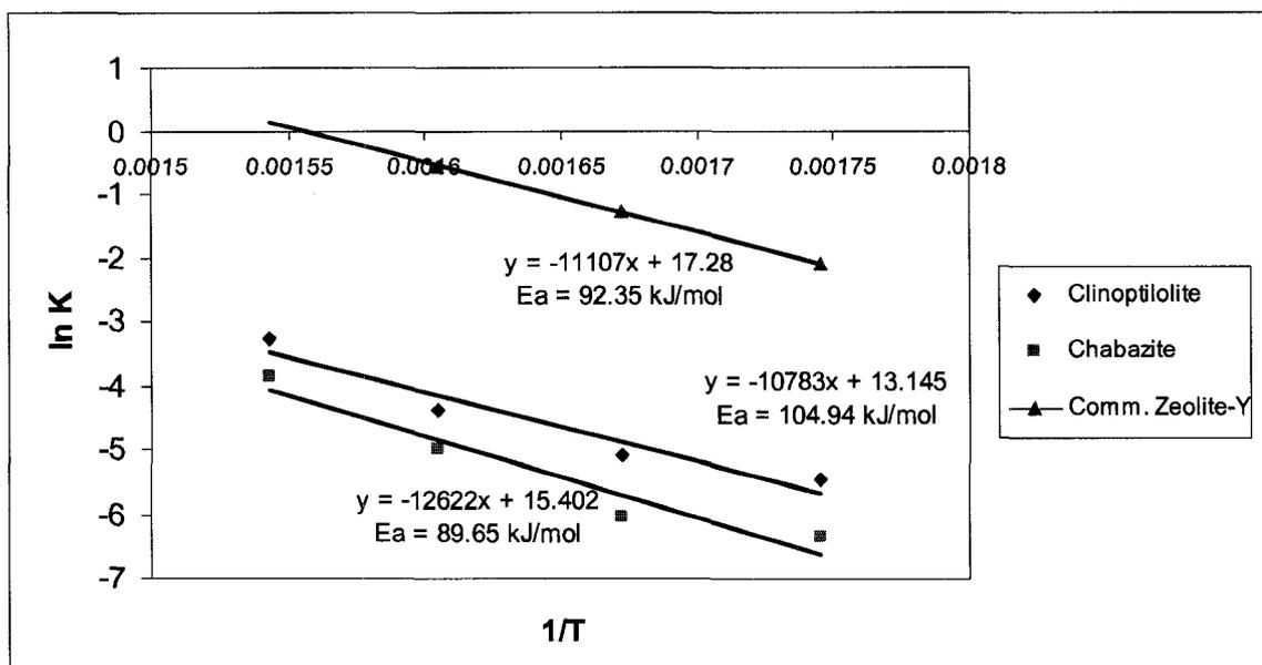
**Figure 4.20 Arrhenius Plot for Determining Catalysts Activation Energy**
