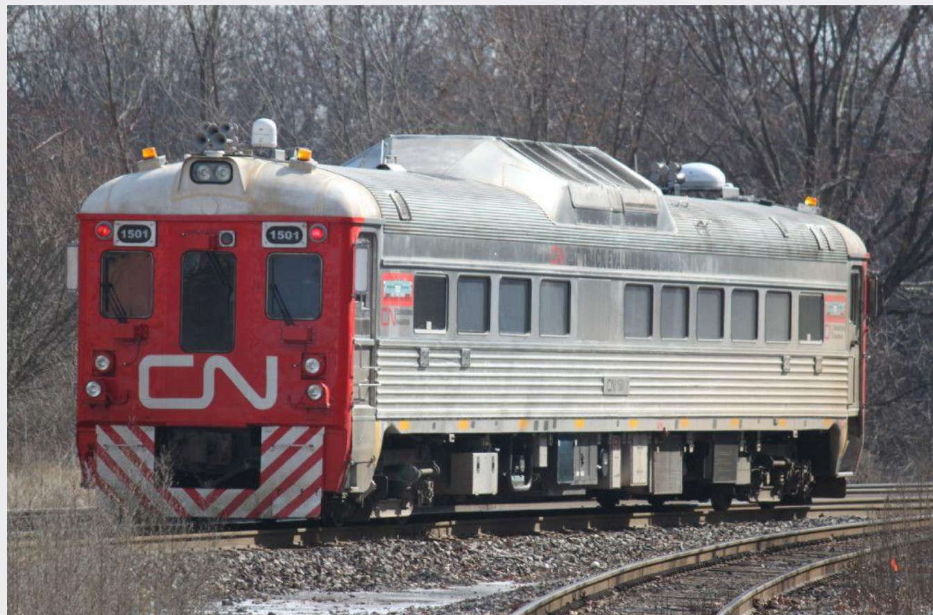
Figure 7. CN's geometry inspection vehicle (BArailssystem, 2014).
